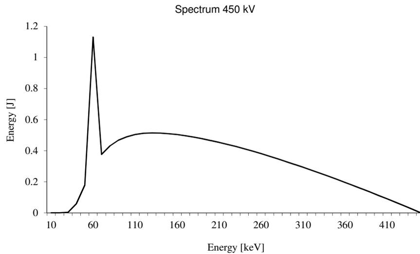
**Figure 7. Spectrum from an 450 kV x-ray tube (tungsten anode).**
