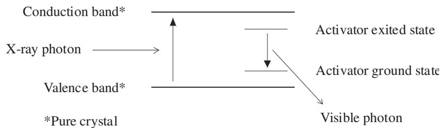
Figure 8. Energy band structure.
