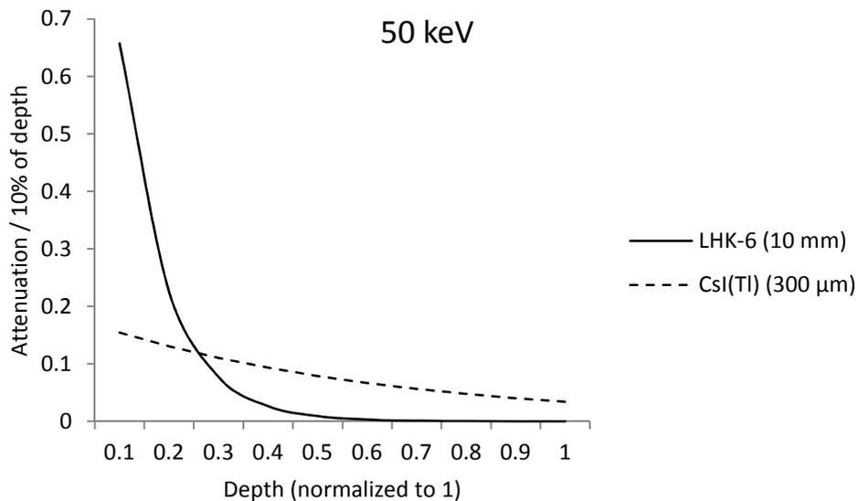
**Figure 11. Attenuation depth 50 keV.**
