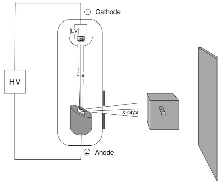
Figure 4. Principles of x-ray radiography.
