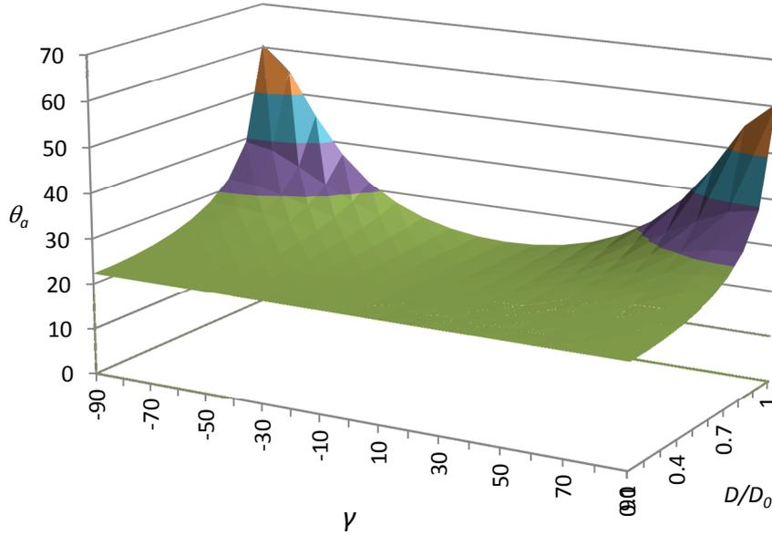
**Figure 17. Acceptance angle vs. radial position.**
