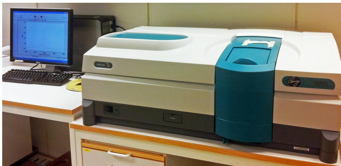
**Figure 5.1: Varian Cary 5000 spectrophotometer together with the computer and software set for calculation of transmission, absorption and extinction.**
