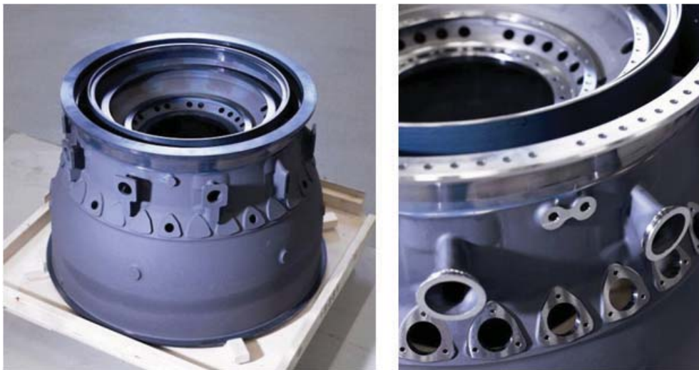
Figure 1: To the left is shown a semi-finished compressor rear frame—one of the parts processed in the multitask cell. To the right is shown a close-up of the final product.
