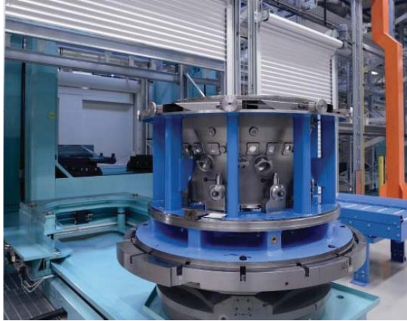
Figure 6: A part mounted into a fixture at a set-up station in the multitask cell.
