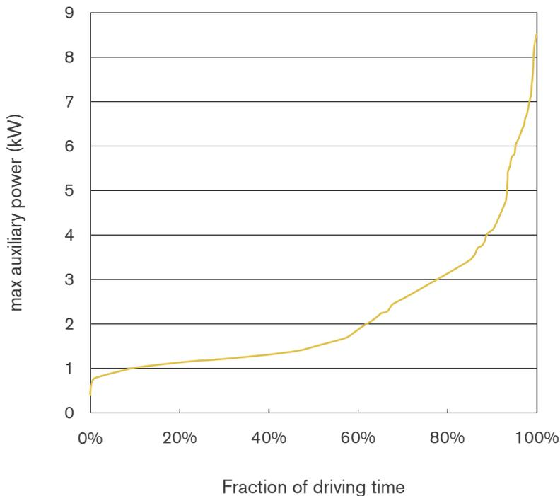
**Figure 5.5** Measured auxiliary power use in six Peugeot Ions during real driving. The driving occurred at all seasons of the year in Belgium.<sup>4</sup>
