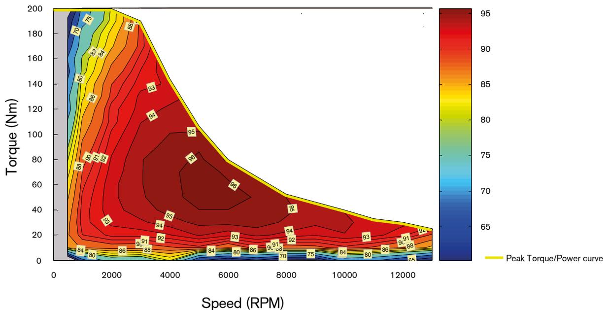
**Figure 5.4** 2010 Toyota Prius motor efficiency contours.<sup>3</sup>
