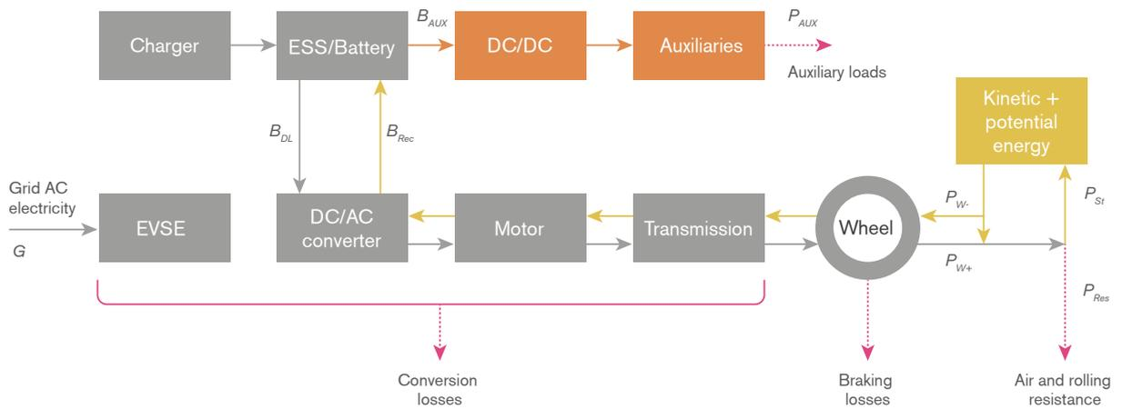
**Figure 5.1** The conversion chain in electric vehicles. Energy is transferred from grid electricity ( $G$ ), via the battery ( $B_{DL}$  and  $B_{Aux}$ ), to energy at the wheels ( $P_{W+}$ ) and auxiliary equipment ( $P_{Aux}$ ). Part of stored potential and kinetic energy is recovered through the wheels ( $P_{W-}$ ) to the battery ( $B_{Rec}$ ).
