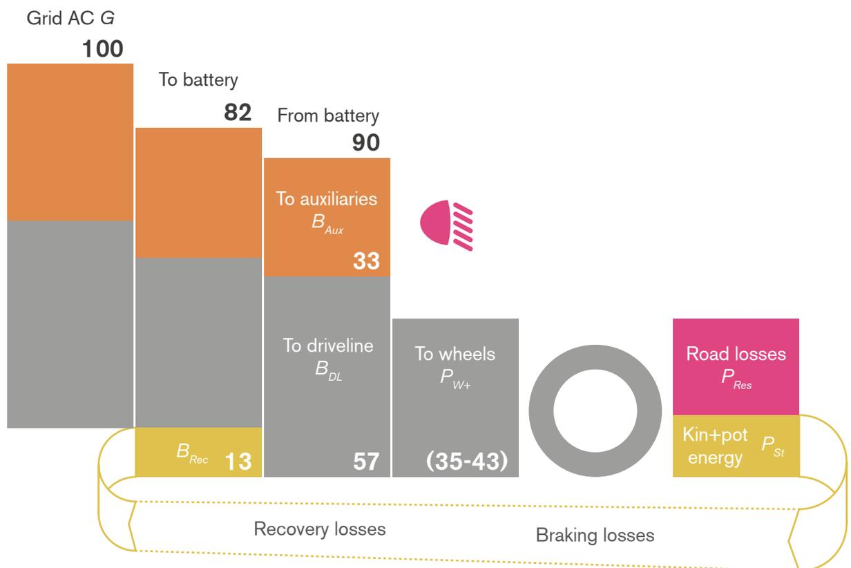
**Figure 5.6** Energy fluxes for a Peugeot Ion electric vehicle during real driving conditions in Belgium. Figures in parenthesis are estimates based on dynamometer measurement. The figures are given in percentages of the energy delivered from the grid = 100. Orange denotes the share required by auxiliaries.<sup>7</sup>
