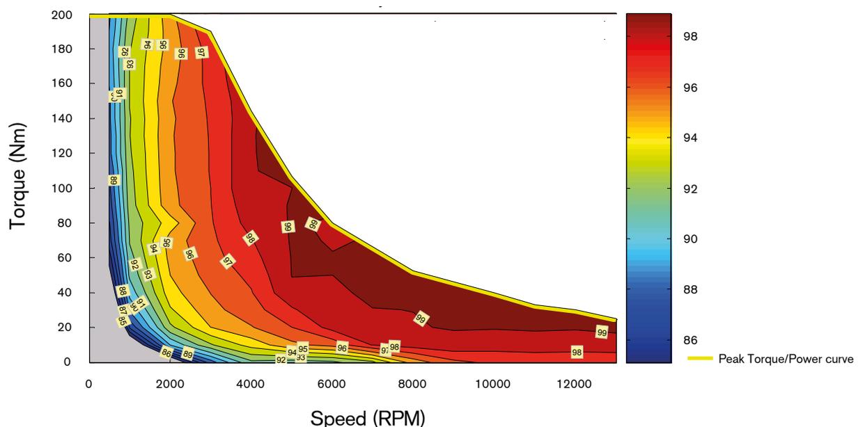
**Figure 5.3** 2010 Toyota Prius inverter (DC/AC converter) efficiency contours.<sup>3</sup>
