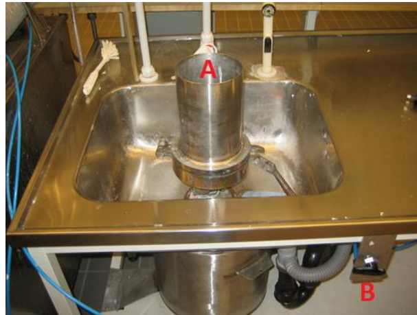
Figure 7 A standard sheet former. A) the container in which the solution was poured in to B) regulation of vacuum
