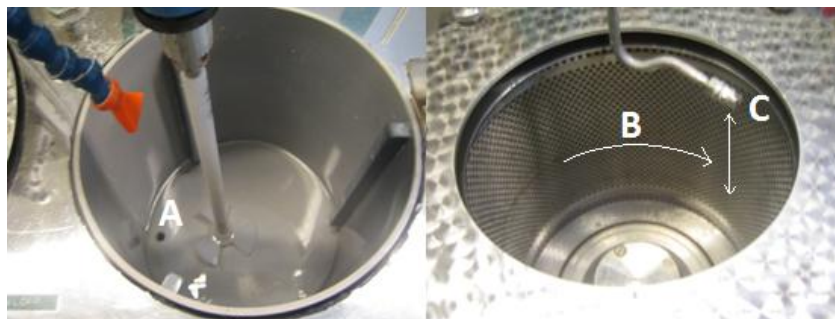
Figure 29 left picture: the drum in which the mixture was poured and pumped to the nozzle. Right picture: Inside of drum without wire. B: rotational direction of drum. C: Vertical direction of the nozzle.
