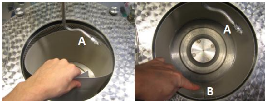
Figure 28 the support wire was placed inside the drum of the Format. A: The nozzle that sprayed the mixture on the monodur fabric. B: Edges of the support wire intertwined which enabled the monodur fabric to remain fixed.
