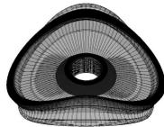
**Figure 6:** Axial mode of the wheel with two nodal diameters and zero nodal circles, which has an eigenfrequency of 430 Hz.
