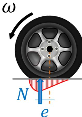
Figure 13. The origin of rolling resistance moment
