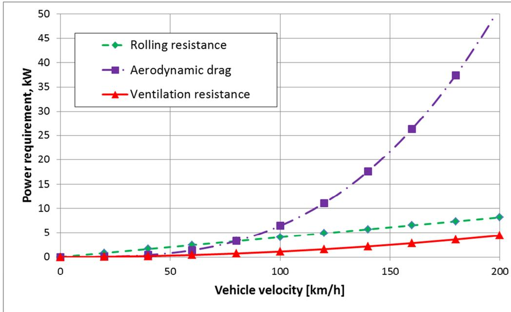
Figure 23. Power requirement to overcome different resistances
