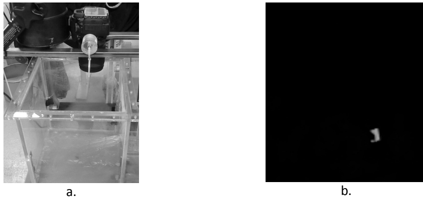
Figure 1: (a) The experimental unit used. The ultraviolet light lamp is visible at the upper left corner. The camera used for video recordings is located next to the UV-lamp. (b) Colored tracer particle (black-and white photo here) viewed from above glows brightly which enables detection of its position.
