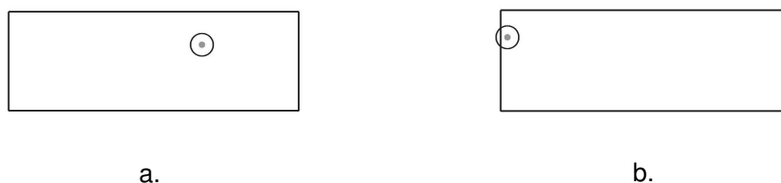
Figure 2: Location of the tracer particle before immersion (dot) and expected traveled distance after immersion time (circle). a): valid data point for the analysis. b): discarded data point in the analysis
