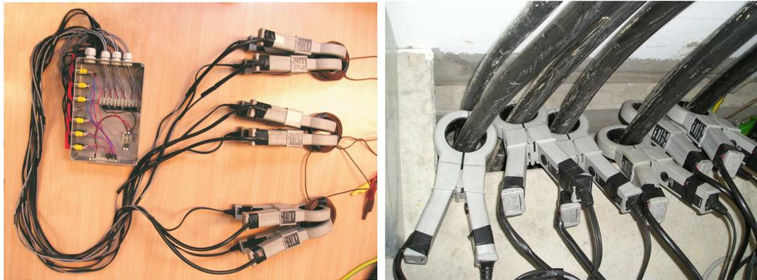
Figure 3.6. Current clamps with power supply unit(left), in real measurement (right)
