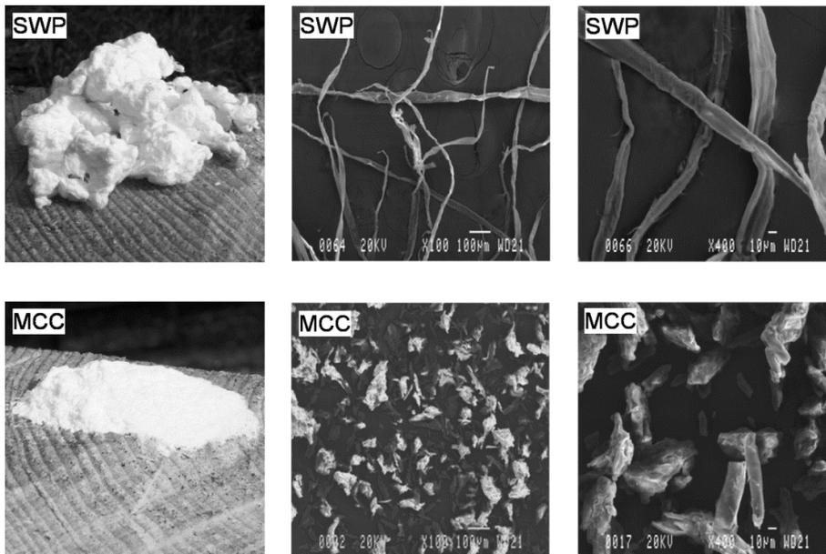
Figure 2 Ordinary photographs and SEM micrographs of softwood kraft pulp (SWP) and microcrystalline cellulose (MCC).
