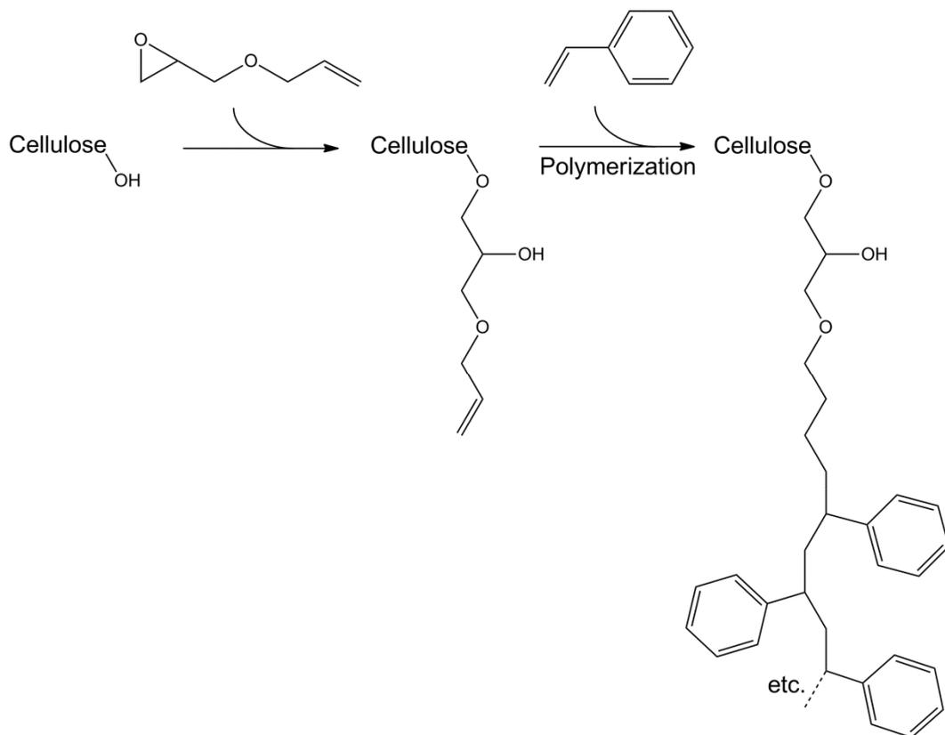
Figure 6 Schematic figure of the reaction of cellulose with allyl glycidyl ether, followed by grafting of styrene.
