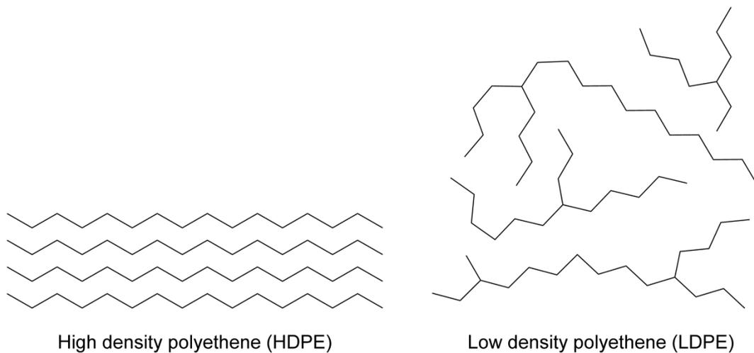
Figure 5 Schematically drawn structures of linear and more crystalline PE, and branched and less crystalline PE.
