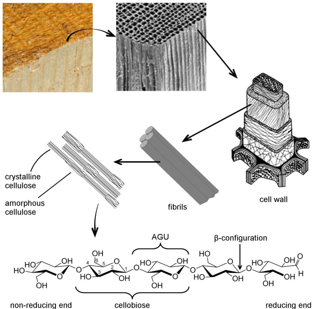
Figure 3 A schematic figure of the wood structure and the chemical structure of cellulose.
