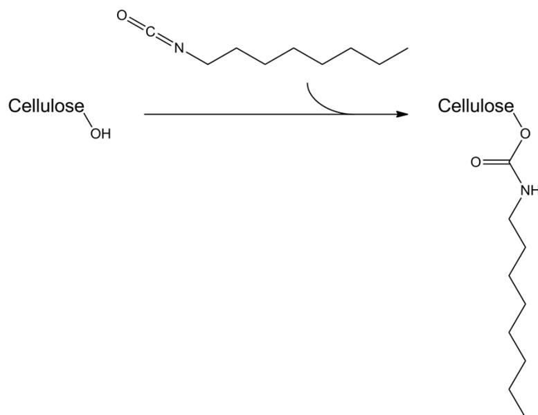
Figure 7 Schematic figure of the compatibilization of cellulose with octyl isocyanate.
