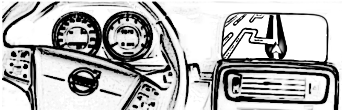
Figure 2.2: This is an example of what is usually associated with an in-vehicle infotainment system. There is normally a touch screen, located in the dashboard between the driver and passenger, allowing user interaction. There may also be a screen behind the wheel as well as a heads-up display shown on the windscreen, to display information to the driver.
