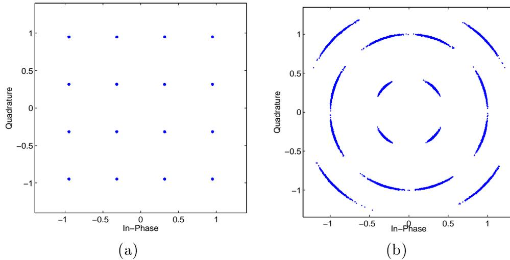
Figure 3.3: 16-QAM constellation at SNR per bit of 40 dB, when (a) no phase noise is present, (b) affected by a Gaussian distributed phase error of variance  $\sigma_p^2 = 1 \times 10^{-2}$  rad<sup>2</sup>.
