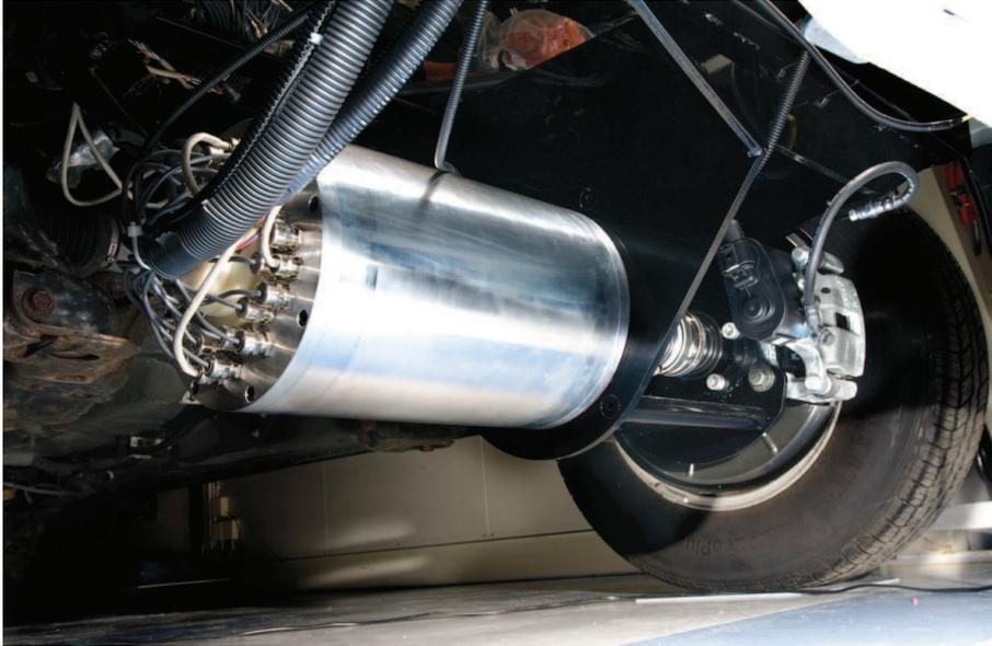
Figure 4.19: Motor installation inside the vehicle.
