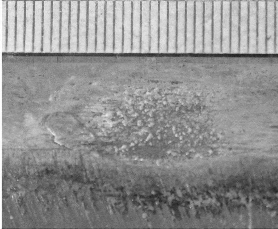
**Figure 8 Squat on the surface of a rail (Scale is in millimeters).**
