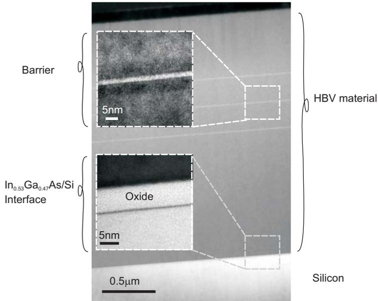
Fig. 3.5: Transmission electron microscopy image of the HBV material structure transferred on silicon substrate with insert showing the magnified barrier and bonding interface. The thickness of the amorphous oxide is approximately 5 nm.
