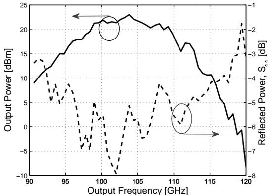
Fig. 4.6: Output (solid line) and reflected power (dashed line) measured at 29 dBm of  $P_{IN,AVA}$  for the silicon integrated case.  $S_{11}$  was better than -6 dBm at the center frequency.
