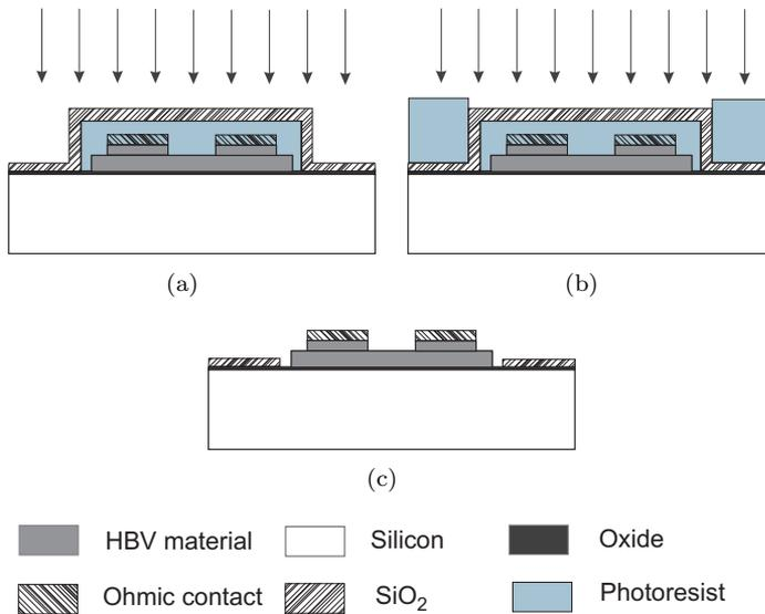
Fig. 3.9: Substrate passivation steps.
