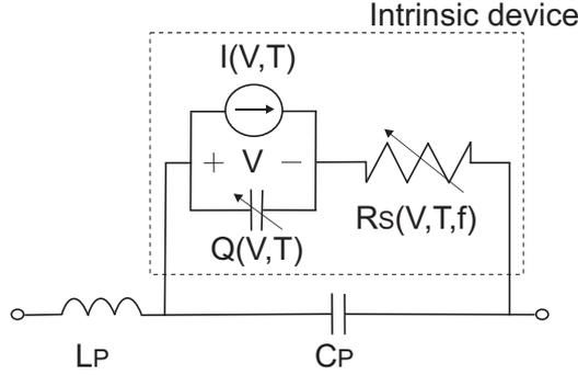
Fig. 2.5: Quasi-static equivalent circuit model of HBV.
