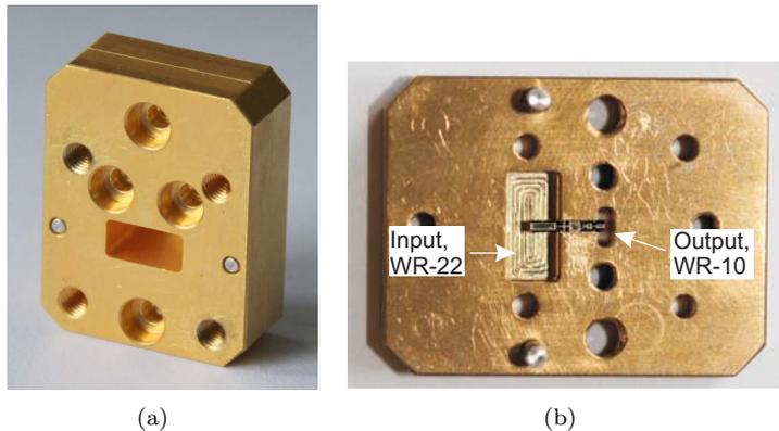
Fig. 4.3: (a) Mounting block for the 100 GHz frequency multiplier; (b) assembled circuit chip in the waveguide channel.
