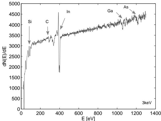
Fig. 3.7: Auger electron spectroscopy data revealing presence of InGaAs on Si substrate.
