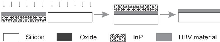
Fig. 3.2: Process flow of LT plasma activated bonding. From *left* surface preparation,  $\text{O}_2$  plasma treatment, (*middle*) bringing the wafers into the contact and bonding at RT. (*right*) After the InP substrate chemical wet etching.
