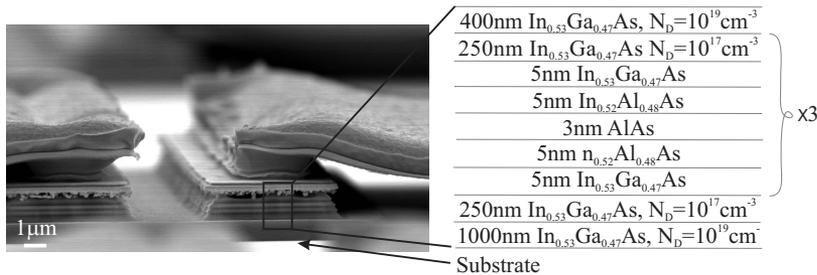
Fig. 3.1: SEM image of an RF diode with depicted material layers on the silicon substrate.
