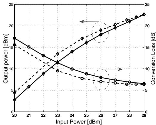
Fig. 4.8: Available output power and a conversion loss as a function of the input power measured at 103 GHz and 107 GHz for devices on Si (solid line) and InP (dashed line), respectively.
