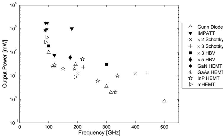
Fig. 1.1: Conventional high frequency power sources: Gunn diodes [12, 13], IMPATT diodes [14, 15], Schottky diodes [16–18], HBVs [19–21], GaN HEMTs [22–24], GaAs HEMT [25], mHEMT [26] and InP HEMT [27–32] power amplifiers.
