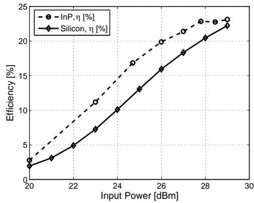
Fig. 4.9: Data for the maximum conversion efficiency at 103 GHz and 107 GHz, for Si and InP, respectively.
