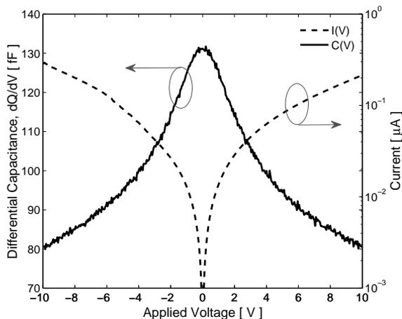
Fig. 4.2: C-V and dark I-V characteristics for a 4 mesas, 12 barriers,  $700\ \mu\text{m}^2$  HBV diode measured at RT.
