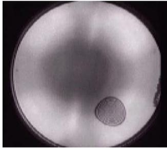
Fig. 3.3: Infrared inspection image of the transferred InGaAs/ InAlAs/ AlAs on silicon. The InP wafer size is 3". The dark area indicates an unbonded region (a void).
