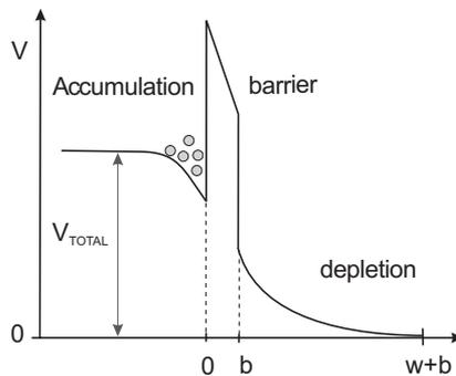
**Fig. 2.4:** Conduction band of HBV under applied bias.  $V_{TOTAL}$  is the applied voltage,  $b$  is the barrier thickness and  $w$  is the depletion layer width.
