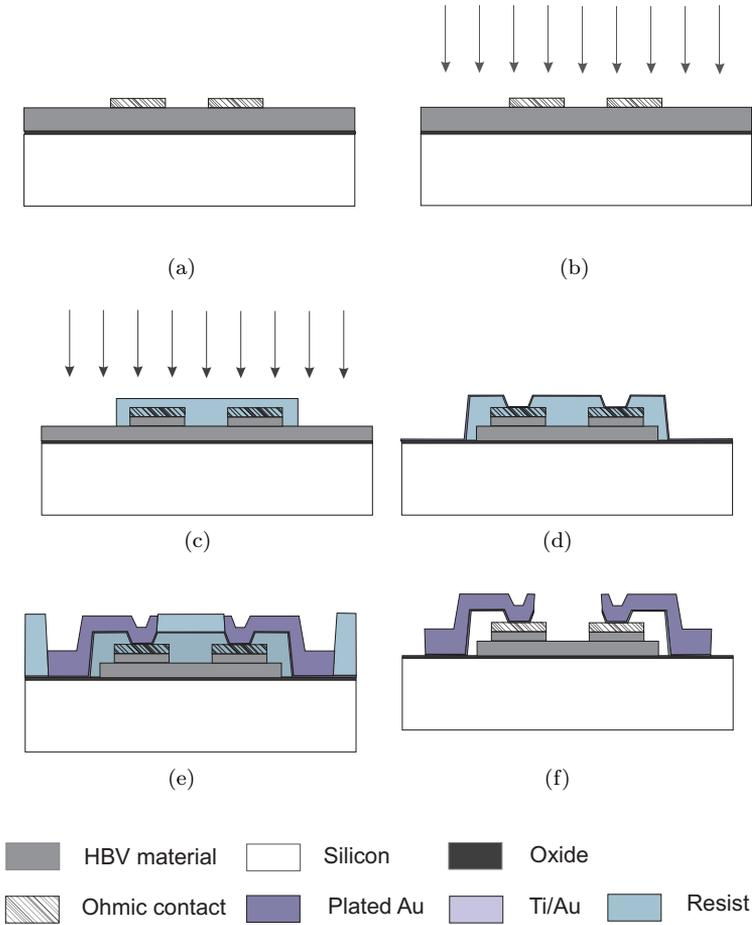
Fig. 3.8: Integrated HBV-based frequency multipliers process steps.
