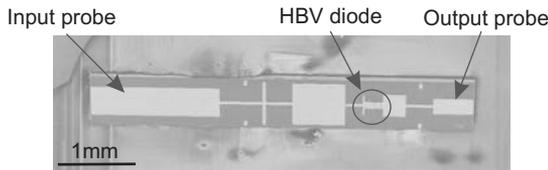
Fig. 4.1: SEM image of an integrated HBV frequency tripler on silicon substrate. The chip size is  $4.7\text{mm} \times 0.8\text{mm} \times 0.08\text{mm}$  (length  $\times$  width  $\times$  thickness). The diode consists of 4 mesas connected in a series (12 barriers). The contact area is  $7 \times 100\ \mu\text{m}^2$ .
