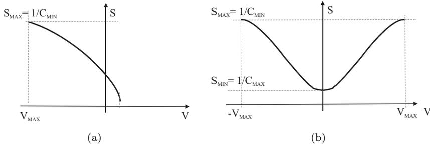
Fig. 2.1: (a) asymmetric and (b) symmetric differential elastance characteristics of varactor devices.
