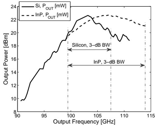
Fig. 4.7: 3-dB bandwidth at peak output power for circuit on Si (solid line) and InP (dashed line). 3-dB bandwidth is 9 % and 15 % for circuit on Si and InP, respectively.
