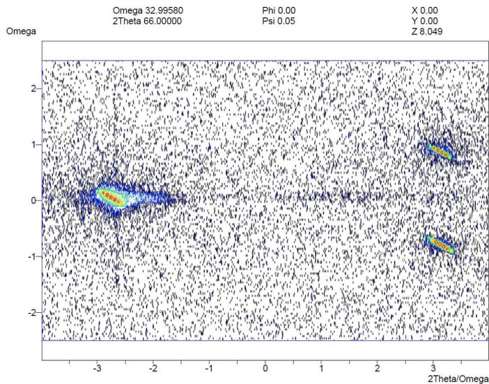
Fig. 3.6: 2D X-ray diffraction scan showing InGaAs ( $2\theta=63^\circ$ ,  $\omega=31.7^\circ$ ) and two peaks related to SOI carrier wafer ( $2\theta=69^\circ$  and  $\omega$  of  $31.5^\circ$  and  $34.5^\circ$  for substrate and top layer, respectively).
