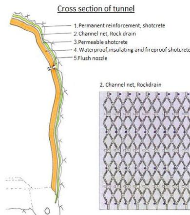
Figure 18: Illustration of the Rockdrain drainage system (Melander, 2011)
