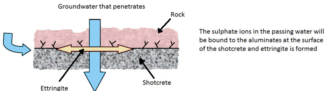
Figure 9: Illustration of ettringite formation, modified after Lagerblad (2007).
