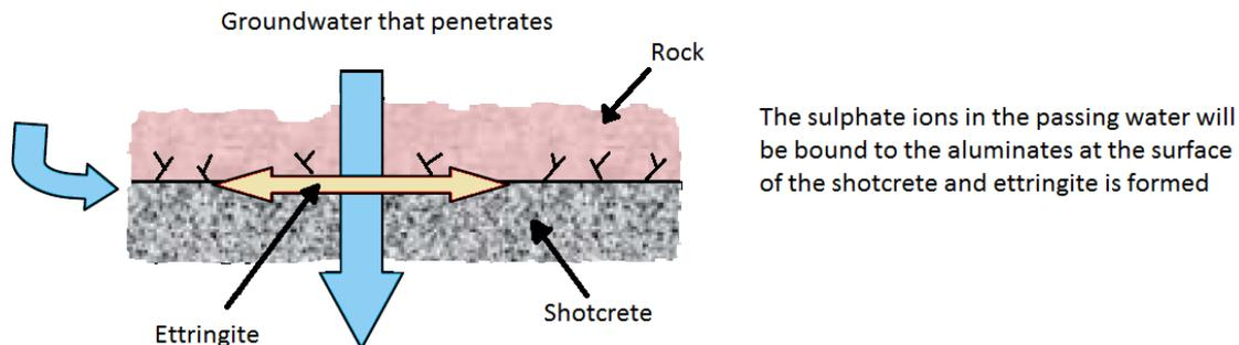
Figure 9: Illustration of ettringite formation, modified after Lagerblad (2007).
