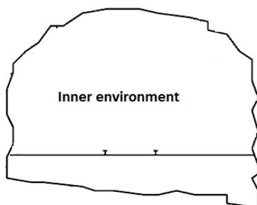
Figure 13: Exposure and corrosivity classes depend on the environment the construction material is exposed to. The rock that surrounds the tunnel is described as the outer environment and the traffic environment is described as the inner environment. Modified after Trafikverket (2011).
