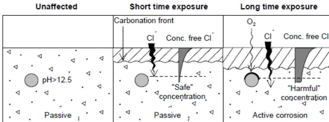
Figure 10: Schematic sketch for chloride induced corrosion (Nordström, 2005).
