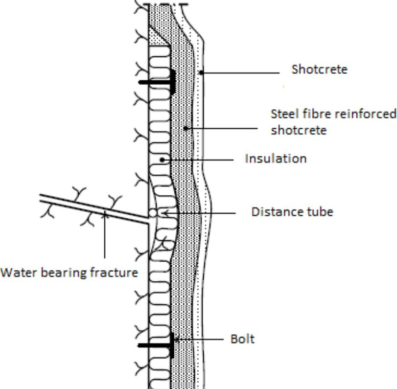
Figure 12: Conventional drainage system (Ansell et al., 2007).
