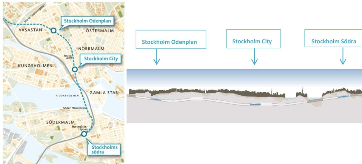
Figure 25: The blue dotted line illustrates the tunnel stretch. The figure to the right shows the profile of the tunnel (Trafikverket, 2012).
