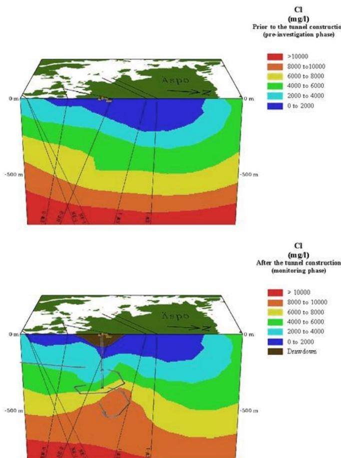
Figure 6: The top figure illustrates the salinity in bedrock groundwater prior the tunnel construction and the figure below shows the upconing effect due to the tunnel construction (Laaksoharju et al., 1999).
