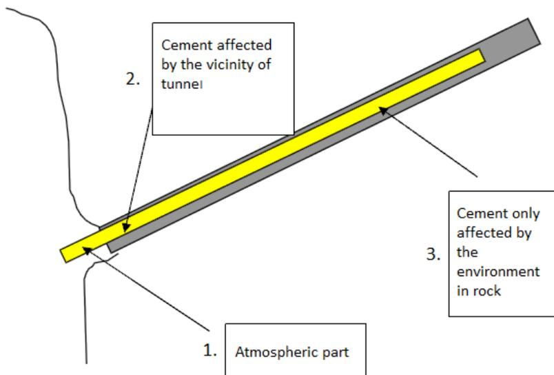
Figure 8: Cement embedded bolt in rock. Modified after Sandberg (2007)
