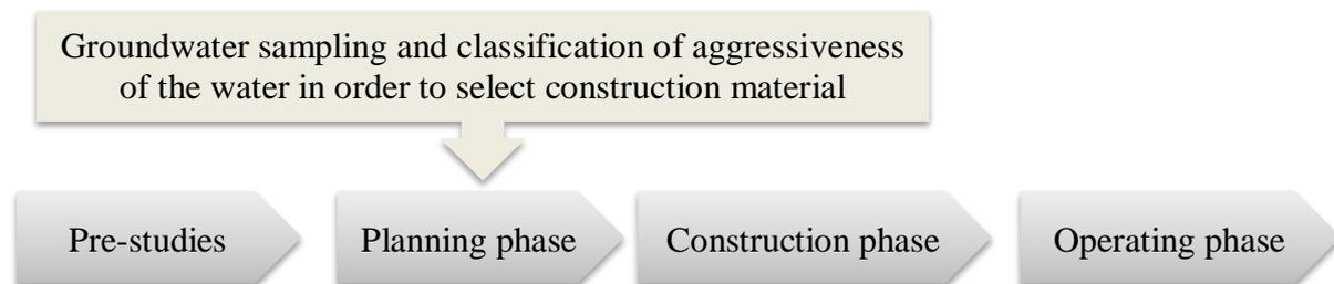
Figure 14: Phases of a tunnel project where it can be seen when the procedures for material selection is performed
