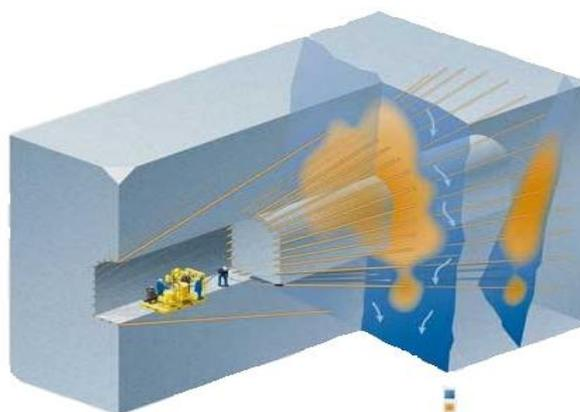
Figure 11: Grouting procedure in tunnel excavation. Orange represents grout and blue represents groundwater in rock (SKB, 2012).
