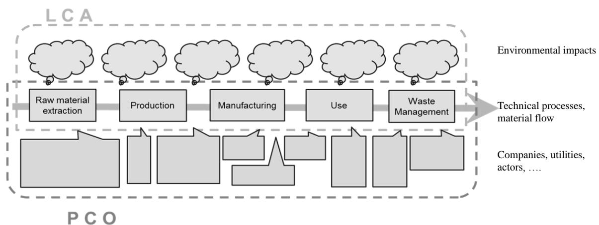
**Figure 1** An illustration of the relation between PCO and LCA. Both are following the technical processes but LCA focus on environmental impacts and PCO focus on companies, utilities, actors etc. (Figure modified from Baumann 2012).
