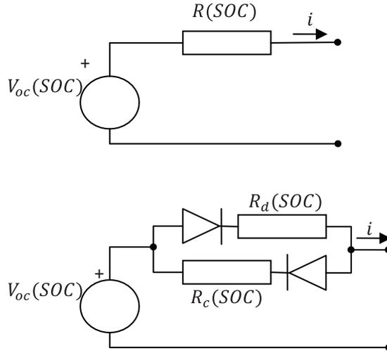
Figure 2.4: The battery equivalent circuit, as an open voltage in series with an internal resistance (upper); the resistance can have different values at charging or discharging modes (lower).
