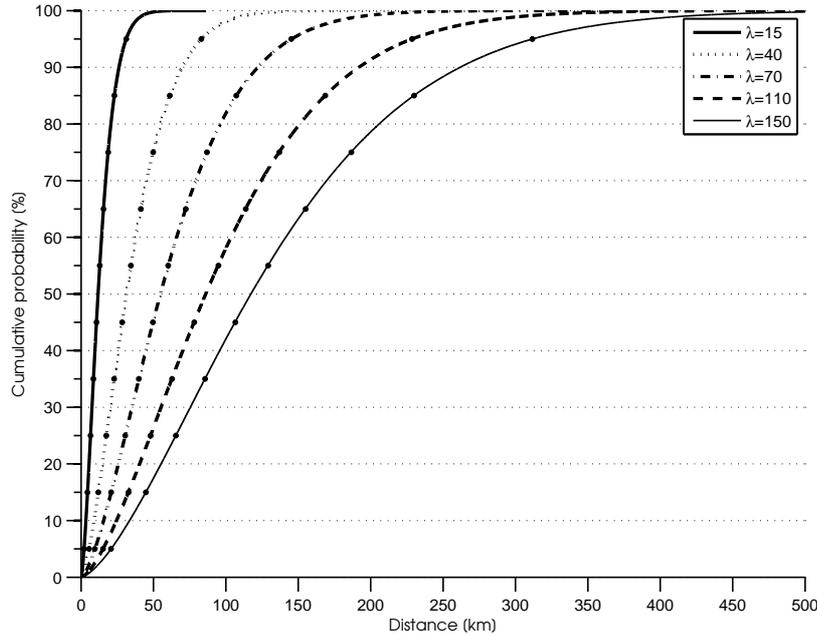
Figure 2.8: Weibull cumulative distribution function for different values of  $\lambda$  and  $k = 1.5$ .
