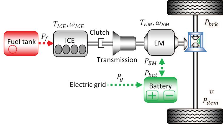
Figure 2.3: Configuration of a parallel PHEV (solid lines are the mechanical link and dashed lines are the electrical links).
