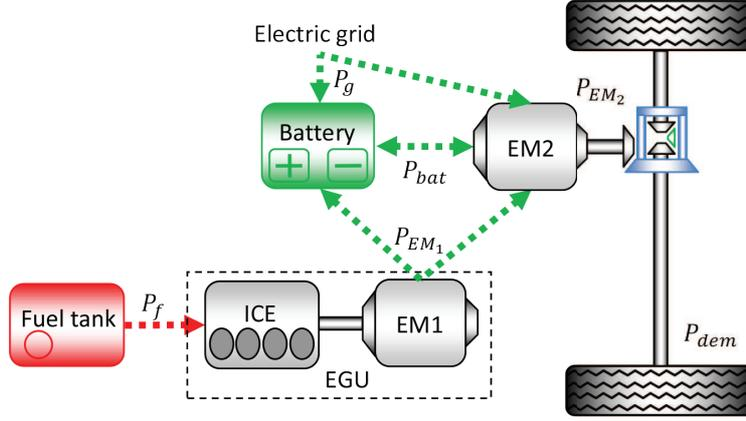
Figure 2.2: Configuration of a series PHEV (solid lines are the mechanical link and dashed lines are the electrical links).
