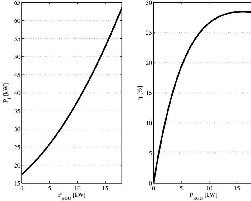
Figure 2.7: The map for a 18kW EGU.
