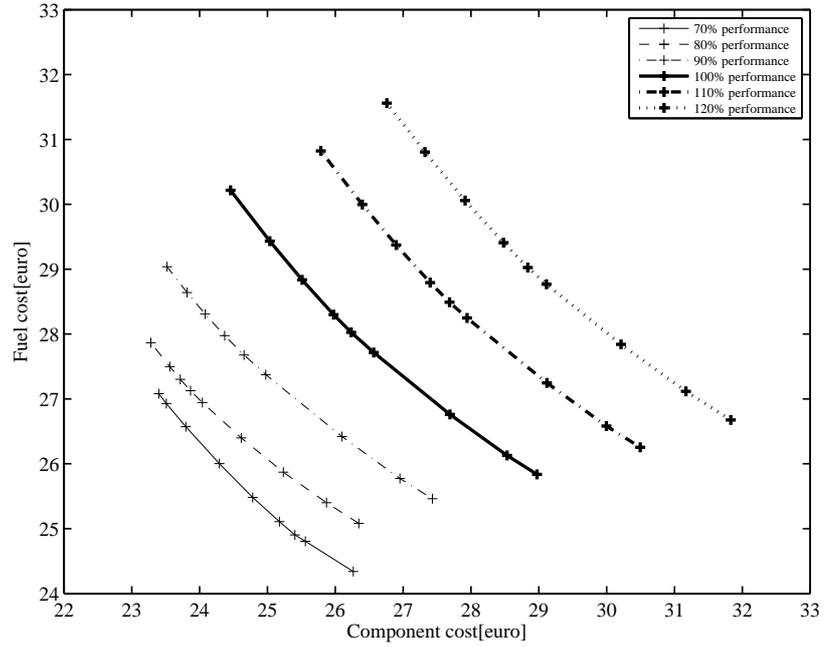
Figure 3.2: Set of pareto points obtained by using different weighting factors between fuel cost and component cost
