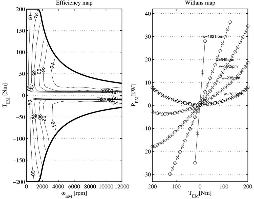
Figure 2.5: The efficiency map (left) and the Willans map (right) for a 35kW permanent magnet synchronous EM.
