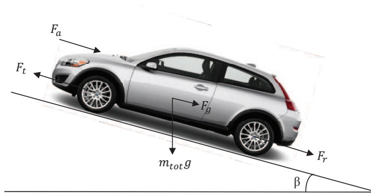
Figure 2.1: Different forces acting on a moving vehicle.
