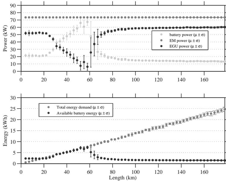
Figure 3.3: Optimal mean battery, EM, and EGU size with the standard deviations, for single trips with different lengths (upper figure); the available battery and demanded energy versus trip distance (lower figure).
