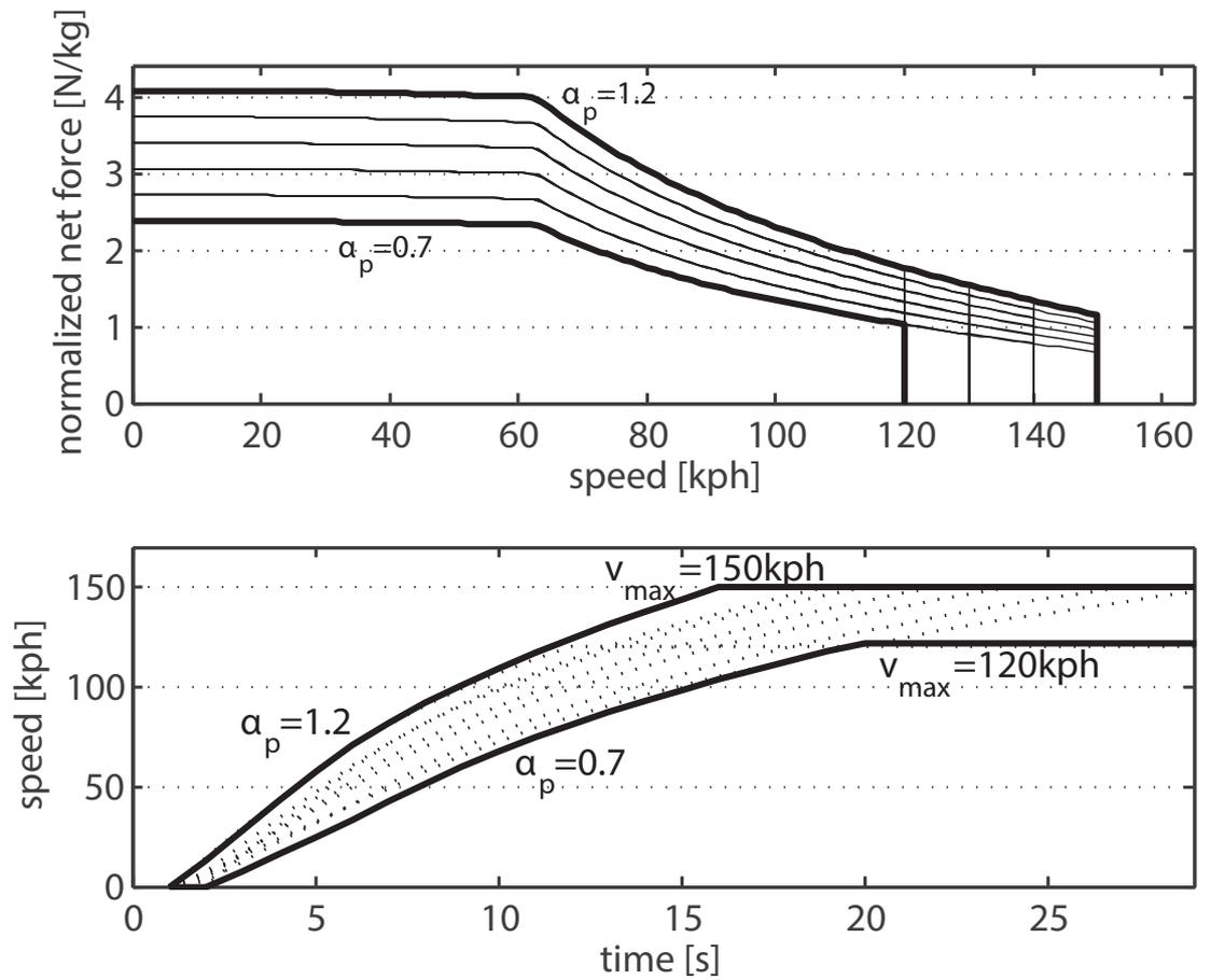
Figure 2.9: Normalized net force as a function of speed (upper), and the generated performance cycles for different levels of performance requirements (lower).
