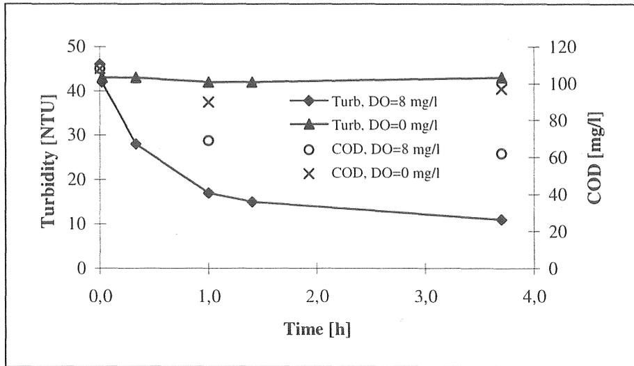
Figure 5.1-3 Change in turbidity and COD versus time (F/M=46 mg COD/g biomass; temp=10.5 °C; SVI=83).
