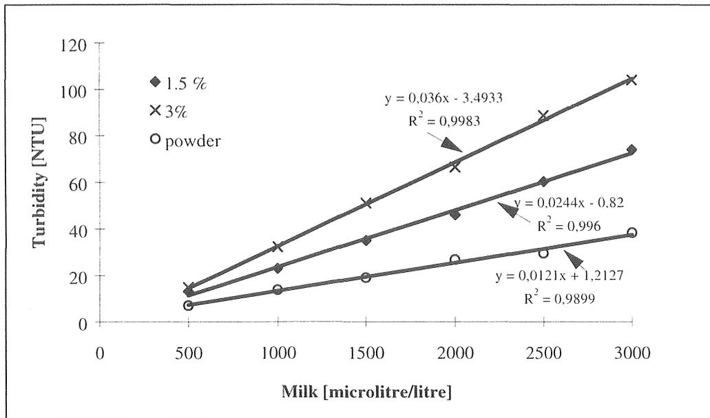
Figure 5.1-13 Relationship between added amount of milk [ $\mu\text{l/l}$ ] to tapwater and turbidity [NTU].
