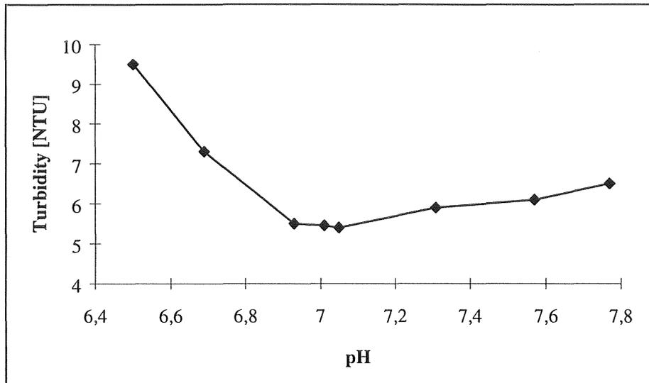
Figure 5.4-4 Turbidity of the supernatant at different pH (5 minutes stirring at 40 rpm; settling for 30 minutes).
