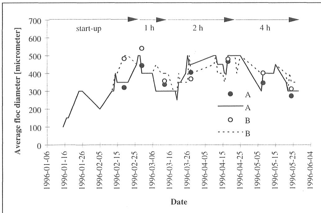
Figure 5.2-30 Average floc diameter, Part II (lines = microscope; points = Malvern instrument).
