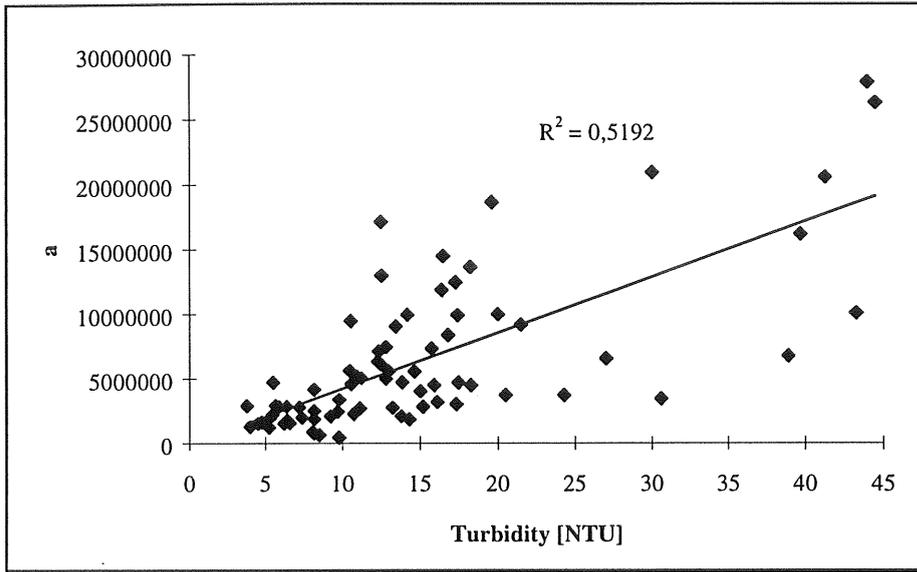
Figure 5.2-53 Correlation between the parameter  $a$  and turbidity (Part IV).
