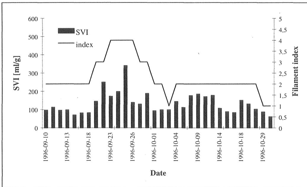
Figure 5.2-69 SVI and filament index (reactor B, Part IV).
