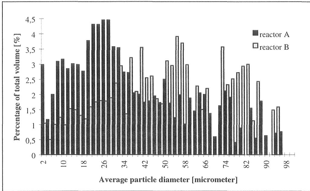
Figure 5.2-50 Distribution by volume by the end of the anaerobic period (Part II).
