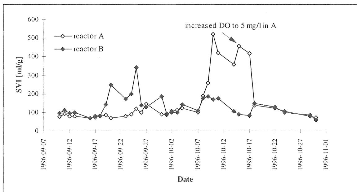
Figure 5.2-6 Change in SVI for Part IV of the experiment (A: 2 mg O<sub>2</sub>/l; B: 5 mg O<sub>2</sub>/l).
