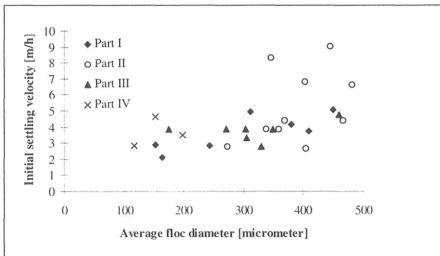
**Figure 5.2-27 Correlation between average floc diameter and initial settling velocity (Part I-IV).**
