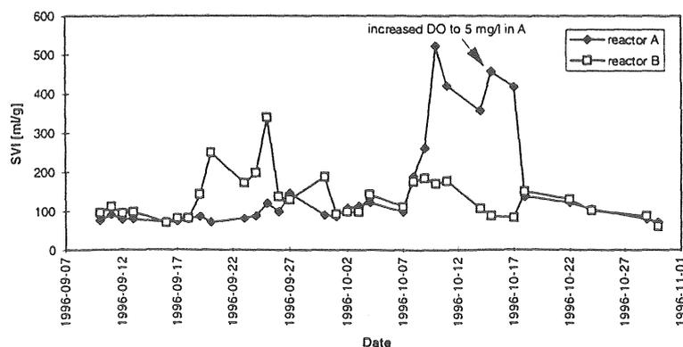
Figure 6. Change in SVI for part IV of the experiment (A: 2.0 mg O<sub>2</sub>/l; B: 5.0 mg O<sub>2</sub>/l).
