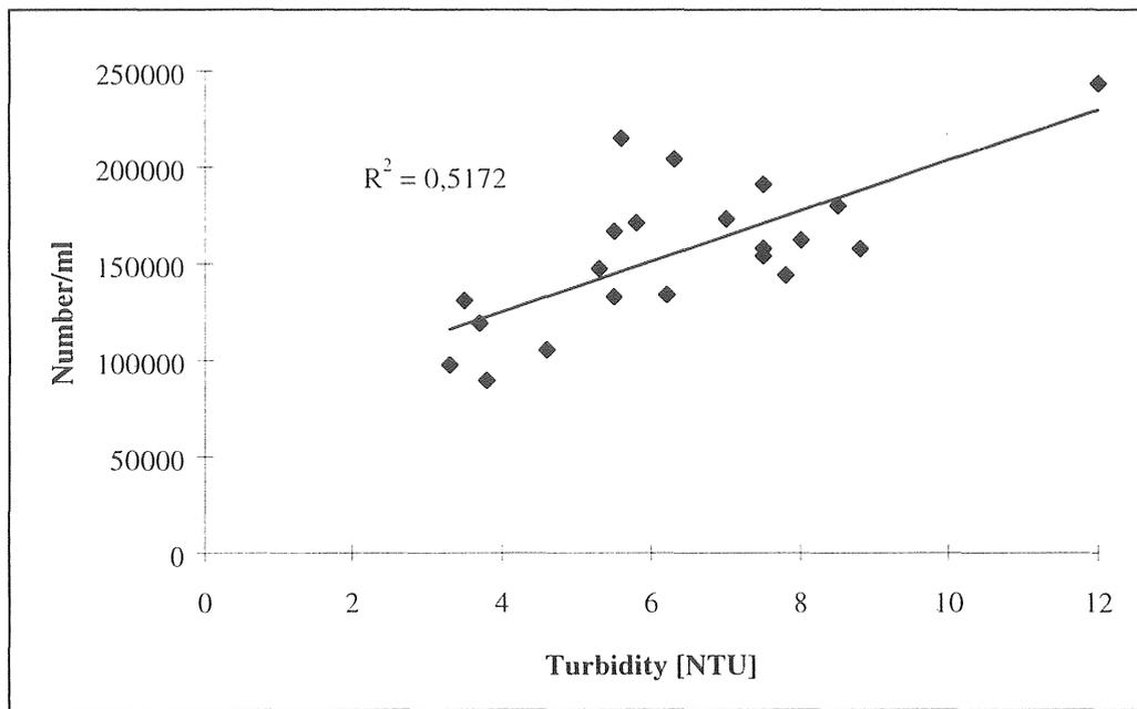
Figure 5.2-41 Correlation between number of particles per ml and turbidity (Part III).
