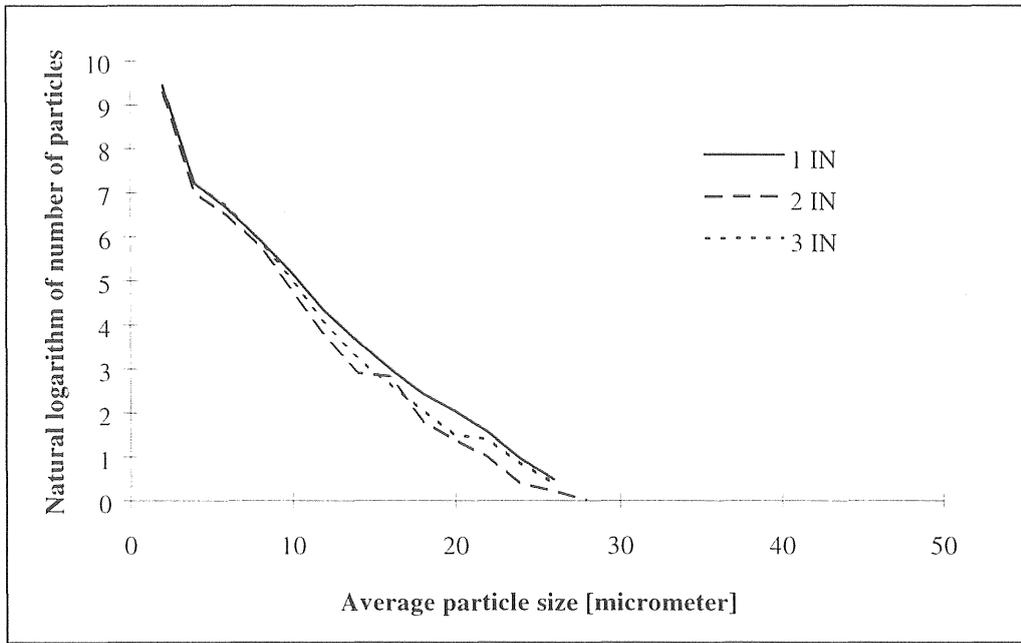
Figure 5.2-48 The natural logarithm of the number of particles in the pre-settled wastewater by the time of 1) end 1<sup>st</sup> oxic period; 2) end anoxic period; 3) end 2<sup>nd</sup> oxic period.
