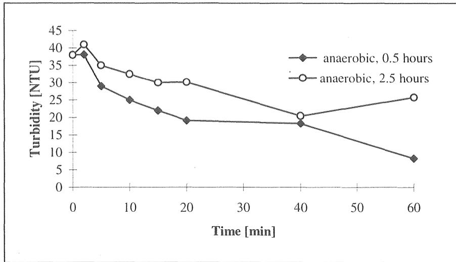
Figure 5.1-11 Change in turbidity versus time for return sludge which has been stored anaerobically for 0.5-2.5 hours (F/M=28 mg COD/g biomass)
