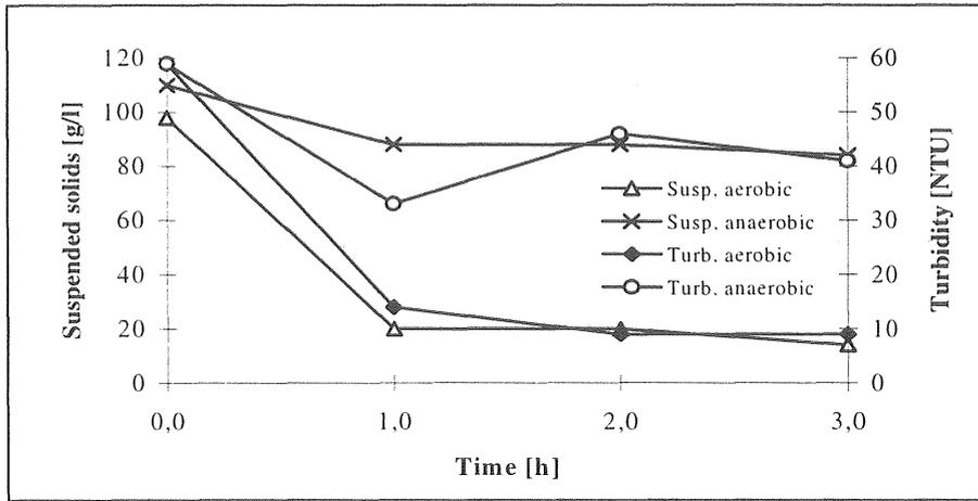
Figure 5.1-1 Turbidity and suspended solids concentration versus time (F/M=34 mg COD/g biomass; temp=15.5 °C; SVI=100 ml/g).
