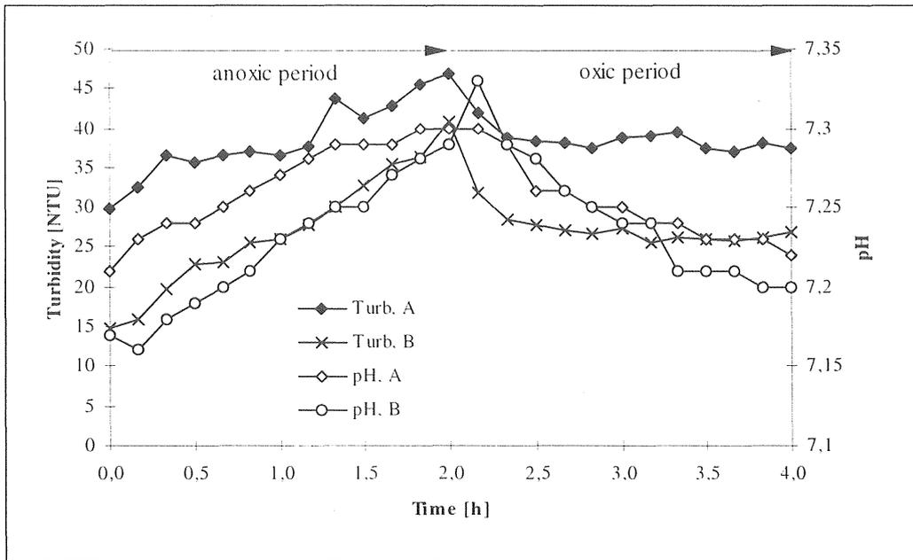
Figure 5.2-21 Change in turbidity and pH during a 4-hour-cycle, Part IV (960918).
