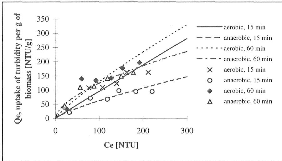
Figure 5.1-21 Data fitted to Freundlich isotherms after 15 and 60 minutes contact time (test I, milk with 3% fat).
