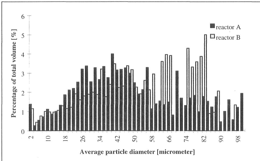
Figure 5.2-51 Distribution by volume by the end of the first aerobic period (Part II).
