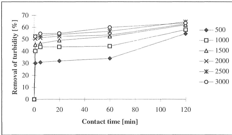
Figure 5.1-23 Percentage removal of turbidity (NTU) versus time at anaerobic conditions (test II).
