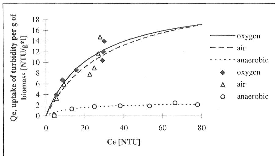
Figure 5.1-19 Data fitted to Langmuir isotherms after 15 minutes contact time (test II, powder milk).
