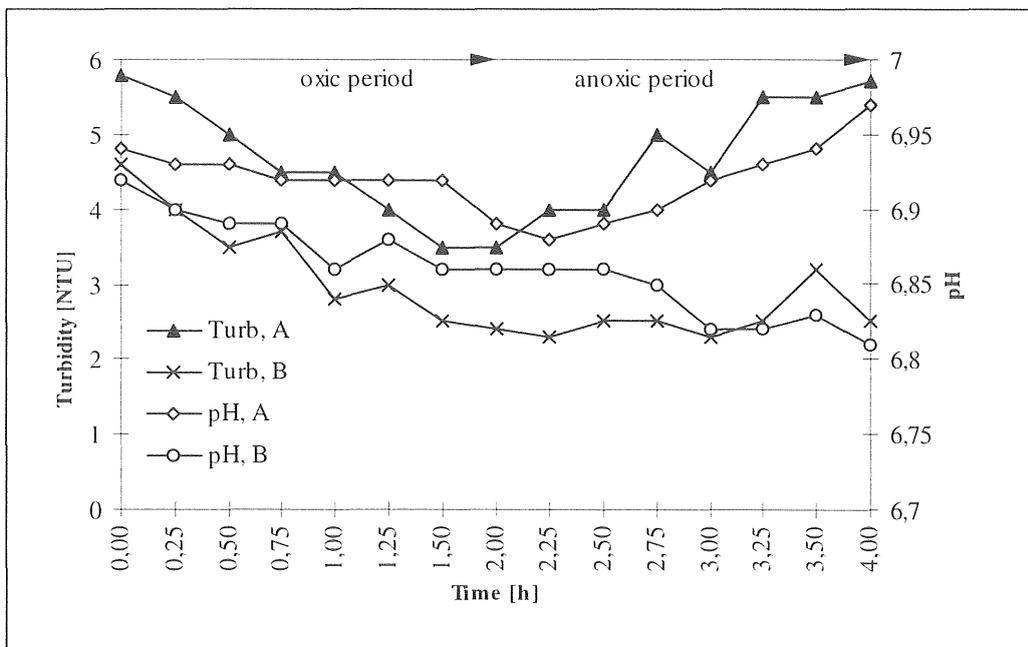
Figure 5.2-12 The change in turbidity and pH during a 4-hour-cycle without influent, Part II (960417).
