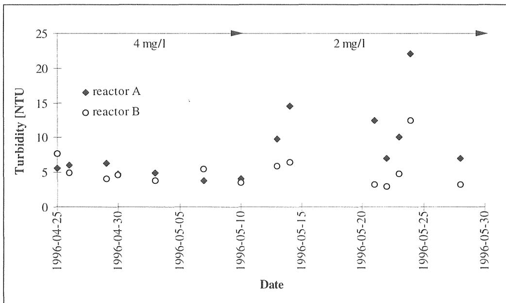
Figure 5.2-9 Turbidity after 20 minutes settling at an alternating period of 4 hours (Part II).
