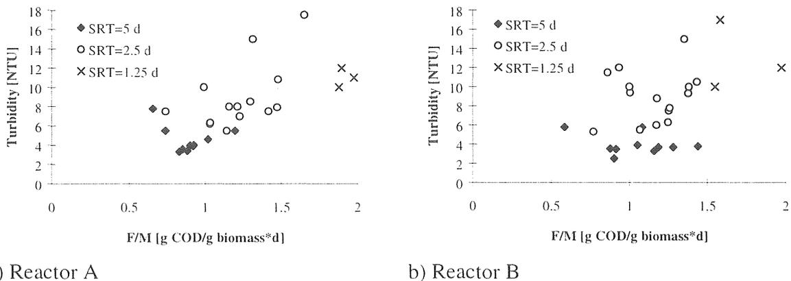
Figure 5.2-23 Turbidity vs organic loading (20 minutes settling), Part III.
