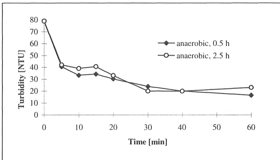
Figure 5.1-10 Change in turbidity versus time for return sludge which has been stored anaerobically for 0.5-2.5 hours (F/M=29 mg COD/g biomass)
