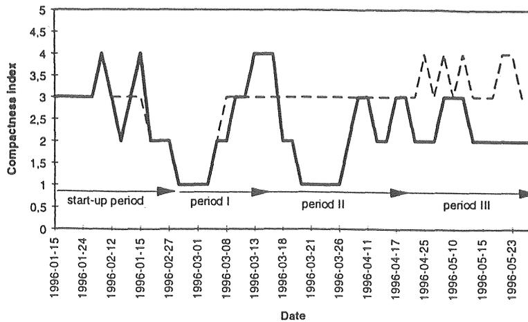
Figure 4 a. Compactness index for part II of the experiment (dotted line=A; continuous line=B; period I=1 h; period II=2 h; period III=4 h; A: alternating oxic/anoxic conditions; B: constant oxic conditions).
