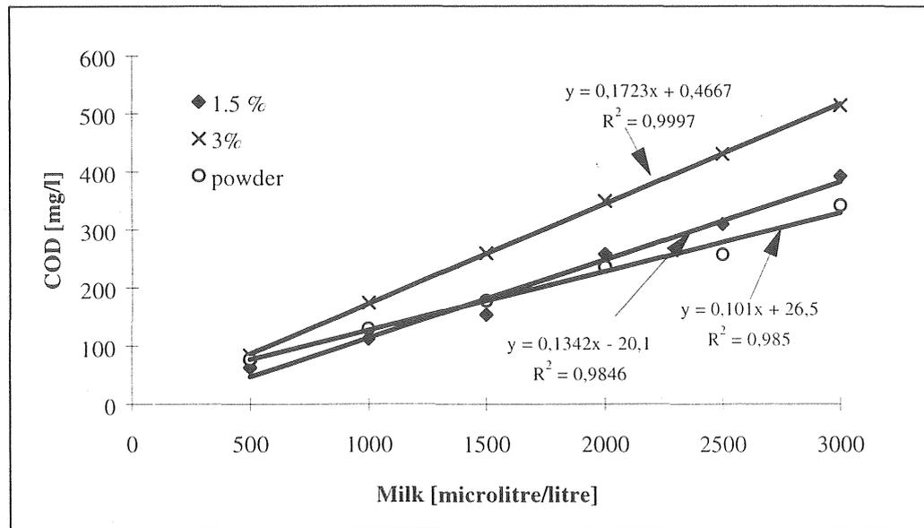
Figure 5.1-14 Relationship between added amount of milk [ $\mu\text{l/l}$ ] to pre-settled wastewater and COD [ $\text{mg O}_2/\text{l}$ ].
