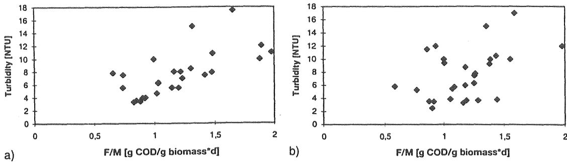
Figure 9. Turbidity vs organic loading, part III; a) reactor A, 0.5 mg O<sub>2</sub>/l; b) reactor B, 2 mg O<sub>2</sub>/l.
