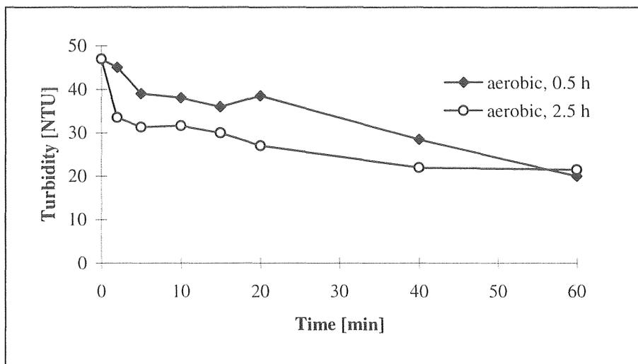
Figure 5.1-12 Change in turbidity versus time for return sludge which has been stored aerobically for 0.5-2.5 hours (F/M=92 mg COD/g biomass)
