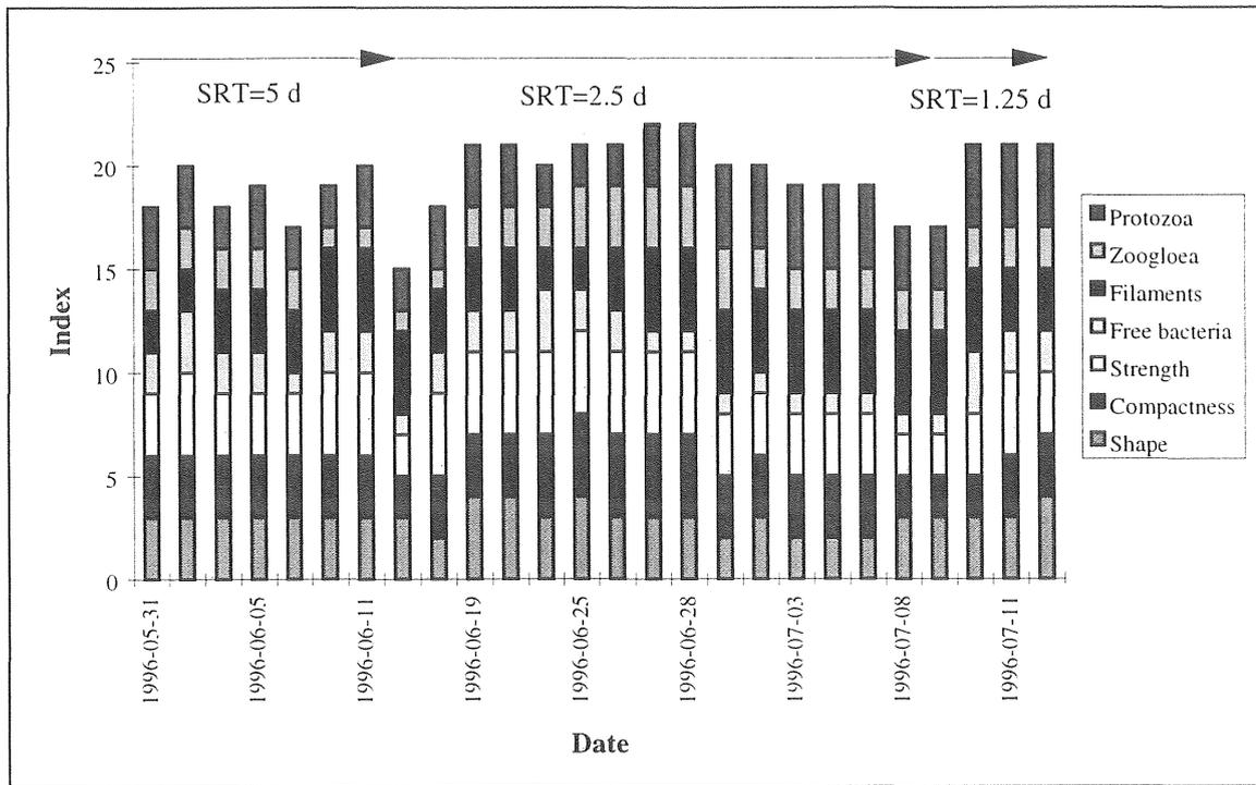
Figure 5.2-59 Classification of the sludge morphology according to a scale from 1-5 (Part III; reactor A).
