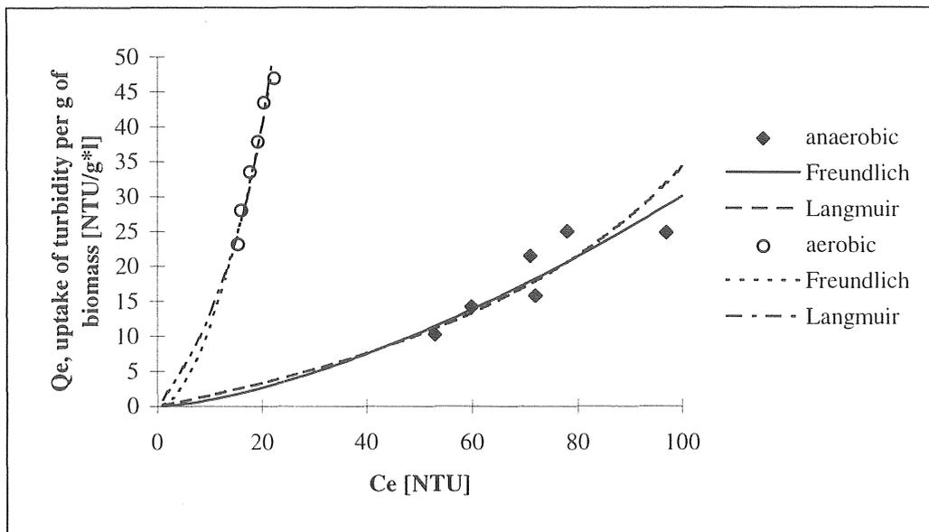
Figure 5.1-17 Adsorption data fitted to Freundlich and Langmuir isotherms after 60 minutes contact time (test I, milk with 1.5 % fat).
