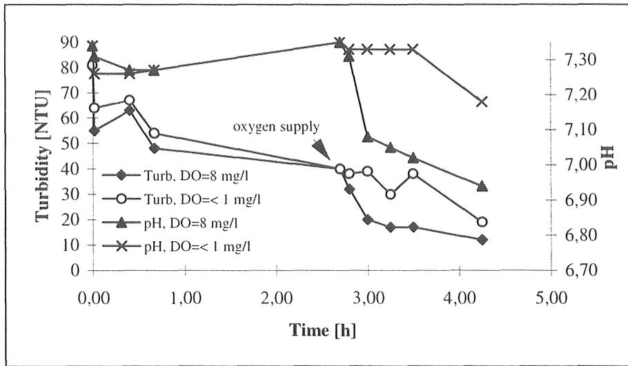
Figure 5.1-9 Change in turbidity and pH versus time (F/M=65 mg COD/g biomass; temp=11 °C; SVI=65 ml/g).
