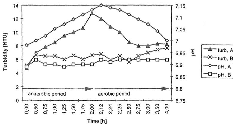
Figure 8a. Change in turbidity and pH during a 4-hour-cycle with influent, part II of the experiment (A: alternating oxic/anoxic conditions; B: constant oxic conditions).
