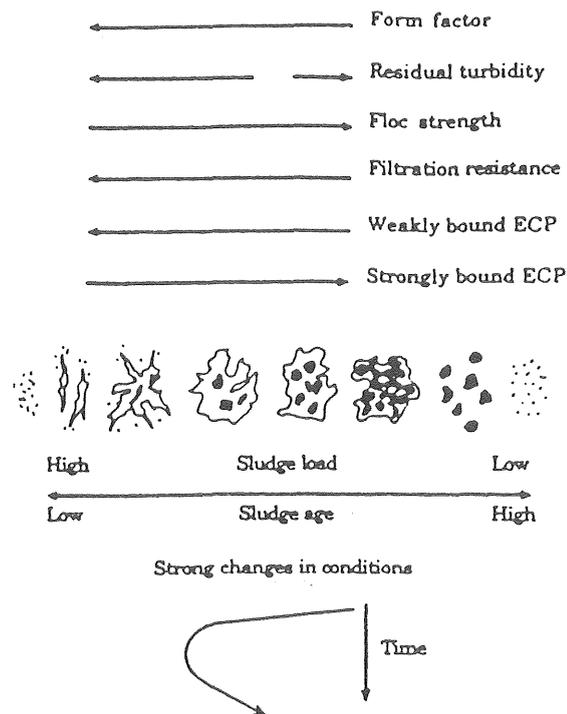
Figure 3.4-1 A general model for flocs built by floc forming activated sludge bacteria (Eriksson *et al*, 1992).
