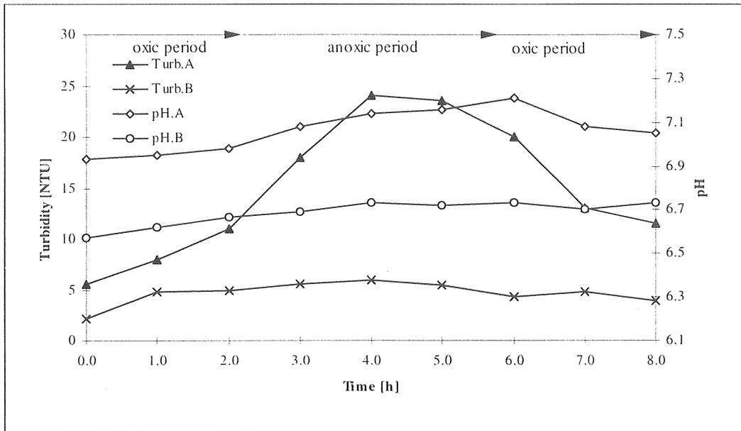
Figure 5.2-13 Change in turbidity and pH during an 8-hour-cycle, Part II (960515).
