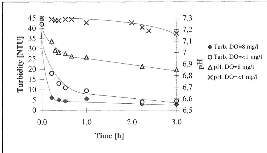
Figure 5.1-5 Change in turbidity and pH for a DO concentration of 8 and  $\leq 1$  mg/l (F/M=19 mg COD/g biomass; temp=15 °C; SVI=80 ml/g).
