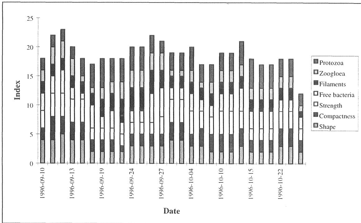
Figure 5.2-62 Classification of the sludge morphology according to a scale from 1-5 (Part IV; reactor B).
