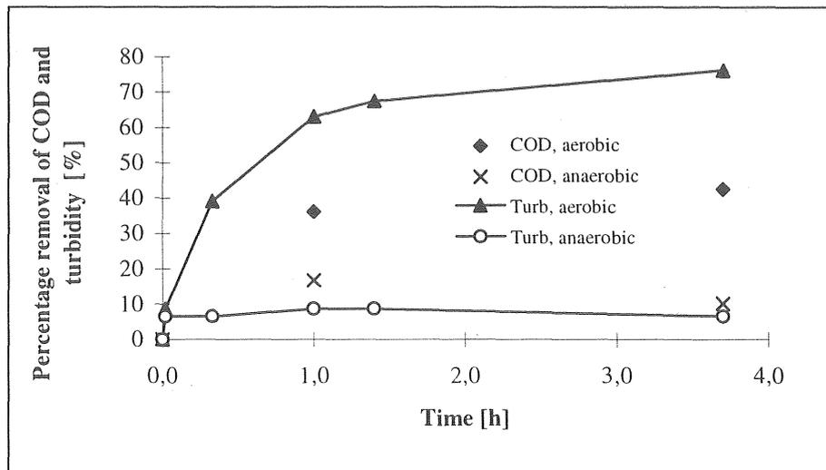
Figure 5.1-4 Percentage removal of turbidity and COD versus time (F/M=46 mg COD/g biomass; temp=10.5 °C; SVI=83).
