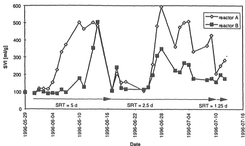
Figure 5. Change in SVI for part III of the experiment (A: 0.5 mg O<sub>2</sub>/l; B: 2.0 mg O<sub>2</sub>/l).
