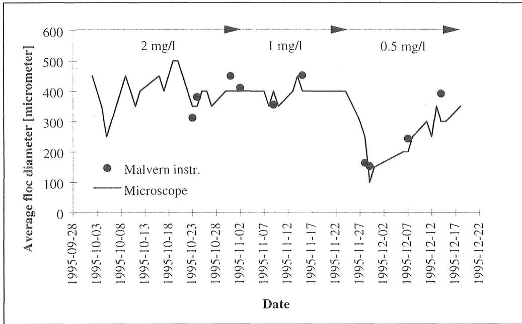
Figure 5.2-29 Average floc diameter, Part I (line = microscope; points = Malvern instrument).
