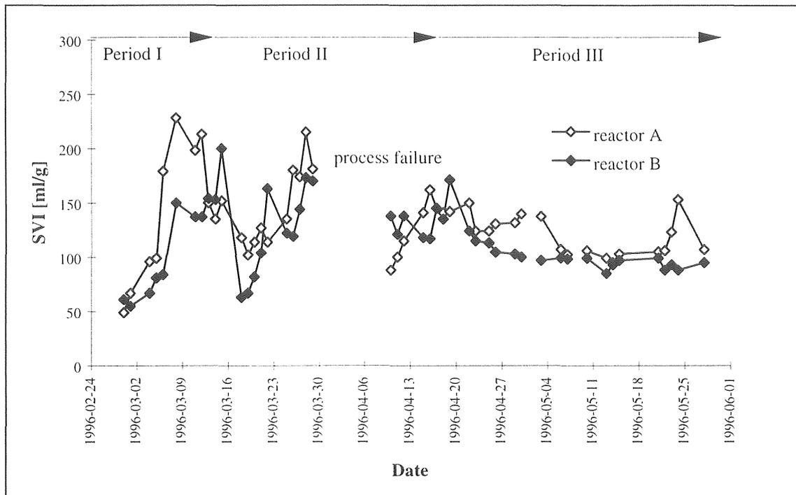
Figure 5.2-4 Change in SVI for Part II of the experiment (B: constant oxic conditions; A: alternating oxic/anoxic conditions; period I=1 h; period II=2 h; period III=4 h).
