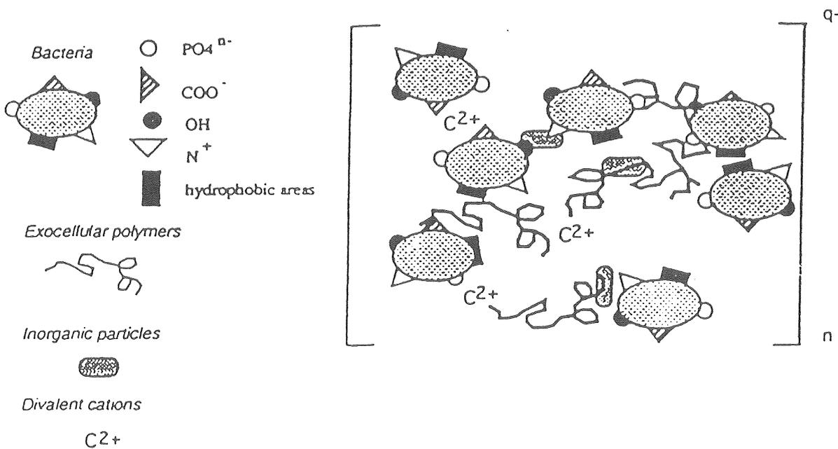
Figure 3.3-1 Schematic presentation of an activated sludge floc (Urbain *et al*, 1993).
