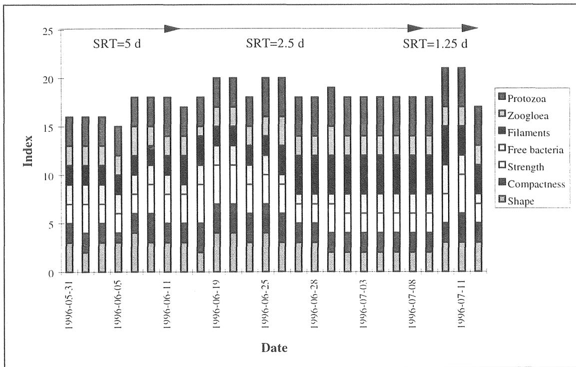
Figure 5.2-60 Classification of the sludge morphology according to a scale from 1-5 (Part III; reactor B).
