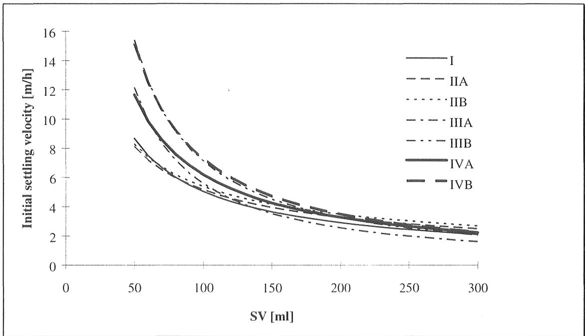
Figure 5.2-25 Relationship between SV and initial settling velocity (power functions).
