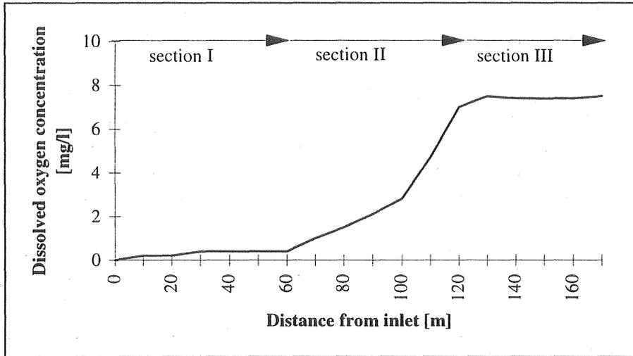
**Figure 4.3-2 Example of a DO concentration profile.**
