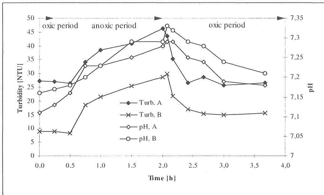
Figure 5.2-20 Change in turbidity and pH during a 4-hour-cycle, Part IV (960917).
