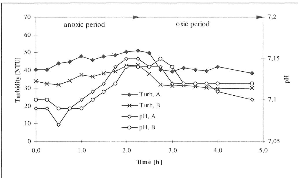
Figure 5.2-22 Change in turbidity and pH during a 4-hour-cycle, without influent, Part IV (960926).
