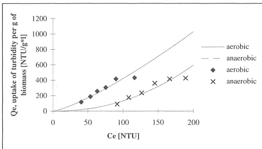
Figure 5.1-22 Data fitted to Freundlich isotherms after 20 minutes contact time (test II, milk with 3 % fat).
