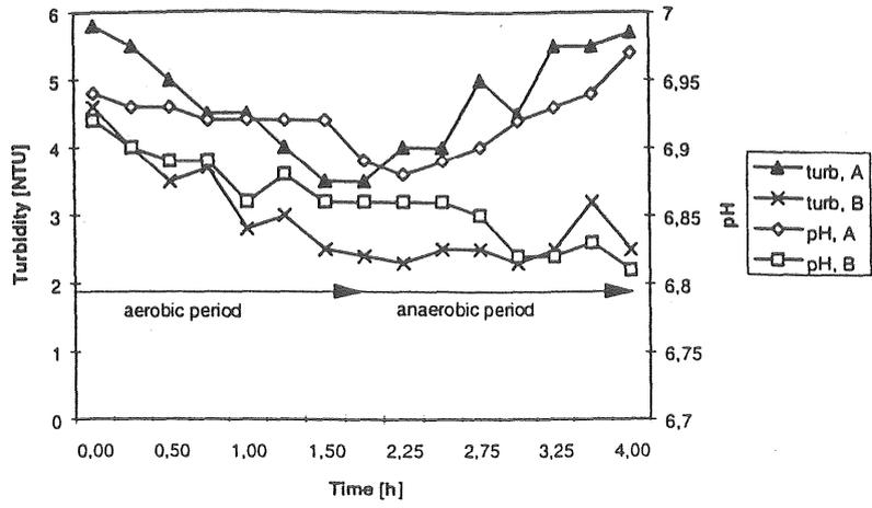
Figure 8b. Change in turbidity and pH during a 4-hour-cycle without influent, part II of the experiment (A: alternating oxic/anoxic conditions; B: constant oxic conditions).
