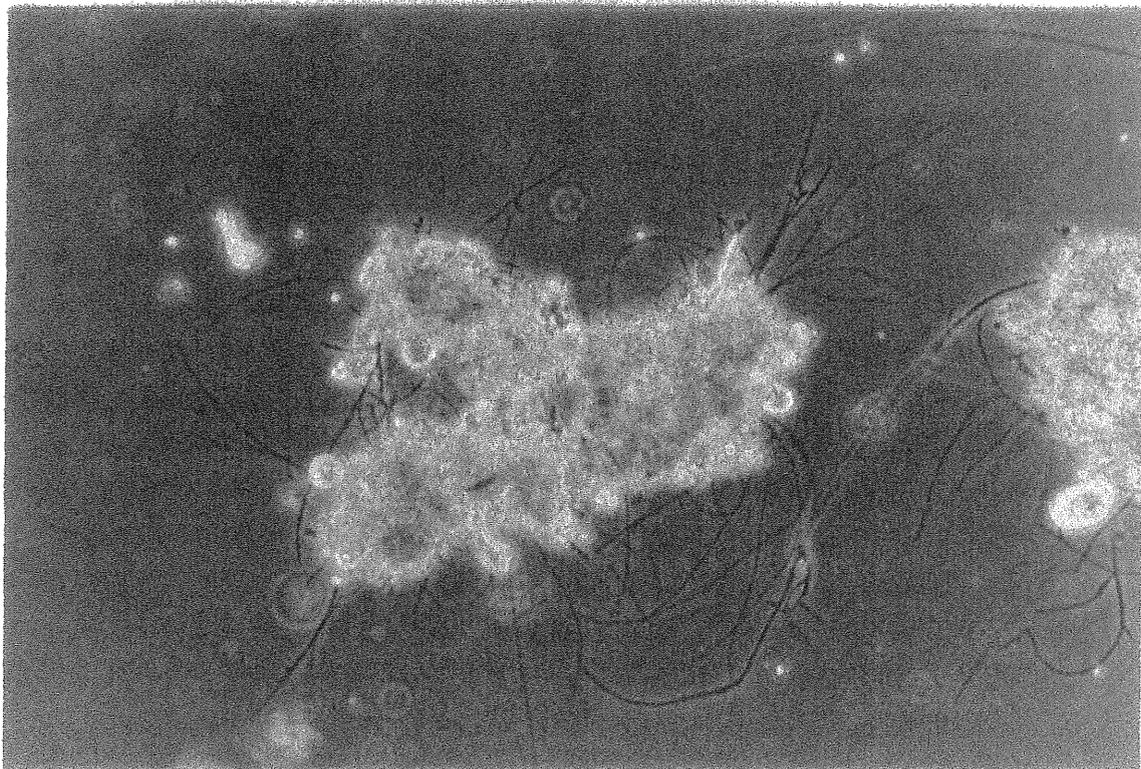
Figure 5.2-77 Round (category 2) and porous (category 3) floes containing filaments (category 3) (960703, Part III: reactor A, SRT=2.5 d, magnification 100x).
