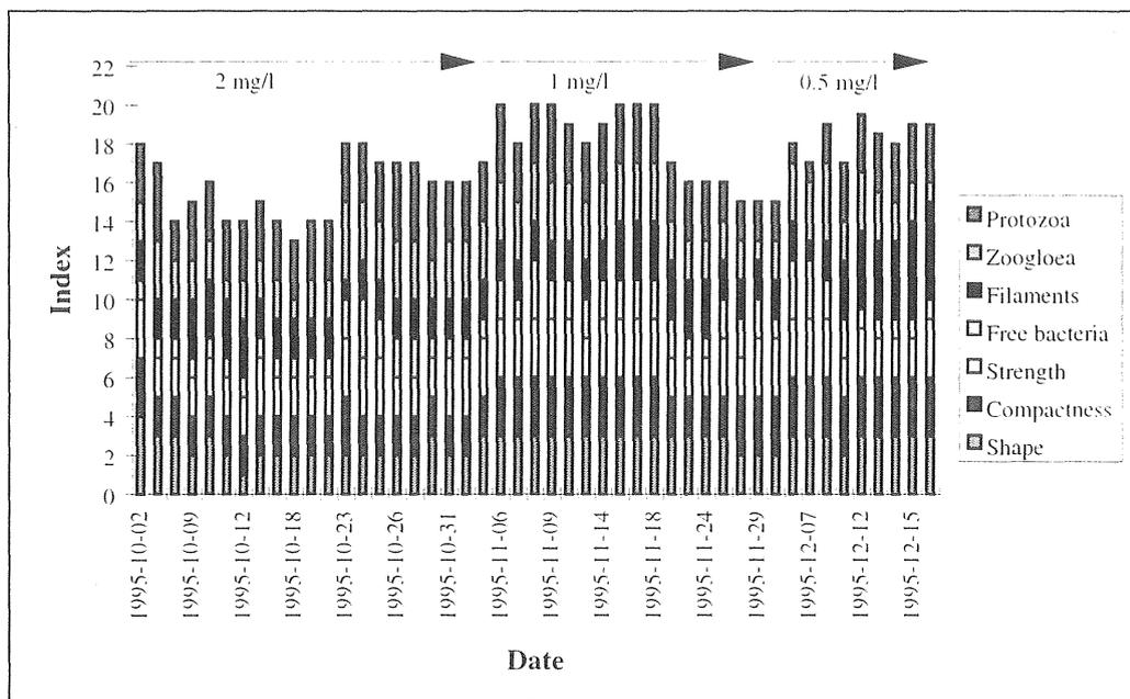
Figure 5.2-56 Classification of the sludge morphology according to a scale from 1-5 (number of free bacteria, filaments, Zoogloea, protozoa: 1=no present, 5=excessive numbers; shape, compactness, strength: 1=round and compact and strong, 5=very irregularly shaped, porous and weak (Part I).
