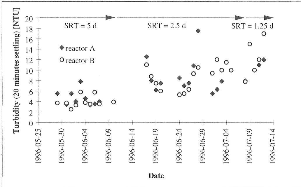
Figure 5.2-16 Turbidity in the supernatant after 20 minutes settling (Part III).
