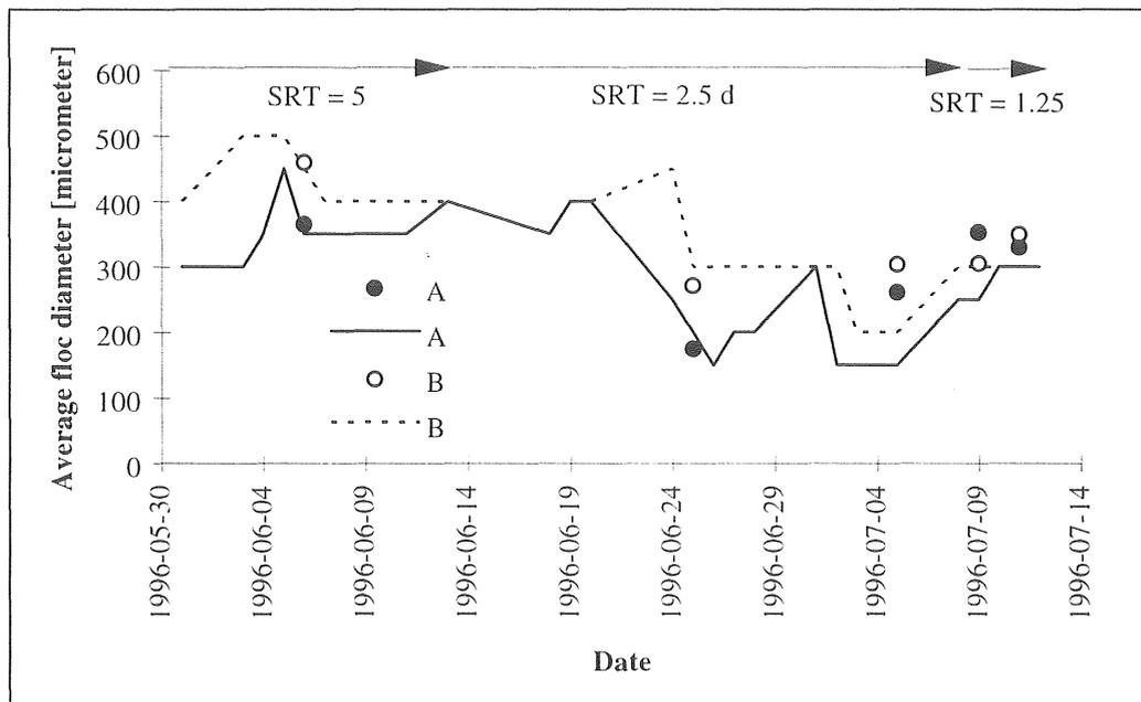
Figure 5.2-31 Average floc diameter, Part III (lines = microscope; points = Malvern instrument).
