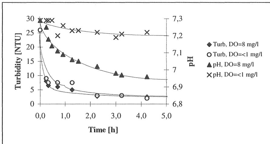
Figure 5.1-6 Change in turbidity and pH versus time (F/M=20 mg COD/g biomass; temp=15.5 °C; SVI=100 ml/g).
