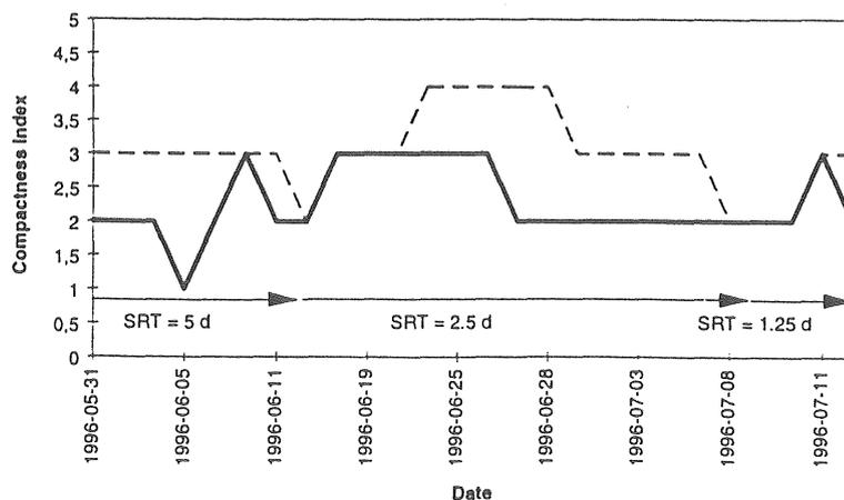
Figure 4 b. Compactness index, part III (dotted line=A; continuous line=B; A: 0.5 mg O<sub>2</sub>/l; B: 2.0 mg O<sub>2</sub>/l).
