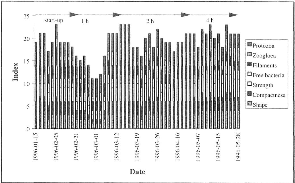
Figure 5.2-57 Classification of the sludge morphology according to a scale from 1-5 (Part II; reactor A).
