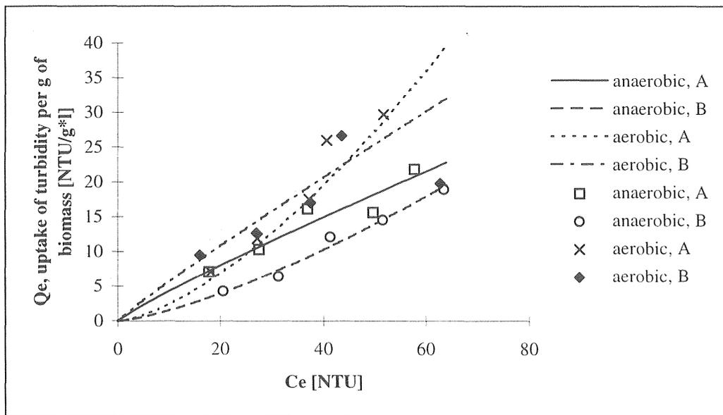
Figure 5.1-26 Data fitted to Freundlich isotherms after 20 minutes contact time (test IV, milk with 1.5 % fat).
