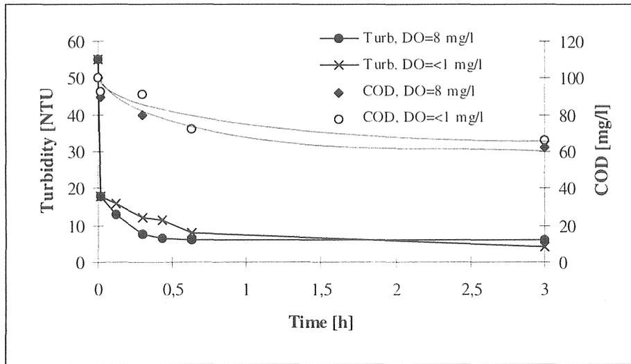
Figure 5.1-7 Change in turbidity and COD versus time (F/M=40 mg COD/g biomass; temp=13 °C; SVI=112 ml/g).
