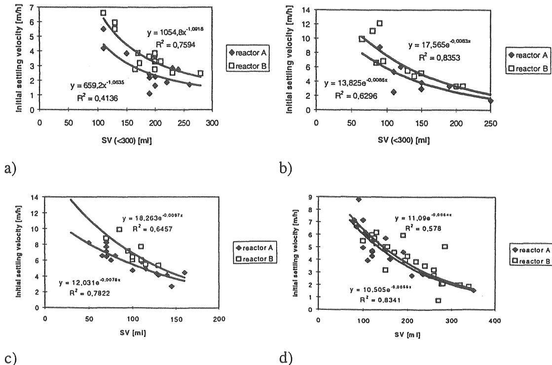
Figure 15. Relationship between SV and initial settling velocity at: a) part III (SRT = 2.5 d); b) part III (SRT = 5 d); c) part II (alternating period of 4 hours); d) part IV (A = 2.0 mg O<sub>2</sub>/l; B = 5.0 mg O<sub>2</sub>/l).
