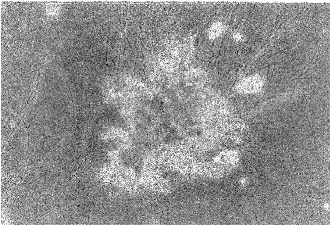
Figure 5.2-75 Irregularly shaped (category 3), and rather porous (category 3) flocs containing large numbers of filaments (category 5) (951215, Part I, magnification 100x).
