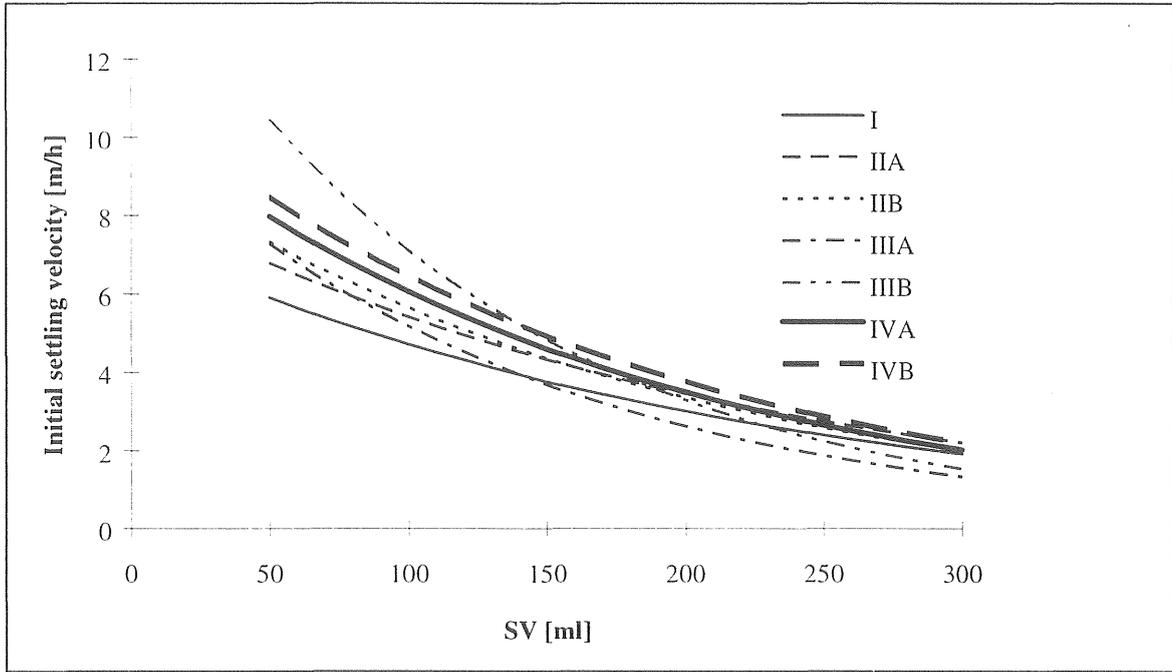
Figure 5.2-24 Relationship between SV and initial settling velocity (exponential functions).
