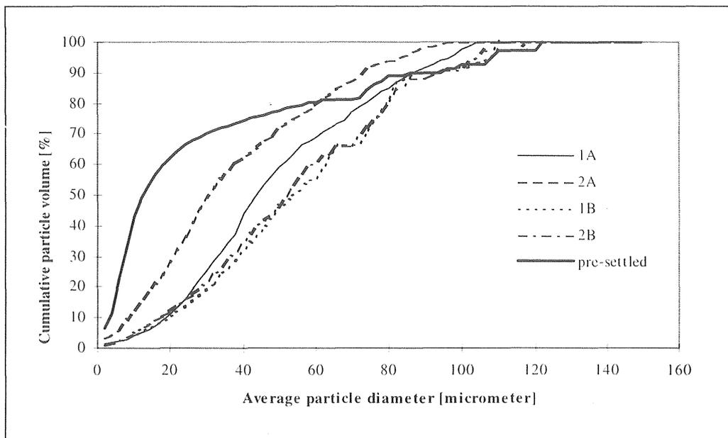
Figure 5.2-49 Particle size distributions in pre-settled wastewater, after the 1<sup>st</sup> oxic period (1) and after the anoxic period (2).
