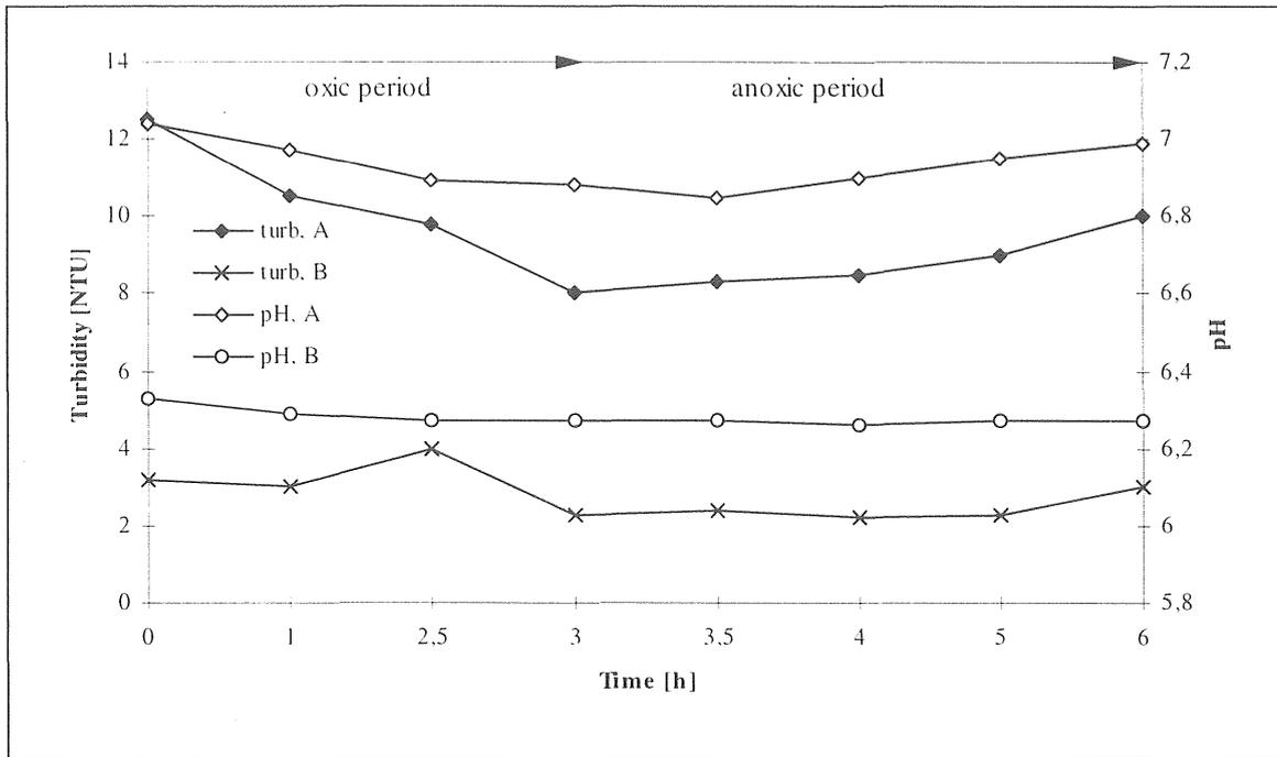
Figure 5.2-15 Change in turbidity and pH during an 8-hour-cycle without influent, Part II (960521).
