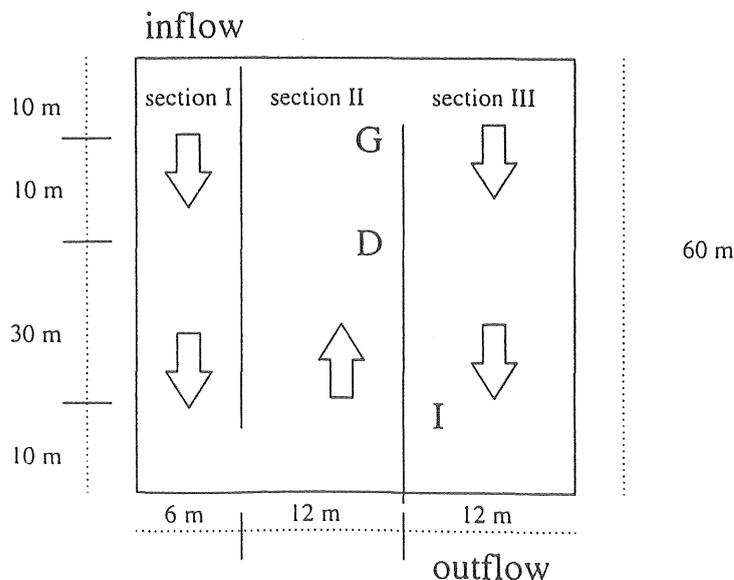
Figure 4.3-1 Schematic presentation of the aeration tank (not drawn to scale): D, G and I are on-line DO-meters; the arrows represent the flow direction of the water.
