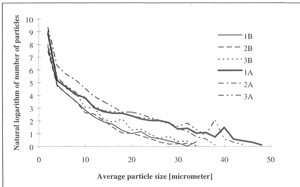
Figure 5.2-47 The natural logarithm of the number of particles within the different size intervals 1) end 1<sup>st</sup> oxic period; 2) end anoxic period; 3) end 2<sup>nd</sup> oxic period.
