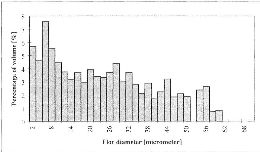
Figure 5.2-39 Example of a size distribution by volume in the supernatant (20 minutes settling).
