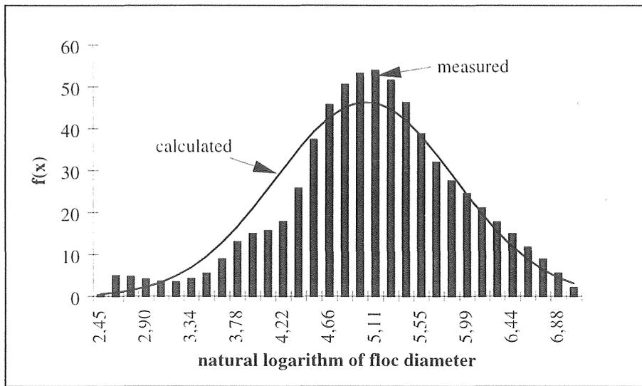
Figure 5.2-36 A size distribution fitted to a log-normal distribution function ( $r^2=0.9$ ).
