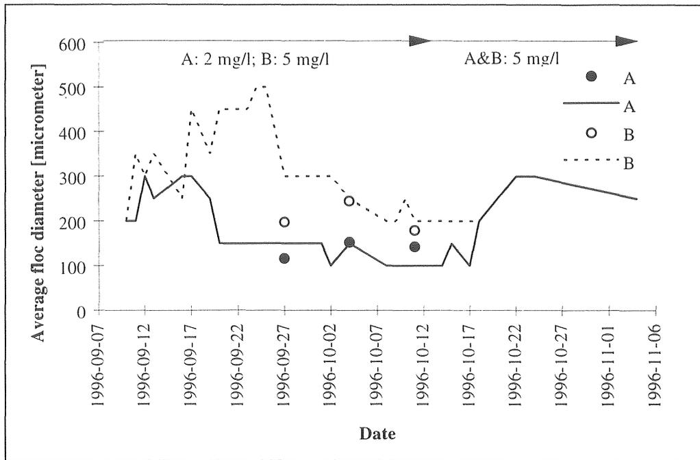
Figure 5.2-32 Average floc diameter, Part IV (lines = microscope; points = Malvern instrument).
