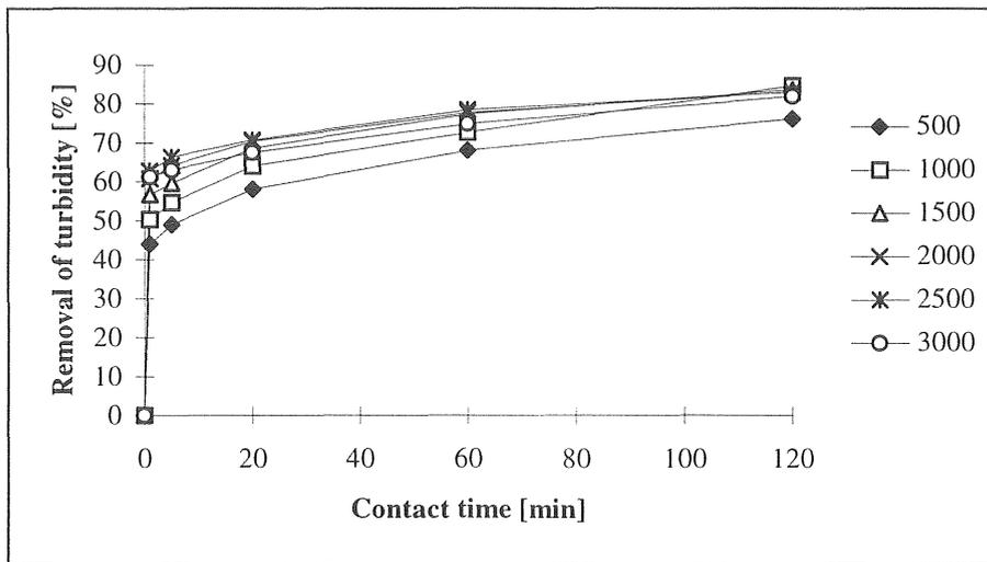
Figure 5.1-24 Percentage removal of turbidity (NTU) versus time at aerobic conditions (test II).
