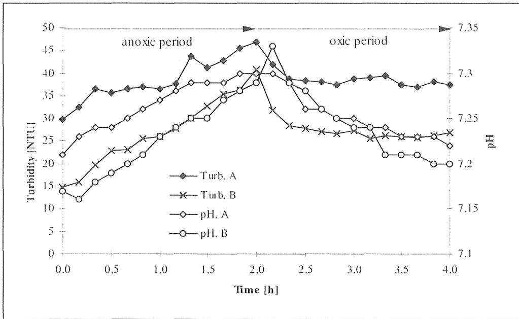
Figure 5.2-11 The change in turbidity and pH during a 4-hour-cycle, Part II (960415).
