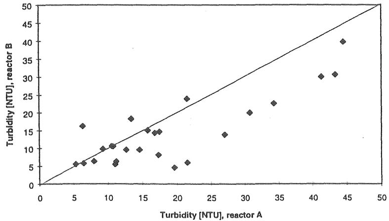
Figure 10. Turbidity after 20 minutes settling, part IV (A=2 mg O<sub>2</sub>/l; B=5 mg O<sub>2</sub>/l).
