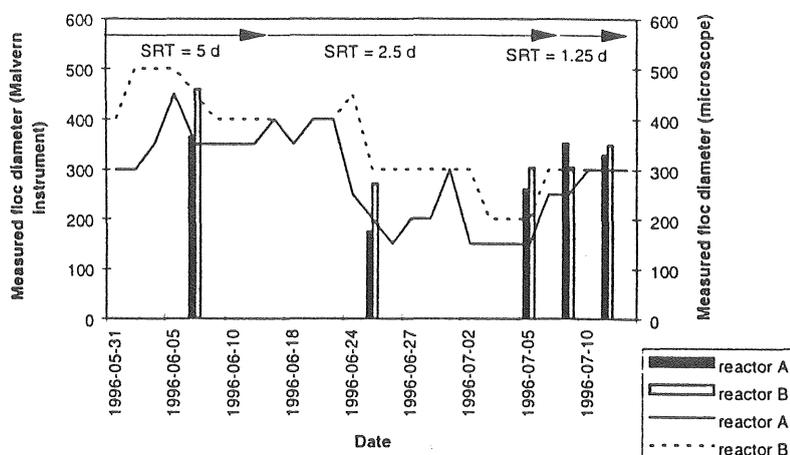
Figure 12. Average floc diameter, part III (line = microscopic measurement; bar = particle analyser measurement).
