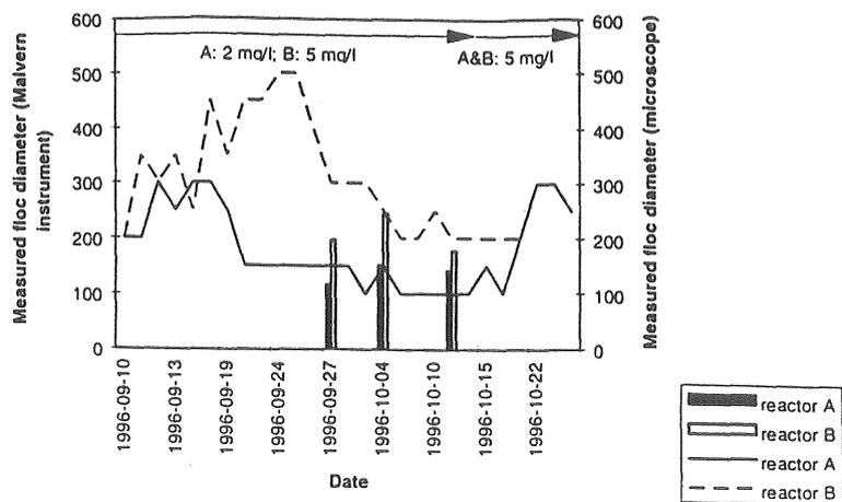
Figure 13. Average floc diameter, part IV (line = microscopic measurement; bar = particle analyser measurement).
