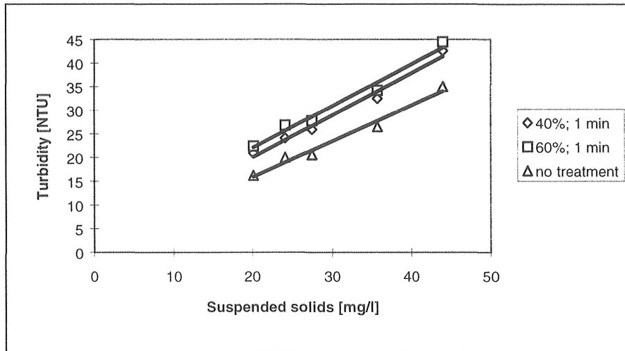
**Figure 2 Relationship between turbidity and suspended solids concentration at different degrees of ultrasound treatment.**
