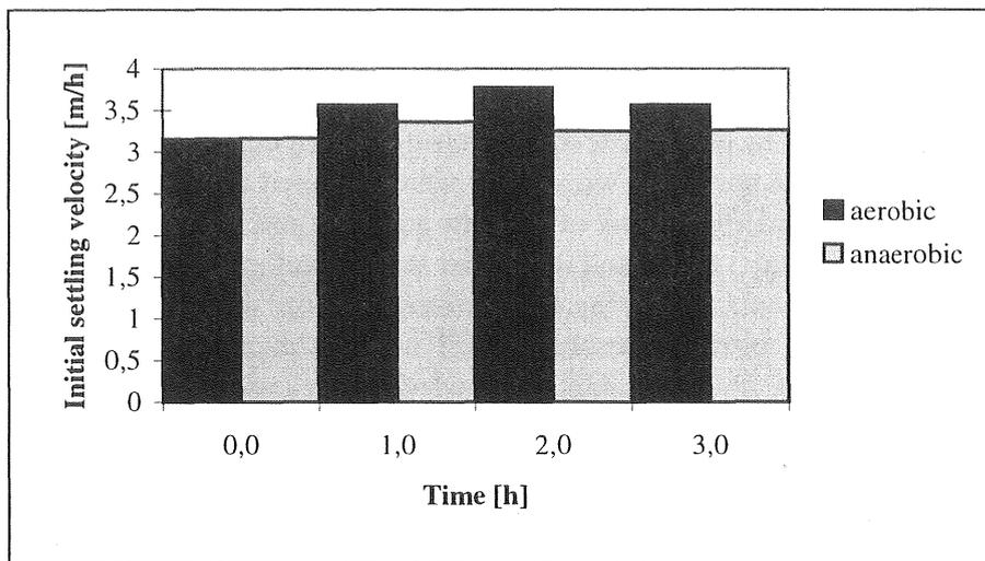
Figure 5.1-2 Change in initial settling velocity with time.
