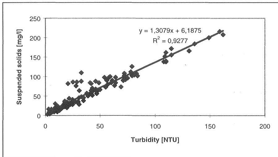
Figure 1 Turbidity as a function of suspended solids concentration.
