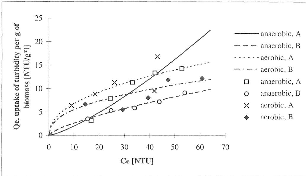
Figure 5.1-25 Data fitted to Freundlich isotherms after 20 minutes contact time (test III, milk with 1.5 % fat).
