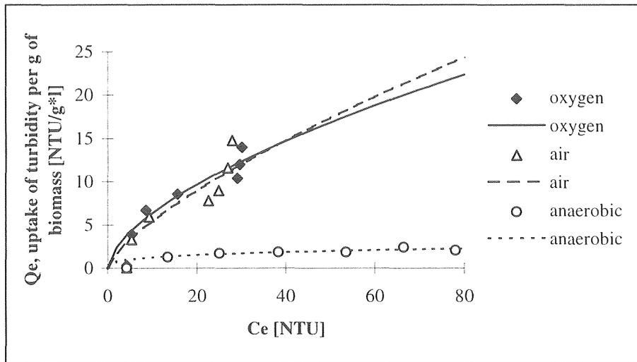
Figure 5.1-18 Data fitted to Freundlich isotherms after 15 minutes contact time (test II, powder milk).
