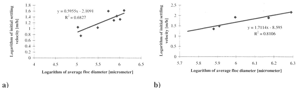
**Figure 5.2-28 Relationship between average floc diameter and initial settling velocity (logarithmic values) for Part I and Part II (reactor B) of the experiment.**
