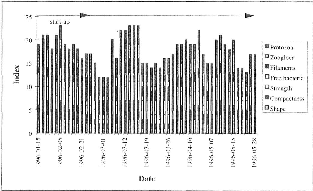
Figure 5.2-58 Classification of the sludge morphology according to a scale from 1-5 (Part II; reactor B).
