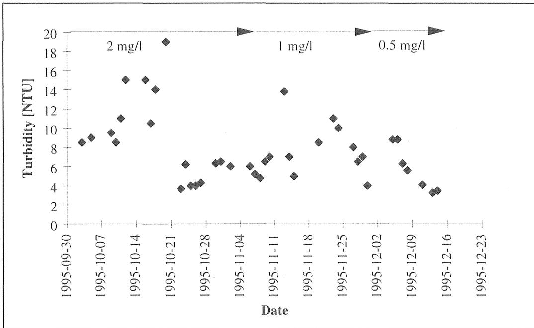
Figure 5.2-7 Turbidity in the supernatant after 20 minutes settling (Part I).
