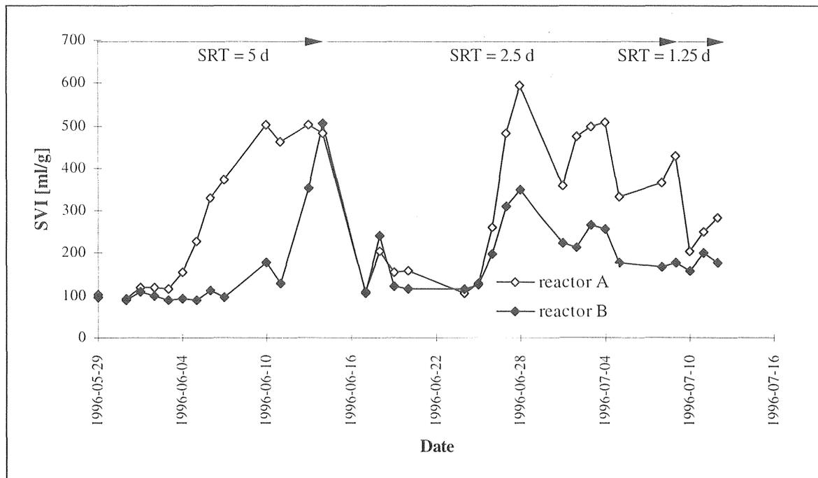
Figure 5.2-5 Change in SVI for Part III of the experiment (A: 0.5 mg O<sub>2</sub>/l; B: 2.0 mg/l).
