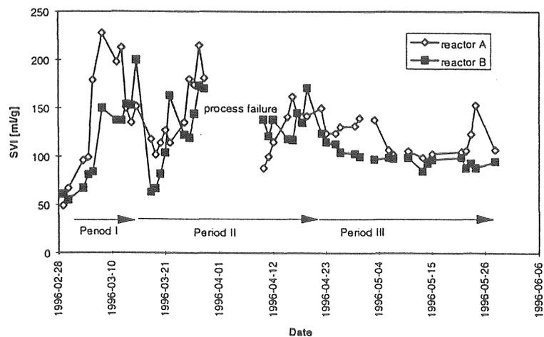
Figure 3. Change in SVI for part II of the experiment (period I=1 h; period II=2 h; period III=4 h; A: alternating oxic/anoxic conditions; B: constant oxic conditions).
