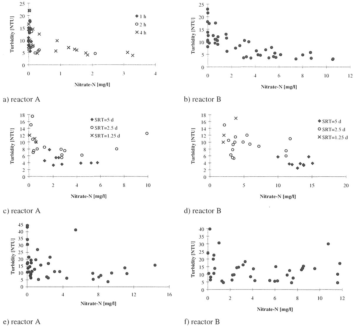
**Figure 5.4-2** Turbidity versus nitrate concentration: a-b) Part II (the labels correspond to the different alternating oxic and anoxic periods for reactor A); c-d) Part III (the labels correspond to the different sludge ages); e-f) Part IV.
