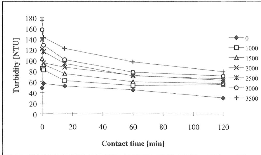
Figure 5.1-15 Decrease in turbidity at different colloidal loadings (test I: anaerobic conditions).
