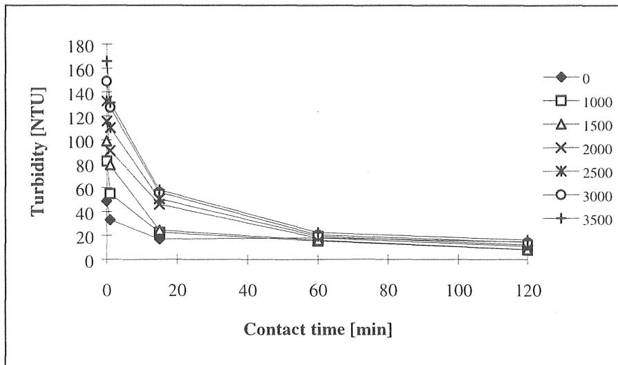
Figure 5.1-16 Decrease in turbidity at different colloidal loadings (test I: aerobic conditions).
