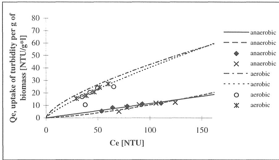
Figure 5.1-20 Data fitted to Freundlich isotherms after 15 minutes contact time (test III, milk with 1.5% fat).
