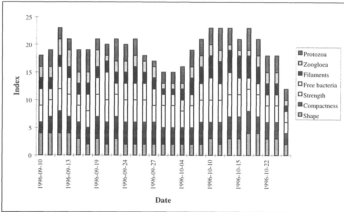
Figure 5.2-61 Classification of the sludge morphology according to a scale from 1-5 (Part IV; reactor A).
