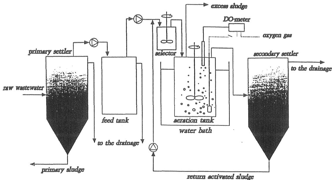
Figure 1. Schematic drawing of the pilot-plant.
