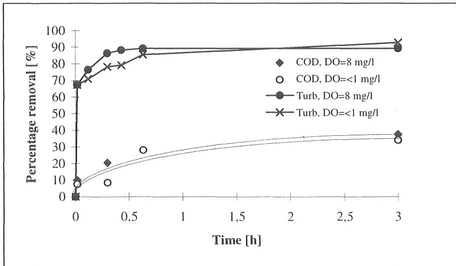
Figure 5.1-8 Percentage removal of turbidity and COD versus time (F/M=40 mg COD/g biomass; temp=13 °C; SVI=112 ml/g).
