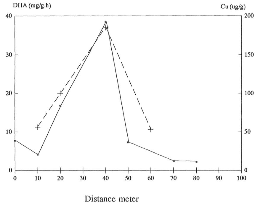
Figure 7. Variation of DHA and Cu concentration downstream from a CSO discharge.
