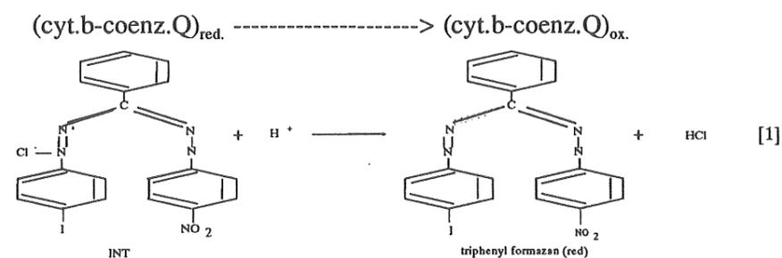
INT is reduced to formazan, an insoluble red precipitate, according to the above reaction. Following incubation, the produced formazan is dissolved in an organic solvent and the red color is measured at 480 nm. Dehydrogenase is expressed as a rate,  $\mu\text{g}$  formazan per gram biological material per incubation time.
