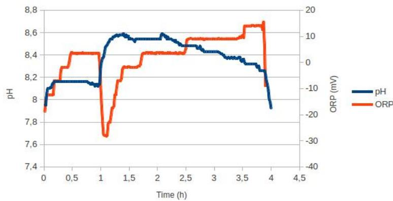
Figure 4.66: pH and ORP trend in R2 during second run
