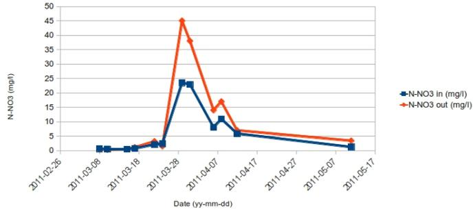
Figure 4.20: Influent and effluent nitrate in R2
