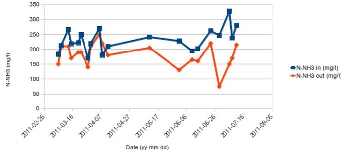
Figure 4.27: Influent vs effluent ammoniacal nitrogen in R3
