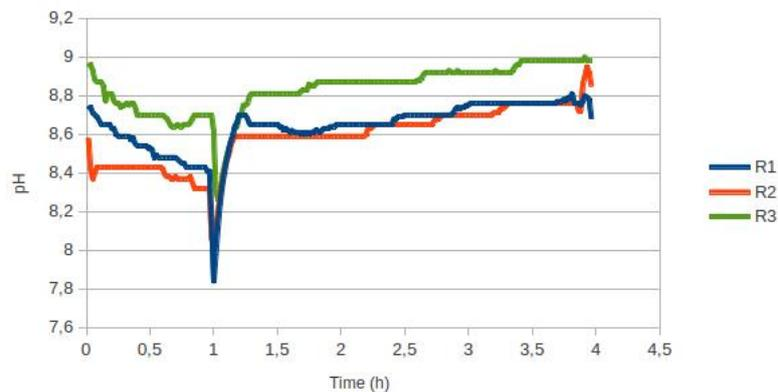
Figure 4.60: pH trend in R1, R2 and R3 before nitrification had started
