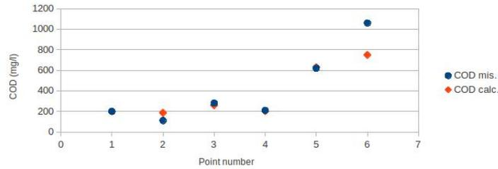
Figure 6.1: COD measured vs COD calculated
