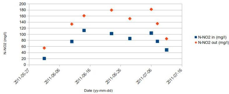
Figure 4.25: Influent and effluent nitrite concentration in R2 during second run
