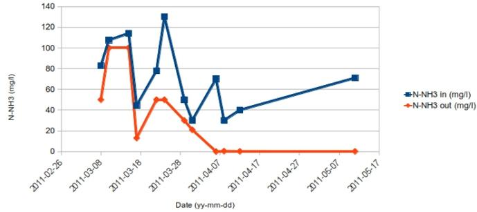
Figure 4.18: Influent and effluent ammoniacal nitrogen in R2
