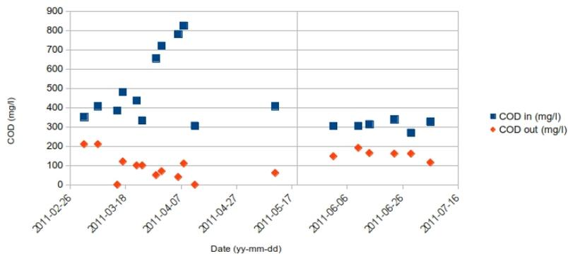
Figure 4.7: Influent and effluent COD in R2
