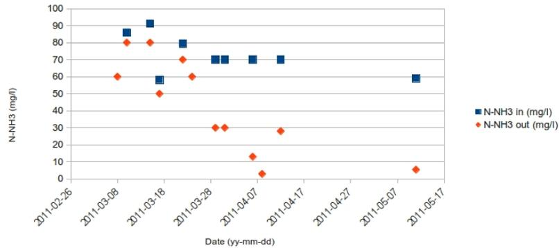
Figure 4.12: Influent ammoniacal nitrogen vs effluent ammoniacal nitrogen in R1
