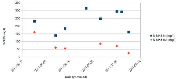
Figure 4.13: Influent and effluent ammoniacal nitrogen in R1 during second run
