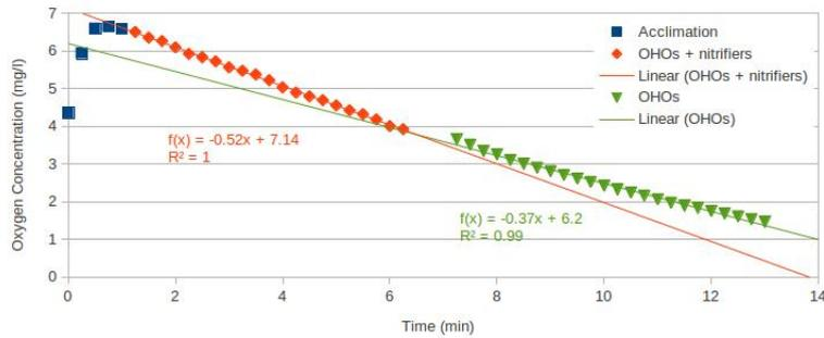
Figure 4.38: OUR test with 30 ml of settled granules for R1
