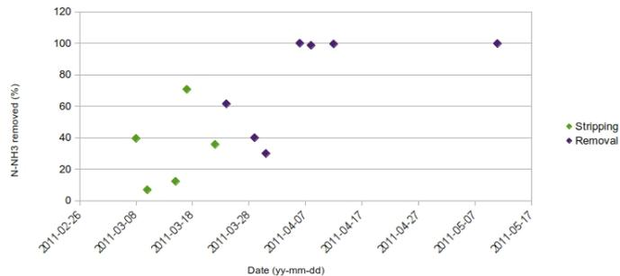
Figure 4.19: Ammonia removal efficiency for R2
