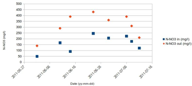
Figure 4.24: Influent and effluent nitrate concentration in R2 during second run
