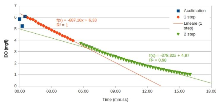
Figure 4.37: OUR analysis with synthetic water for R1
