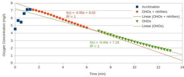
Figure 4.40: OUR test with 30 ml of settled granules for R3
