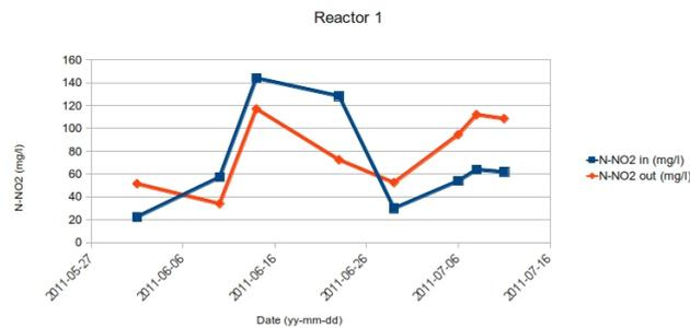
Figure 4.16: Influent and effluent nitrite concentration in R1 during second run
