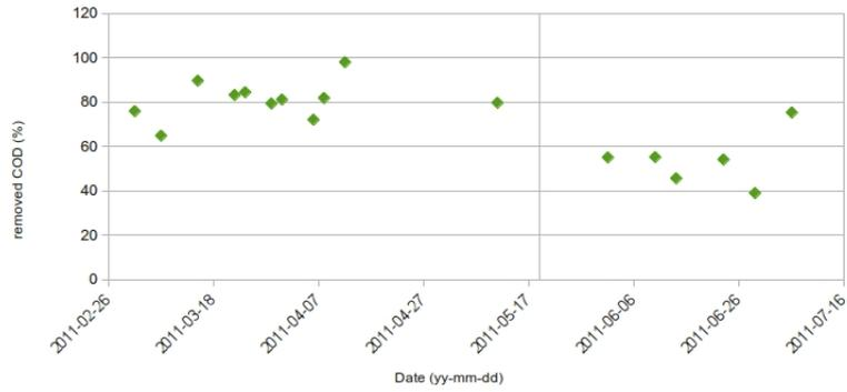
Figure 4.3: COD removal efficiency in R1
