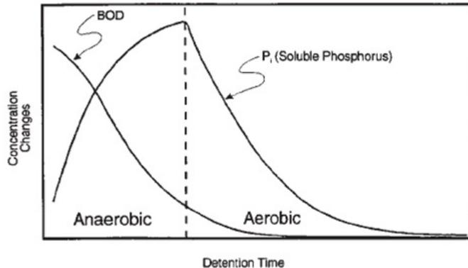
Figure 1.2: BOD and phosphate concentration trend during aerobic and anaerobic conditions
