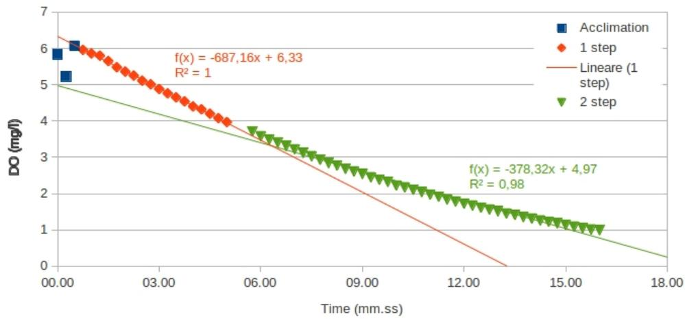
Figure 3.2: Plot example obtained with the OUR test (ATU added at the beginning of step 2).
