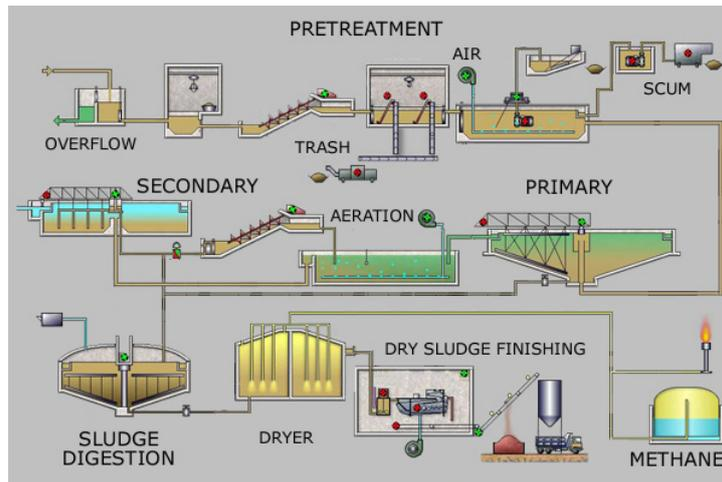
Figure 1.3: Wastewater treatment plant scheme
