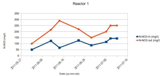
Figure 4.15: Influent and effluent nitrate concentration in R1 during second run
