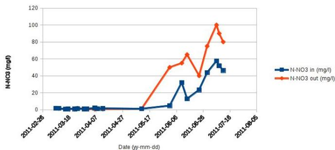
Figure 4.28: Influent and effluent nitrate in R3
