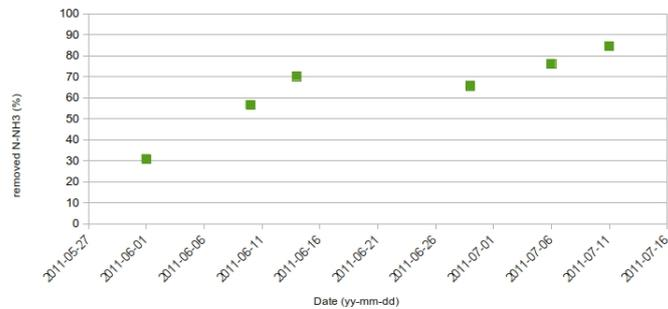
Figure 4.14: Ammonia removal efficiency in R1 during second run
