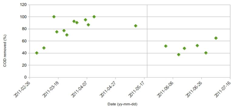
Figure 4.4: COD removal efficiency in R2
