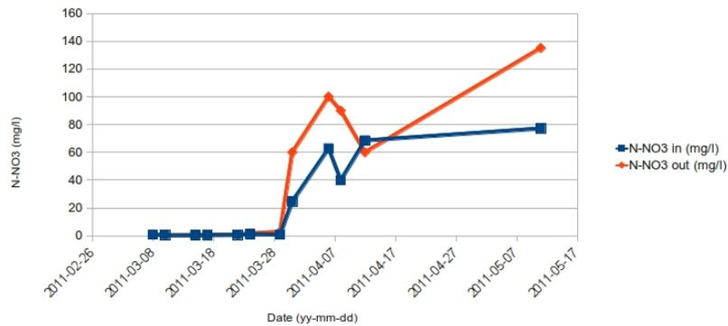
Figure 4.10: Influent and effluent nitrate concentration in R1
