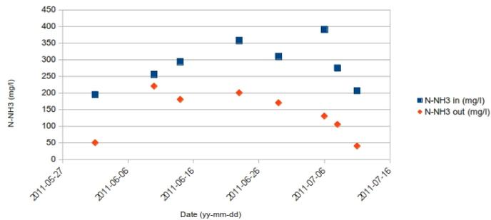
Figure 4.22: Influent vs effluent ammoniacal nitrogen during second run
