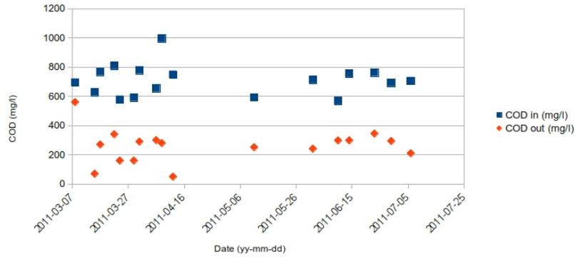
Figure 4.8: Influent and effluent COD in R3
