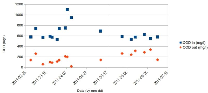
Figure 4.6: Influent and effluent COD in R1
