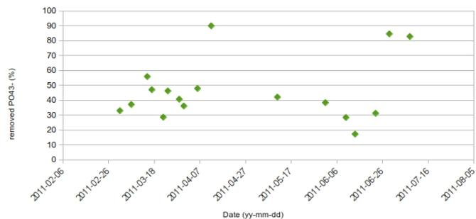
Figure 4.33: Phosphate removal efficiency in R3
