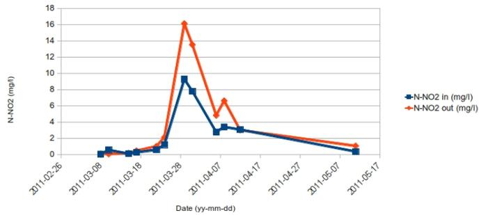
Figure 4.21: Influent and effluent nitrite in R2
