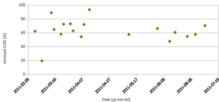
Figure 4.5: COD removal efficiency in R3
