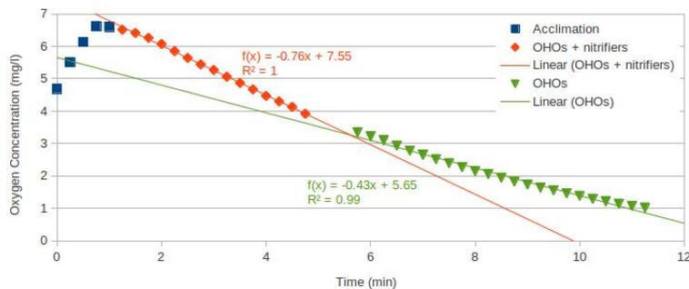
Figure 4.39: OUR test with 30 ml of settled granules for R2
