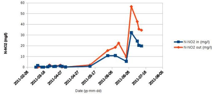
Figure 4.29: Influent and effluent nitrite in R3
