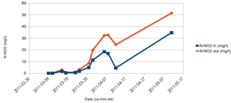
Figure 4.11: Influent and effluent nitrite concentration in R1
