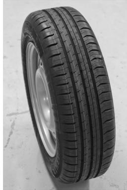
**Fig. 5.3.** The 175/65R 14T XL tyre modelled in this thesis.
