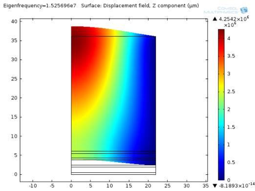
Figure 4.3: Circular cMUT with protective FPC coating,  $f_0 = 15.2 \text{ MHz}$
