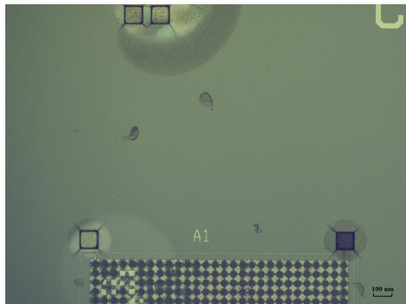
Figure 3.9: Cracks and delamination of SU8 after development
