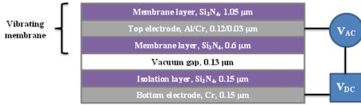
Figure 4.1: Test cMUT verification model
