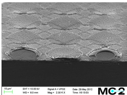
Figure 3.10: SEM picture of the cMUT array
