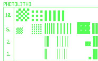
Figure 3.4: “Photolitho” pattern for the resolution check
