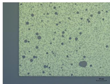
Figure 3.8: Etched Al layer due to micropores in PECVD SiO<sub>2</sub>
