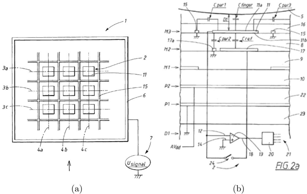
Figure 2.4: Capacitive fingerprint sensor design: a) top view, b) side view (with permission from Fingerprint Cards AB)
