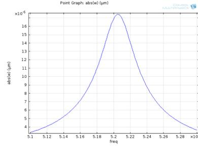
Figure 4.6: Frequency analysis of test structure,  $Q_{air} = 180$
