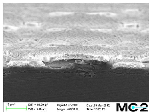
Figure 3.11: SEM picture of the cMUT membrane
