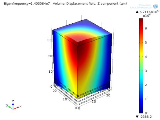
Figure 4.4: Square cMUT with protective FPC coating,  $f_0 = 14 \text{ MHz}$
