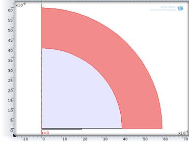
Figure 4.5: Geometry of test structure and Perfectly Matched Layer (PML)
