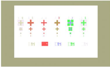
Figure 3.3: Fine alignment marks in the framebox
