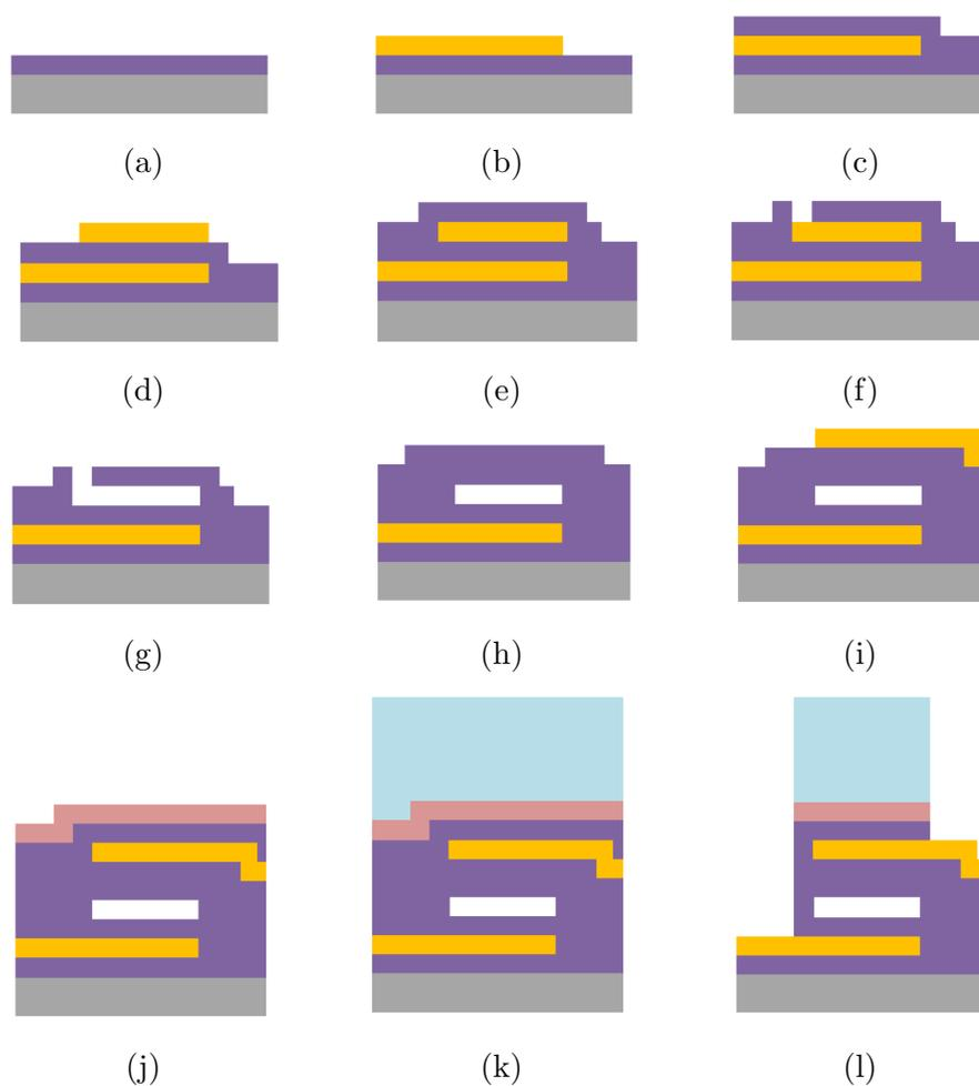
Figure 3.6: Schematic fabrication process plan of cMUT
