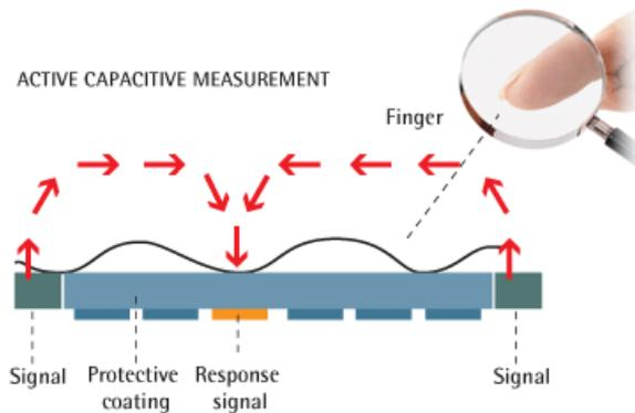
Figure 2.3: Capacitive fingerprint sensing method (with permission from Fingerprint Cards AB)
