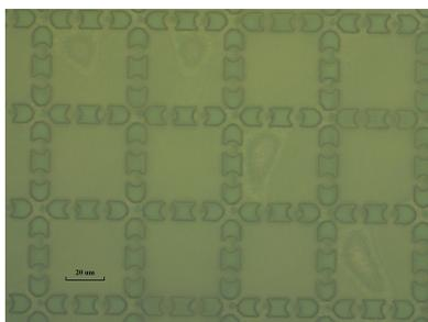
Figure 3.7: Collapsed membranes recognized by optical rings
