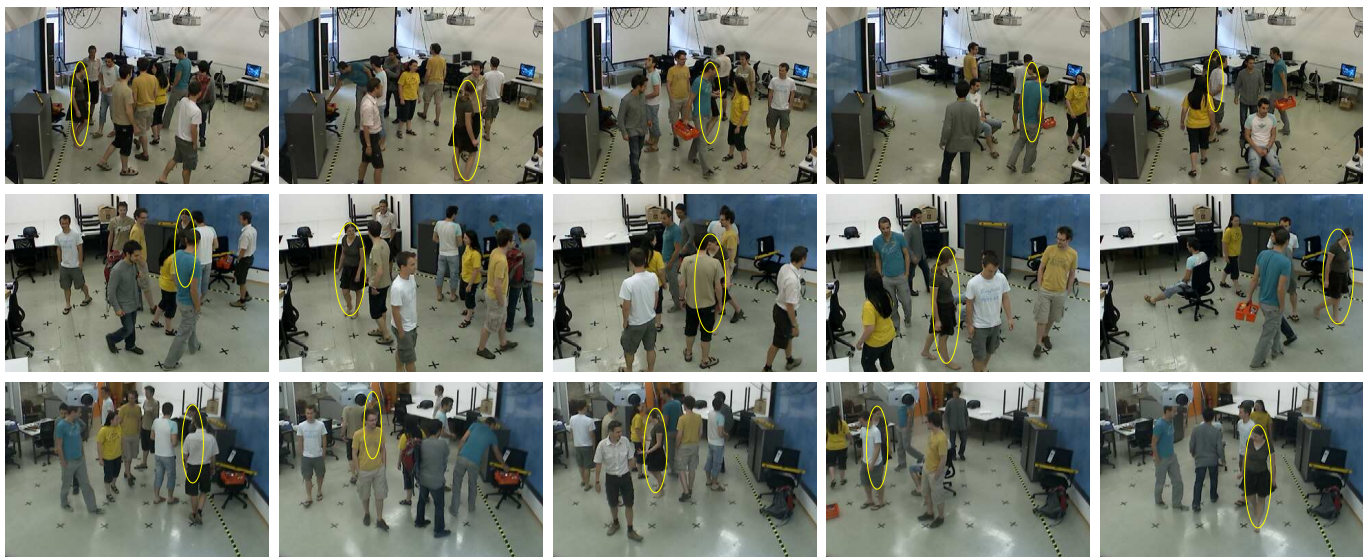
Fig. 8. Results of three-view tracking for an object experiencing frequent intersections. Row 1-3: results from proposed multi-view ML tracking (yellow ellipse) for the 1st, 2nd and 3rd view, respectively. Frames are: # 3201, 3272, 3369, 3702, 3835. Multi-view videos are from Hard scenario Set 1 of TU Graz Multi-Camera datasets.
