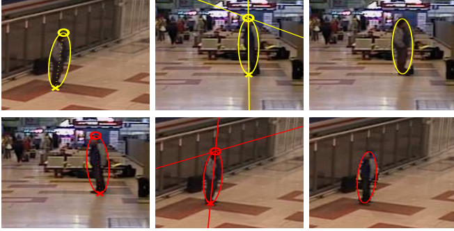
Fig. 4. Mapping estimated position and object appearance between a pair of views, using warped vertical axis. For each row, Column 1: detected vertical axis (dotted line) and tracked region in one view. 'o' and 'x': top and ground points of object. Column 2: warped vertical axis in each destination view, where the vertical line passes through the warped axis, the inclined line is epipolar line associated with object top point from the other view in Column 1. Column 3: mapped object appearance in each destination view.
