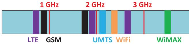
Fig. 1.2: Spectral position of the main communication standards.
