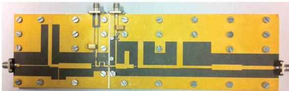
**Fig. 4.10:** Photo of the realized dual-band Main PA.
