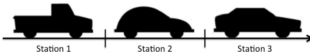
Figure 7. Example of the principle of a mixed model assembly line
