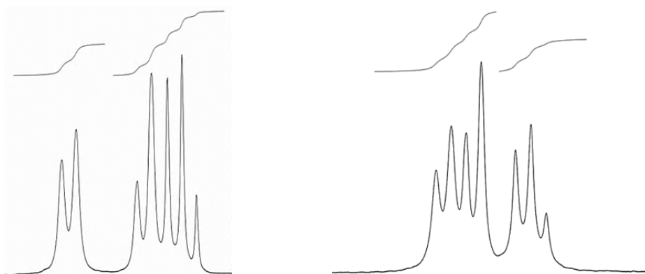
Figure 5.3.5 ^1\text{H} NMR spectra of solid complexes of Ag and CyMe 4 -BTBP (left) and Ag and C2-BTBP (right) dissolved in cyclohexanone with an addition of C 6 D 6 (approximately 7.5%)
