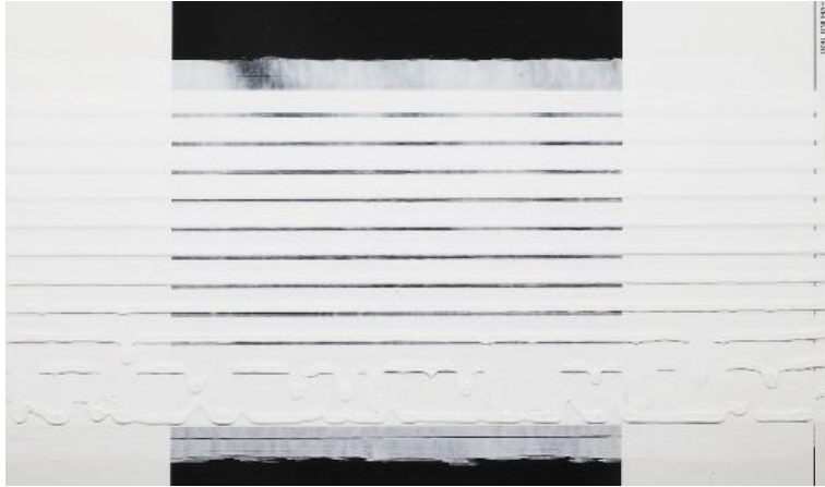
Figure 10: Illustration of a sagging test.
