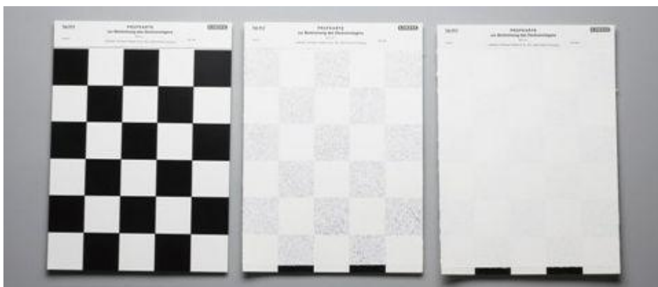
Figure 11: Illustration of a hiding power test.
