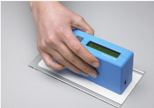
Figure 7: Illustration of gloss measurement.
