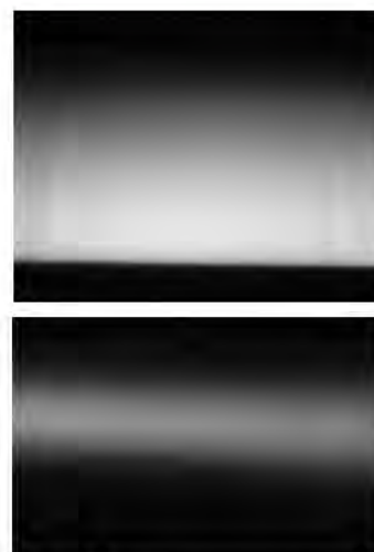
Figure 4.4 (TOP) Linear gradient formed by using 100%, 50% and 0% of fluorescence solution in inlet 1 to 3. (Bottom) Parabolic gradient formed by using 0%, 100% and 0% in inlet 1 to 3.
