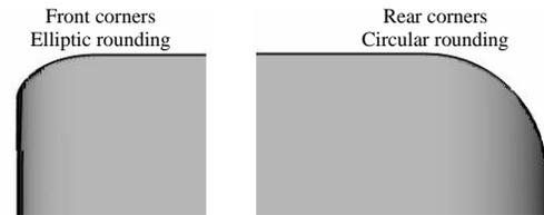
**Figure 2. The front and rear corners of the train model, respectively.**
