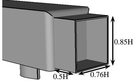
**Figure 3. The flaps attached on the base of the train model.**
