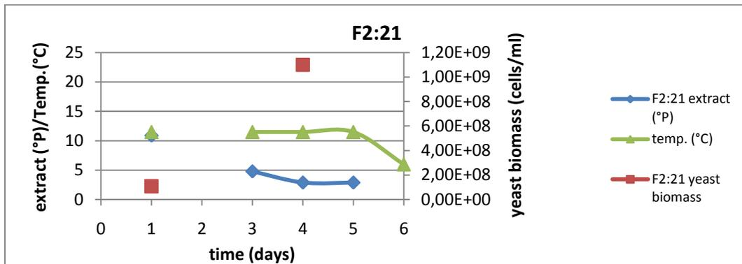
Figure 4.5 Yeast count, extract and temperature during 1<sup>st</sup> round of propagation in second yeast batch.
