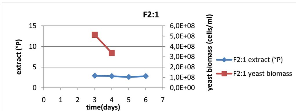
Figure 4.1 Yeast biomass and extract during 1<sup>st</sup> round of propagation from first yeast batch.
