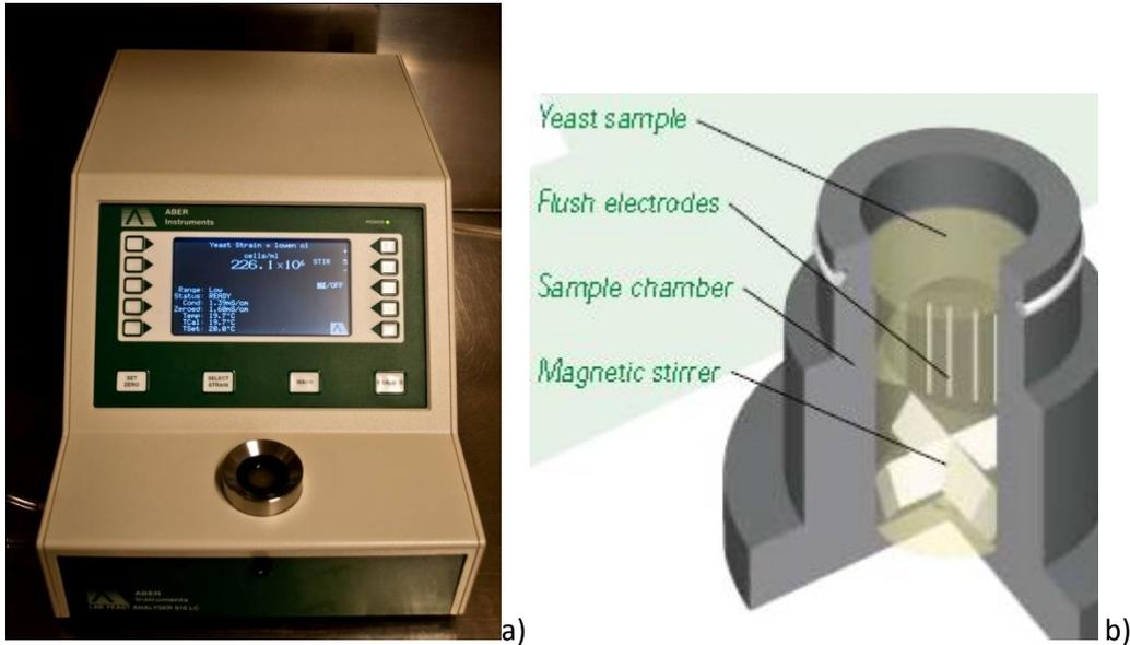
**Figure 2.5** ABER Lab Yeast Analyser (a) (Martin Marais, 2010. [Photograph]); Schematic illustration of the sample chamber of Lab Yeast Analyser (b) (Aber Instruments, 2010).
