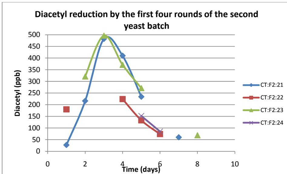
**Figure 4.13** Diacetyl reductions during fermentations by the second batch of propagated yeast.
