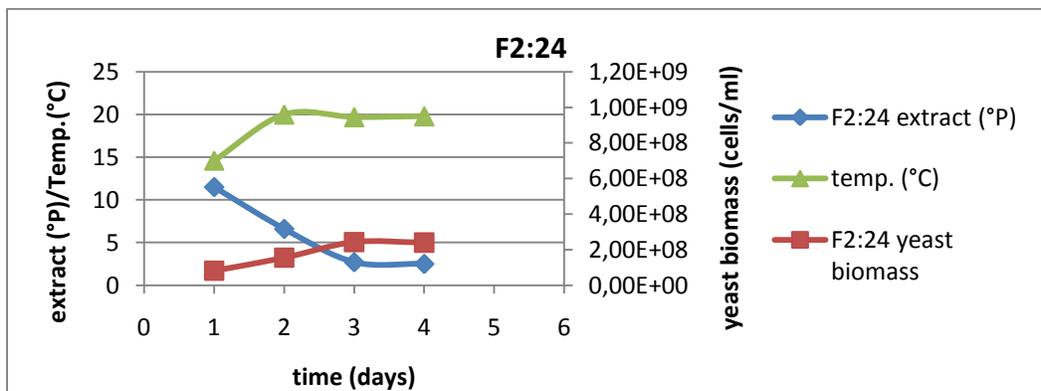
Figure 4.8 Yeast count, extract and temperature during 4<sup>th</sup> round of propagation in second yeast batch.
