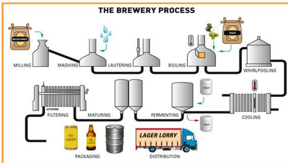
Figure 2.1 Simplified diagram of the in- process production of beer (IBD, 2010).
