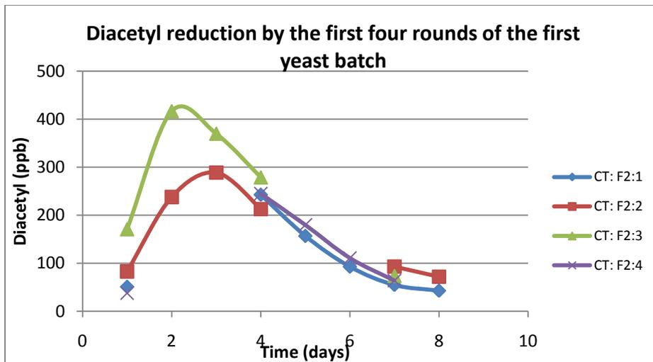
**Figure 4.12** Diacetyl reductions during fermentations by the first batch of propagated yeast.
