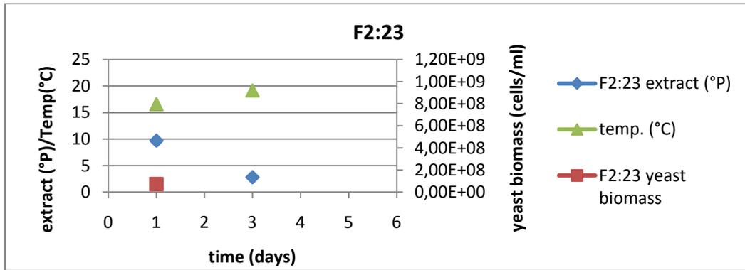
Figure 4.7 Yeast count, extract and temperature during 3<sup>rd</sup> round of propagation in second yeast batch.
