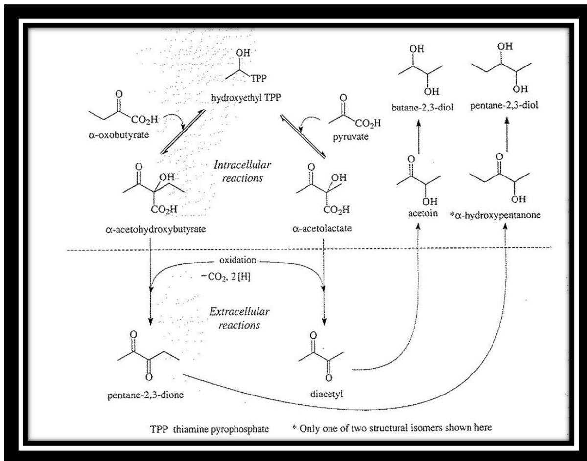
**Figure 2.8** Pathway of diacetyl formation from leaked out  $\alpha$ -acetolactate (Hughes, 2001).
