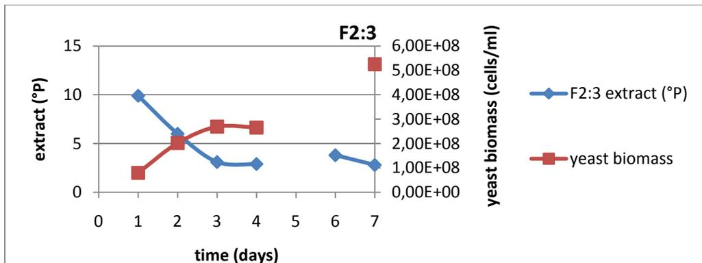
**Figure 4.3** Yeast biomass and extract during 3<sup>rd</sup> round of propagation from first yeast batch.
