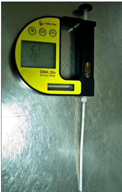
**Figure 2.4** Extract measurement device called density meter (Martin Marais, 2010 [Photograph]).
