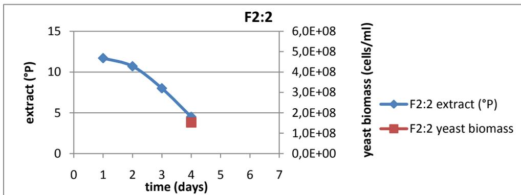
**Figure 4.2** Yeast biomass and extract during 2<sup>nd</sup> round of propagation from first yeast batch.
