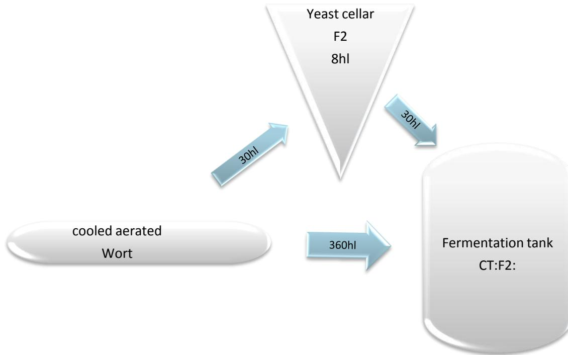
**Figure 2.3** Schematic illustration showing the procedure of each round of propagation at Spendrups brewery.
