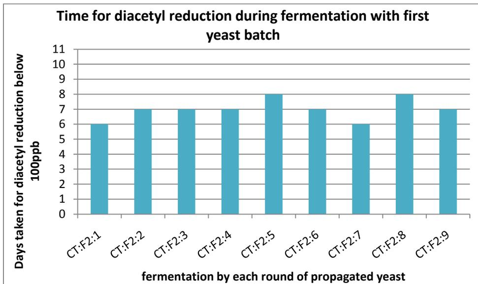
**Figure 4.10** Time taken for diacetyl reduction below 100ppb by rounds of propagation of the first yeast batch.
