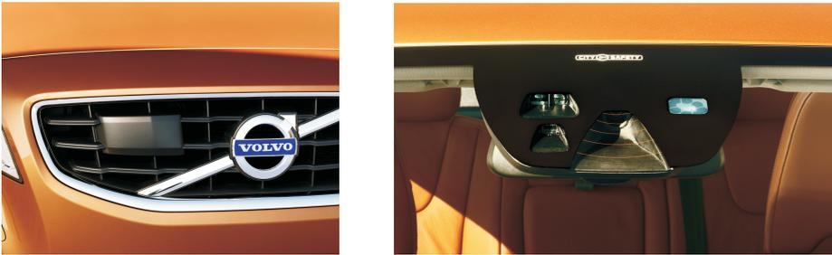
Figure 3.2: Example of how radar, lidar and camera sensors providing information of the surrounding environment can be mounted in a passenger vehicle. These sensors complement each other well, the advantages of the radar are typically the disadvantages of the camera and vice versa [14].
