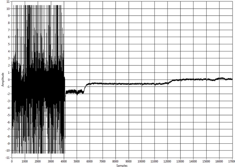
Figure 37: Here it is clearly visible that the high frequent noise is removed when the low pas filter is used.
