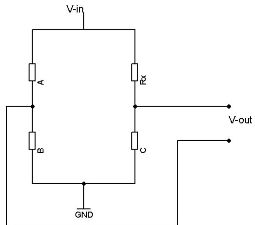
Figure 4: Quarter Bridge where the element  $R_x$  is the sensor
