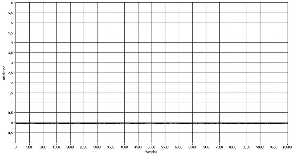
Figure 30: Signal post Decoupling stage (Passive high pass filter). Here the static DC signal is removed and only the AC-component remains.
