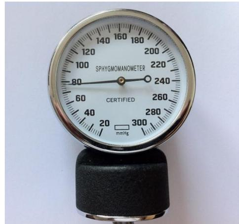
Figure 40: A manometer used to measure pressure.
