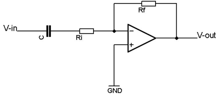
Figure 14: Inverting Active High Pass Filter
