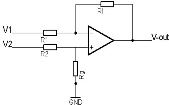
Figure 8: Schematic image of a differential amplifier where the voltage difference between the two signals is amplified.
