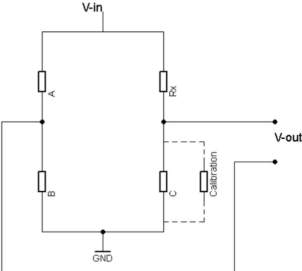
Figure 39: Circuit showing how the shunt calibration should be performed
