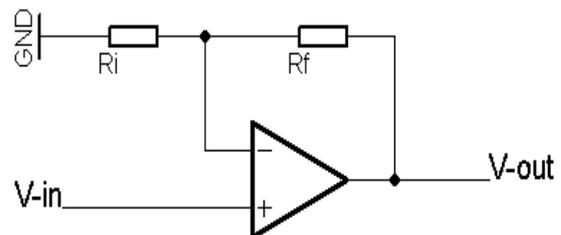
Figure 7: The amplification in a non-inverting amplifier is determined by the quotient of  $R_f$  and  $R_i$
