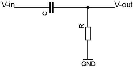
Figure 12: Passive High Pass Filter
