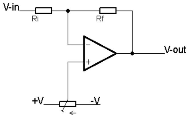
Figure 33: Levelshift circuit where the signal that is to be shifted is  $V_{in}$
