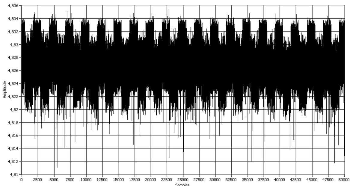
**Figure 18: The USB supply voltage when using computer 1. The Peak to Peak level of the noise is approximately 34mV**
