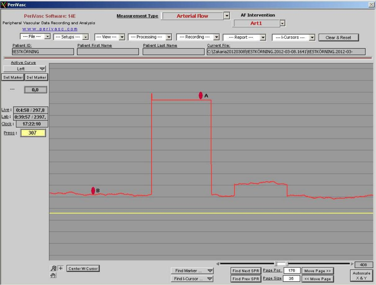
Figure 54: Here the higher peak corresponds to 1% strain (or increase of length) and the lower peak corresponds to a strain of 0.1%
