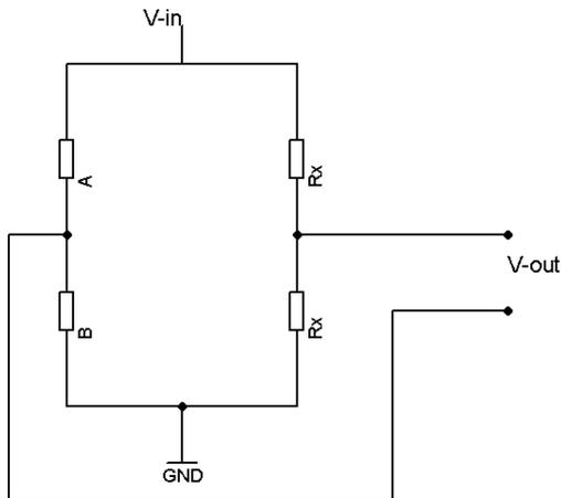
Figure 5: Schematic image of a half bridge. Where  $R_x$  is the sensor element, as seen there are two sensor elements.
