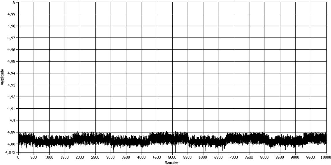
Figure 19: Voltage signal from the USB-drive of computer 1
