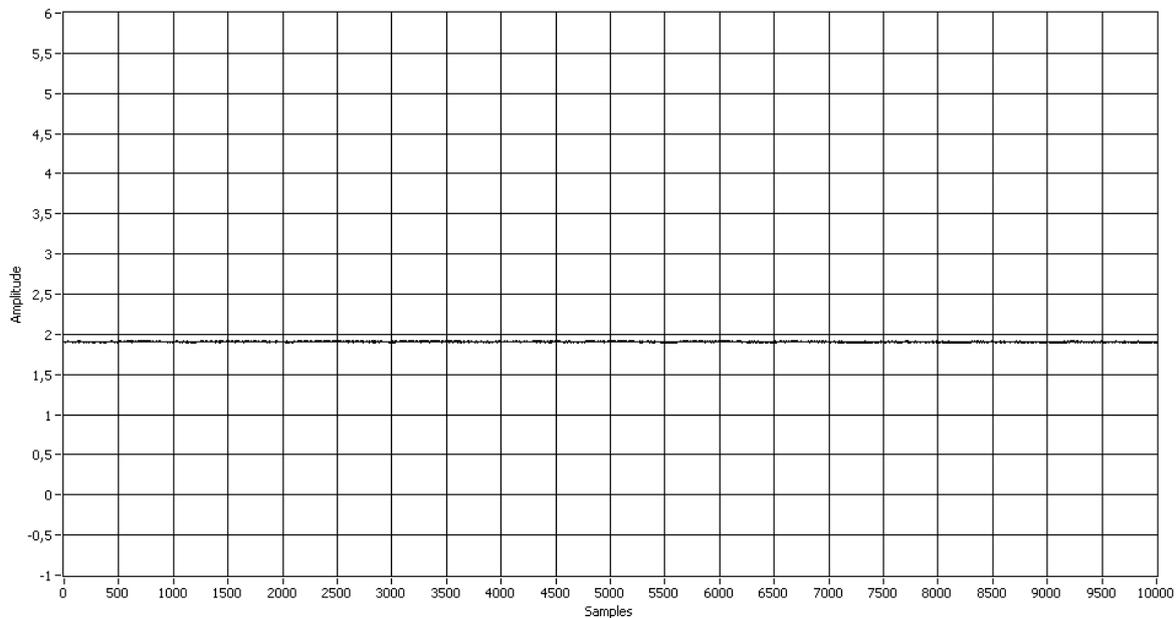
Figure 29: Signal prior to Decoupling stage (Passive high pass filter), The signal is over riding a static DC voltage with an amplitude of 2V.
