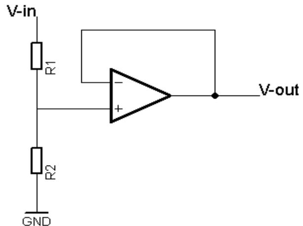
Figure 24: Voltage follower cascaded to a voltage divider
