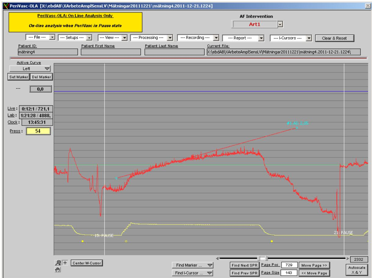
Figure 56: The result from a normal measurement on a forearm with the perimeter of 30.9 centimetres. The red curve is the signal from the strain gage and the yellow is from the blood pressure sensor. This person has a flow of 2.05[(ml/minute)/100 ml tissue] during rest.
