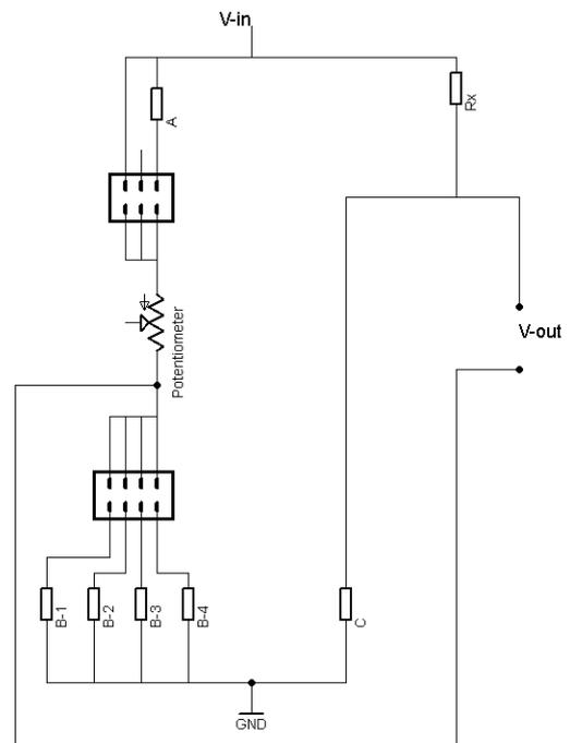
Figure 38: Schematic image of the bridge balancing circuit.
