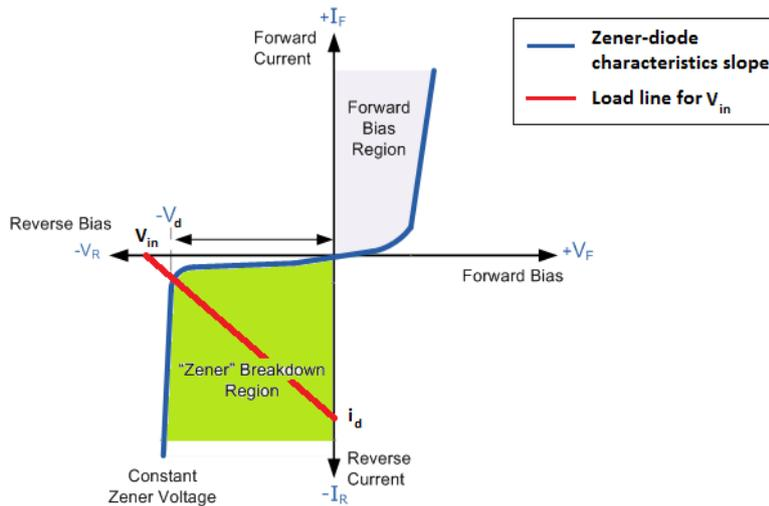
Figure 23: Load characteristics of a voltage regulator. (Source: (Hambley A. R., 2000))
