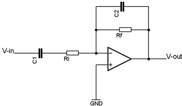
Figure 15: Inverting Active Band Pass Filter
