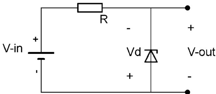
Figure 22: A schematic image of a voltage regulator. The voltage can be regulated by using components with different characteristics.
