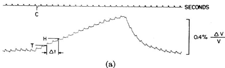
Figure 3: Signals from blood flow measurements done with strain gage. (Source: (Hokanson, Summer, & Strandness, 1972))
