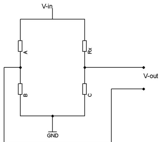
Figure 4: Quarter Bridge where the element  $R_x$  is the sensor
