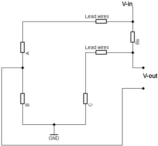
Figure 35: Circuit of Four-terminal sensing connection implementation using a Wheatstone quarter bridge
