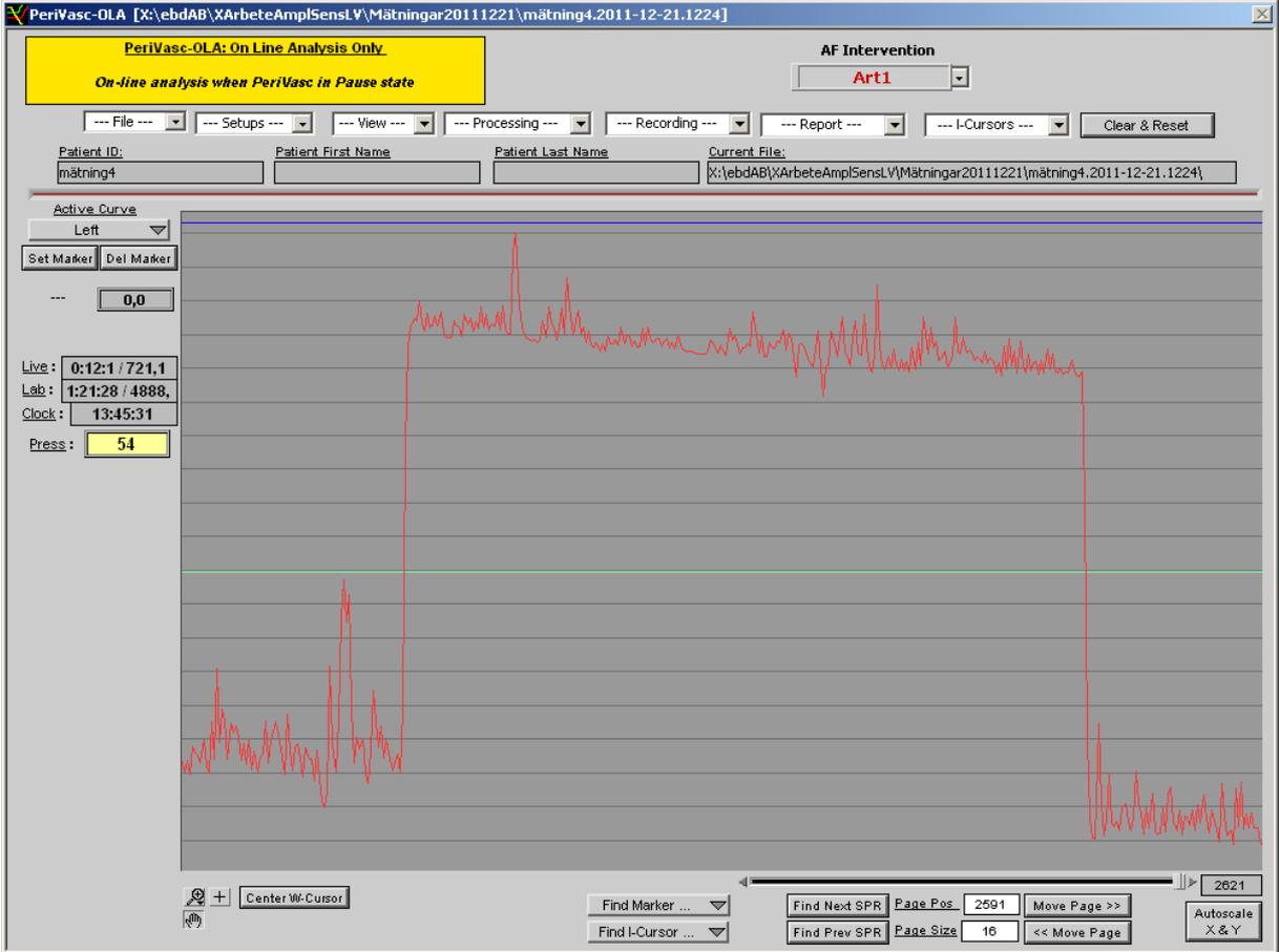
Figure 53: The electric calibration curve that corresponds to a strain of a 1 % increase of the original length of the strain gage.
