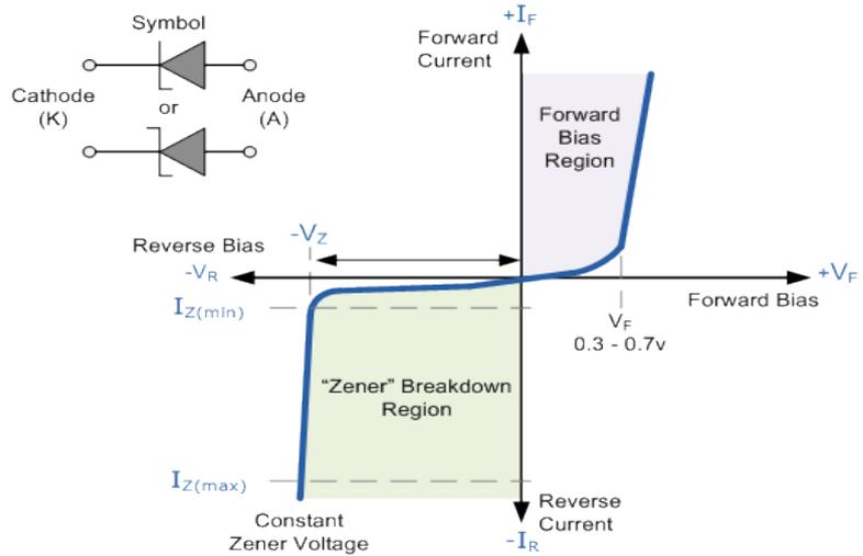
Figure 21: Characteristics of a zener diode. (Source: (Storr, 2011))
