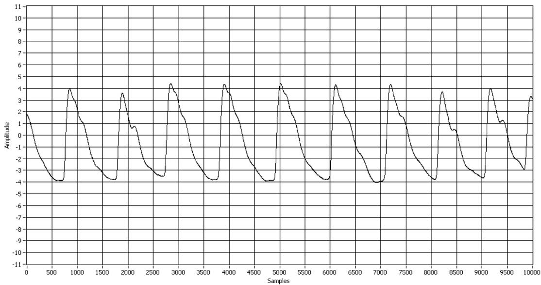
**Figure 34: Result of amplification due to level shifting, the signal is also shifted by the user so that the base line is at -4 Volts instead of 0 Volt.**
