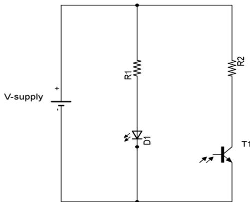
Figure 1: Schematic showing how the diode and transistors are connected in order to form a photo-cell sensor.
