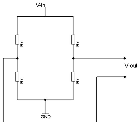
Figure 6: Schematic image of a full bridge configuration. Here  $R_x$  are sensor elements and as seen all elements are sensors.
