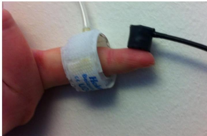
Figure 46: Placement of cuff and photo-cell sensor on finger.
