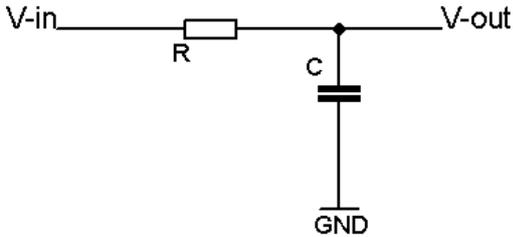
Figure 11: Passive Low Pass Filter.
