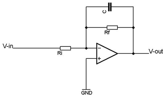
Figure 13: Inverting Active Low Pass Filter
