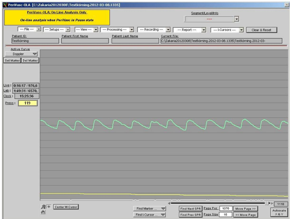
Figure 47: Readings from the prototype. The bottom curve is the cuff pressure and the one above is the signal from the photo-cell. Those curves that are left blank are not used for this evaluation. The pressure in the cuff when the pulses start to appear are 119 mmHg.
