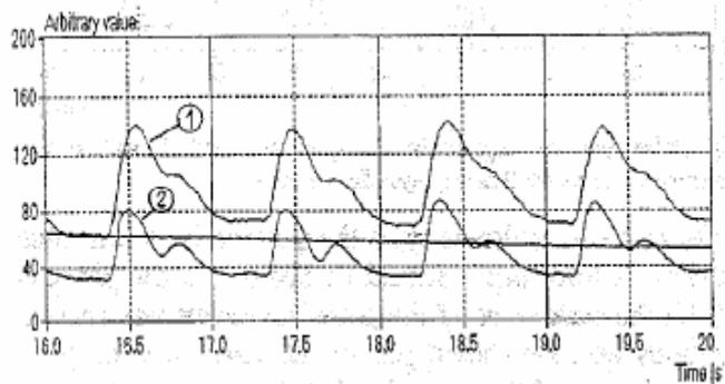
Figure 2: Typical shape of pulses when measuring with a photo-cell sensor. (source: (Wei))
