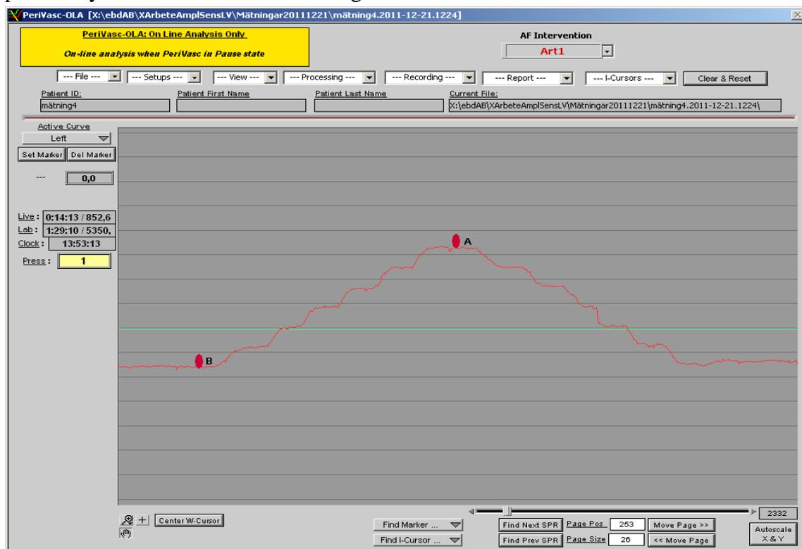
Figure 52: Calibration of strain gage using a millimetre screw, the screw is turned 6 times in one direction and then 6 turns in the other, in order to return to the baseline.
