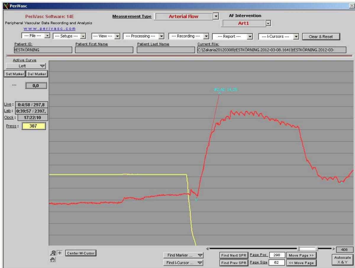
**Figure 57: Result from a measurement (on the same arm and person as above) using provocation to get a more distinct curve. To provoke the body the cuff was inflated until a pressure of 54 mmHg was reached, this pressure was then maintained for a few minutes and then slowly lowered. The flow is here calculated to 14.25[(ml/minute)/100 ml tissue].**
