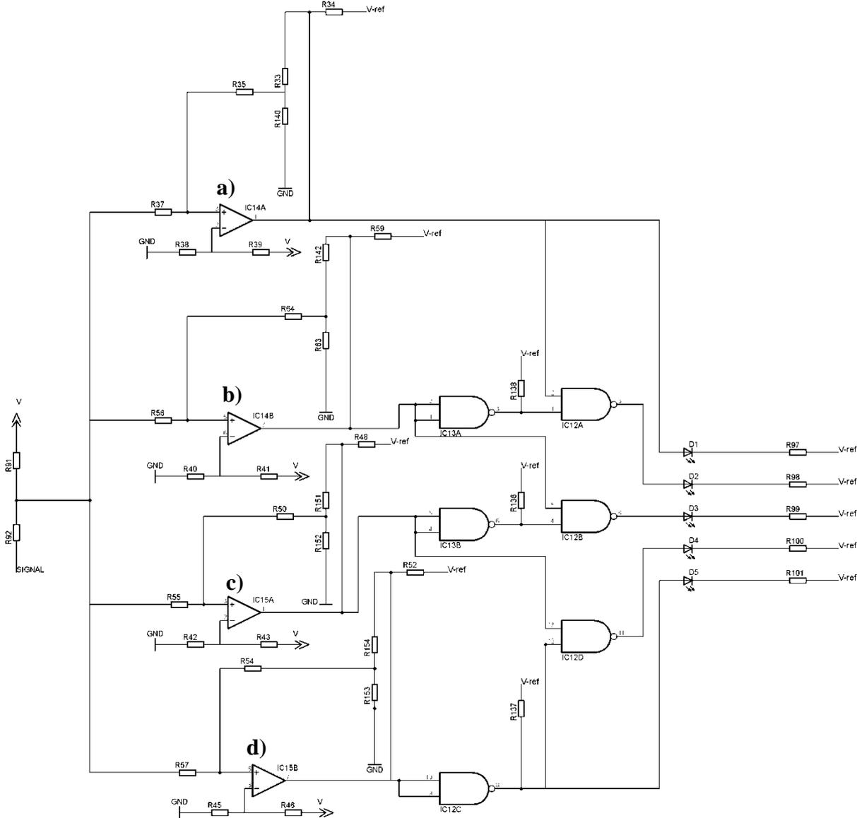
Figure 43: Schematic image of the comparators and logic circuit used for controlling the diodes. Here complete with signal scaling and pull-up resistors as well as hysteresis.
