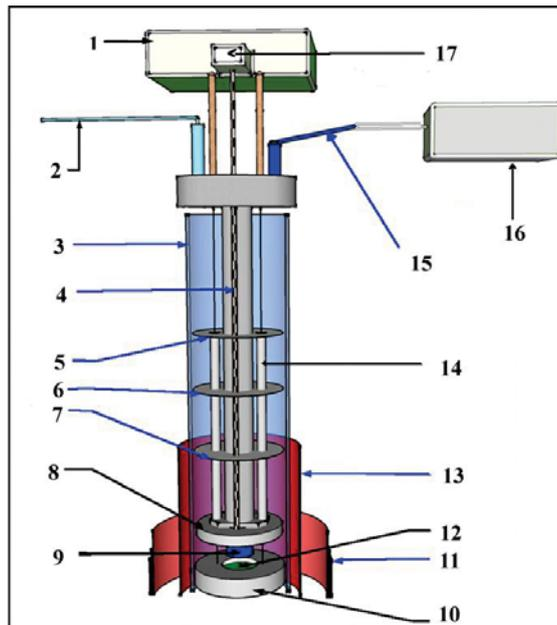
Figure 10: Schematics of the *in-situ* impedance spectroscopy cell. The components are named in table 2.
