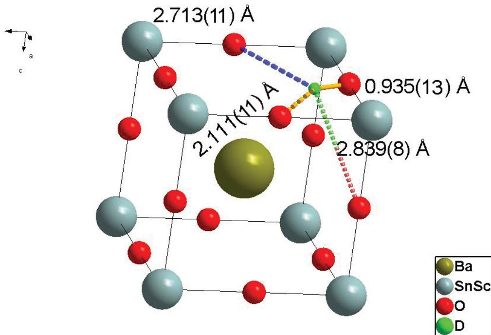
Figure 18: The unit cell of  $\text{BaSn}_{0.6}\text{Sc}_{0.4}\text{O}_{2.8}(\text{D}_2\text{O})_{0.2}$  showing bond arrangements, distances and the deuterium site at  $24k$  (0.584(2), 0.208(3), 0).
