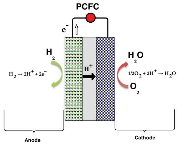
Figure 2: The schematics of a PCFC using hydrogen as a fuel and showing that H<sub>2</sub>O is produced at the cathode.
