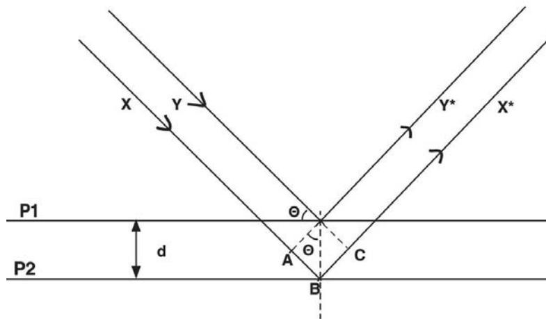
Figure 5: An illustration of the Bragg's law showing that the path length difference travelled by the second X-ray beam X, ABC can be calculated using  $2d\sin\theta$  where  $d$  is the interplanar distance,  $\theta$  is the incident angle, P is the plane and X and X' are the incident and diffracted beams respectively.
