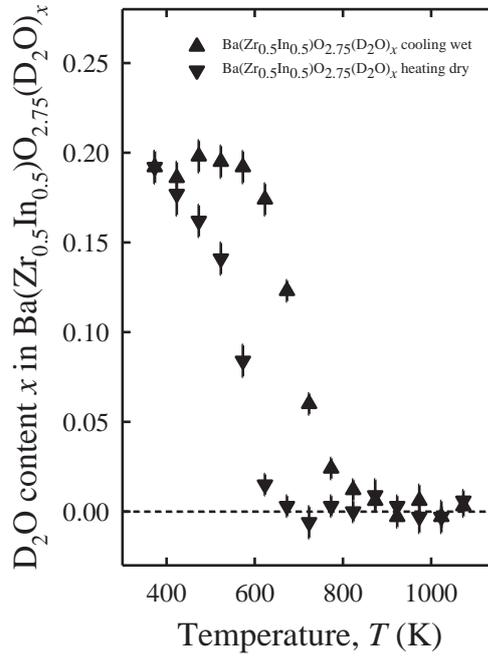
Figure 14: Variation of the refined D<sub>2</sub>O content as a function of temperature under dry Ar heating and under wet Ar on cooling.
