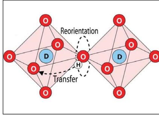
Figure 4: The Grotthuss mechanism for protonic transport in acceptor-doped perovskite. D is the dopant, O is Oxygen and H is the proton.
