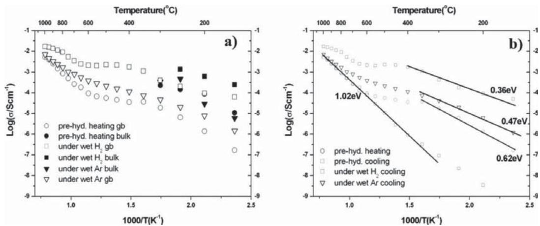
Figure 11: Conductivity of SPS BaZr<sub>0.5</sub>In<sub>0.5</sub>O<sub>3-δ</sub> sample under different atmospheres (a): bulk and grain boundary (gb) and (b): total.
