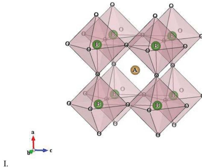
Figure 3: The structure of the cubic perovskite  $ABO_3$
