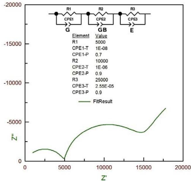
Figure 7: A simulated plot in the complex plane showing three semi-circles in the frequency range scan of interest. From the left, each semi-circle represents the grain bulk, grain boundary and the electrode responses. The insert shows the respective circuit models used for the plot.
