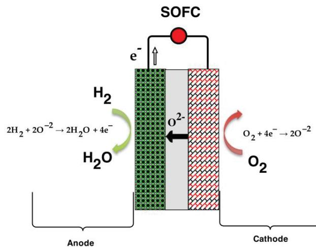
Figure 1: The schematics of a SOFC using hydrogen gas as the fuel.  $H_2O$  is produced on the Anode.
