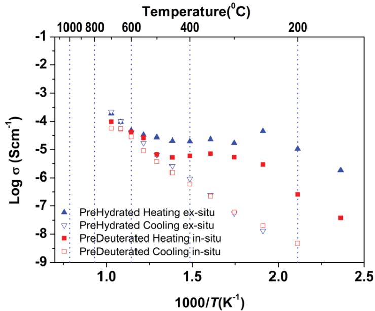
Figure 17: *In-situ* conductivity data of pre-deuterated sample compared to *ex-situ* pre-hydrated sample data collected by Ahmed *et al.*<sup>[47]</sup>.
