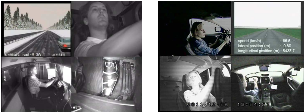
Figure 3.3: Left panel: A snapshot from the unexpected scenario in the ESC experiment, where a truck driver is forced to carry out rapid maneuvers on a slippery road. Right panel: A snapshot from the unexpected scenario in the eLKA experiment, where a car driver looks away from the road at the same time as a collision course with an oncoming car is established.
