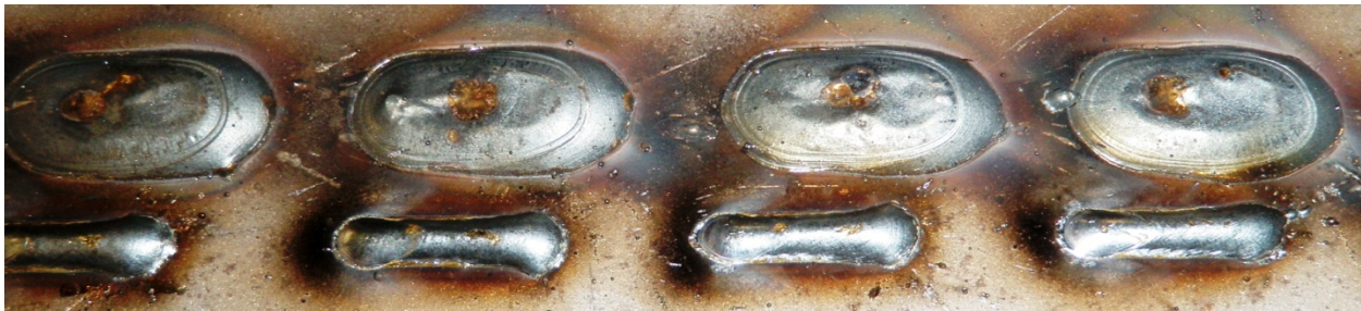
Figure 3.1 Sample Spray and Short Arc welding Tests
