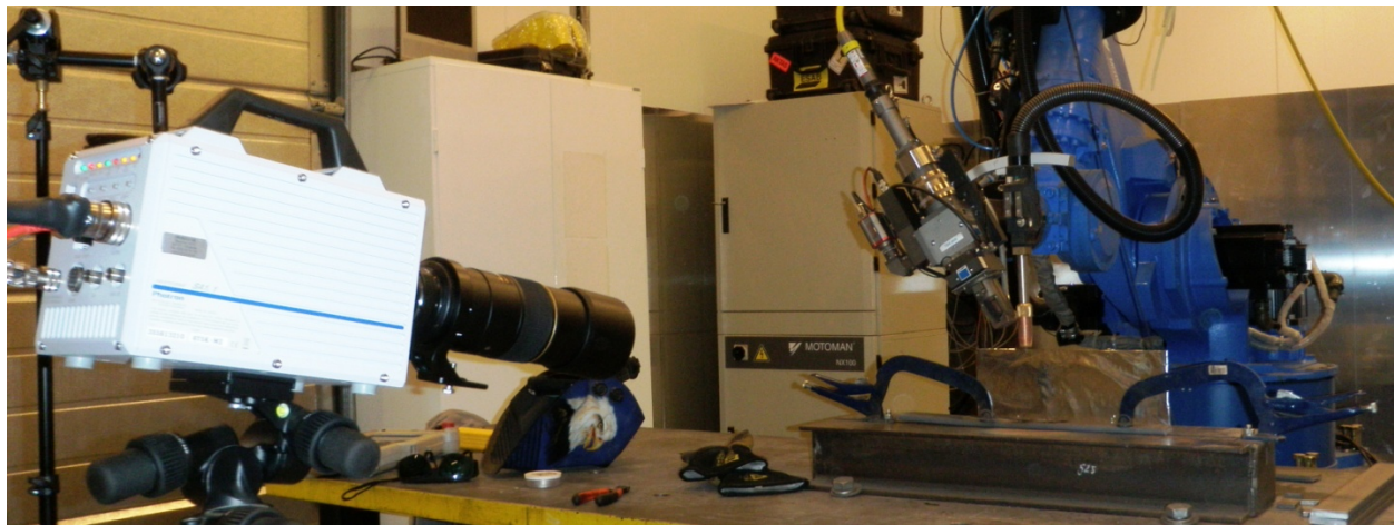
Figure 3.2 Welding Test Setting with High Speed Camera (left), Robot (right), table and work piece (middle)
