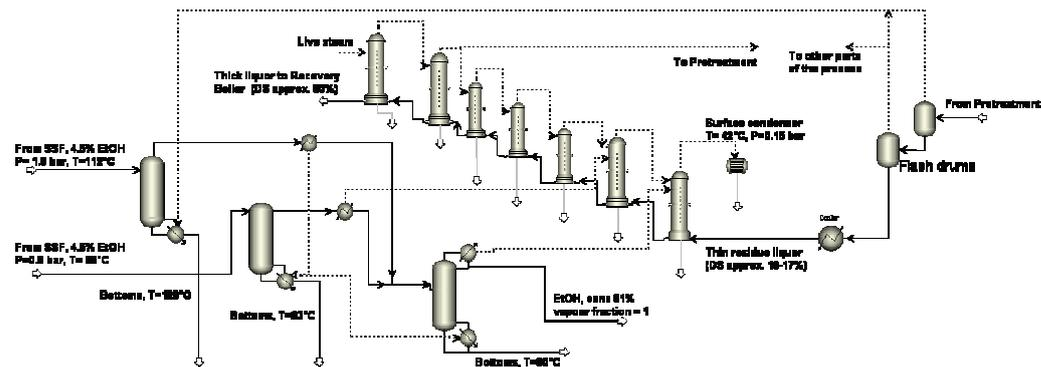
Figure 5.6. Distillation columns in parallel (upper), and stripper + rectifier (lower) sequence, integrated with other parts of the process (from Paper II).
