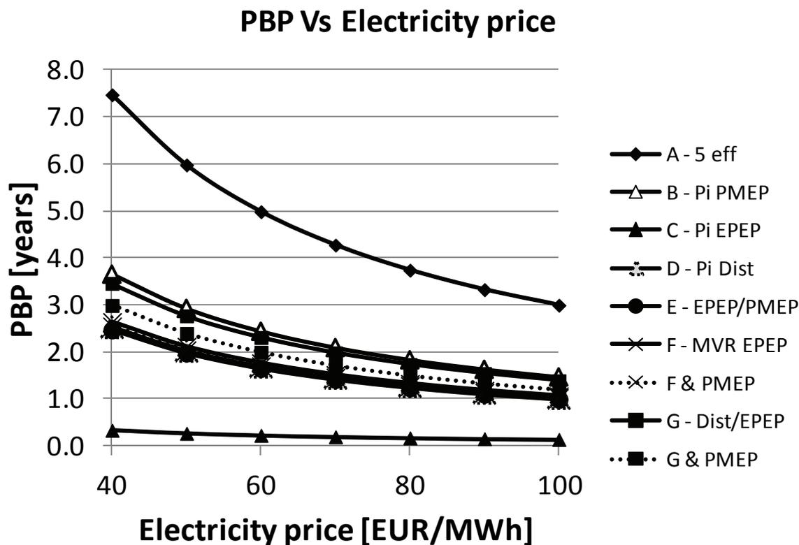
Figure 7.20. Sensitivity analysis of the payback period versus the electricity price for the alternatives in Table 2. EPEP = Ethanol Process Evaporation Plant, PMEP=Pulp Mill Evaporation Plant.
