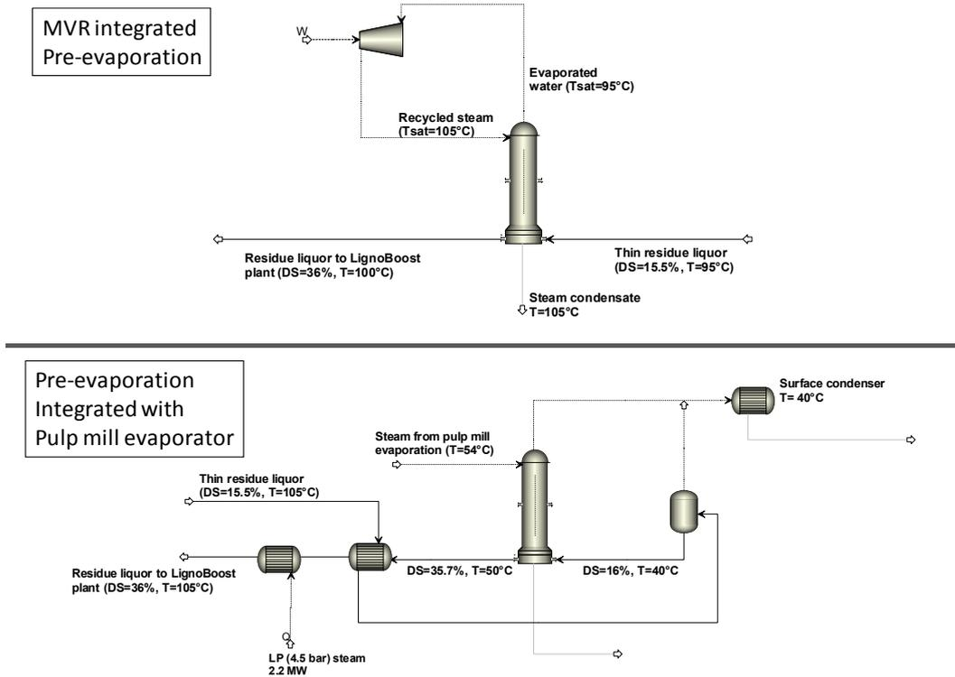
Figure 7.7. Ethanol process evaporation plant integrated with MVR-heat pump (upper) and pulp mill evaporation plant (lower).
