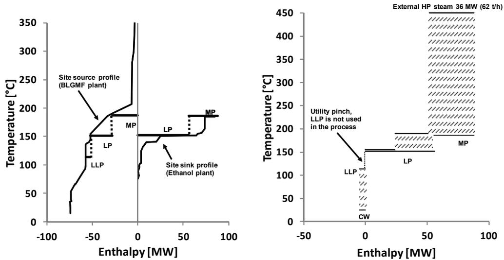
Figure 7.4. Site source and sink profiles and the resulting utility system for the combined ethanol and DME biorefinery.
