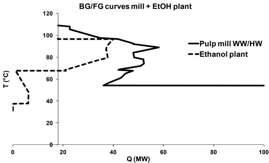
Figure 7.8. Split Grand Composite Curves indicating the potential for integration of the ethanol beer column and excess heat in the pulp mill secondary heating system.
