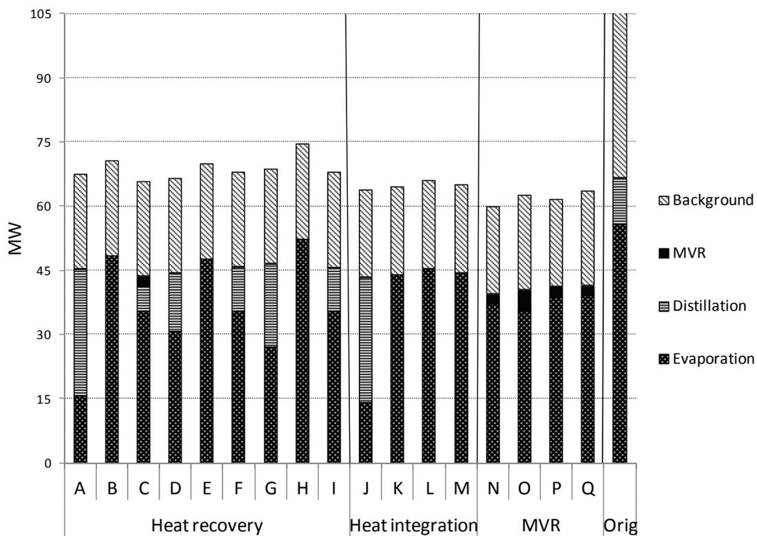
Figure 7.3. Steam demands in the studied process alternatives (based on data in Paper 2).
