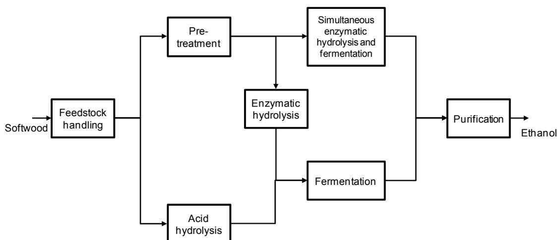
Figure 3.1. Block diagram of acid-or enzyme hydrolysed production of ethanol from lignocellulosic raw material (softwood).
