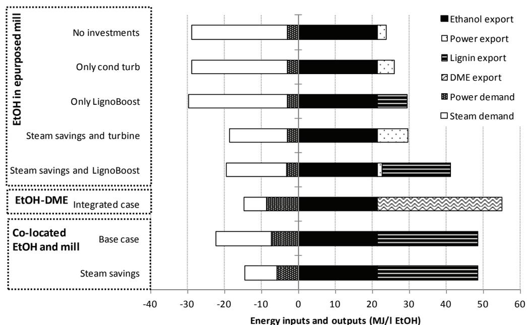
Figure 7.10. Utility demands (negative values) and energy allocation possibilities (positive values) in the different processes studied.
