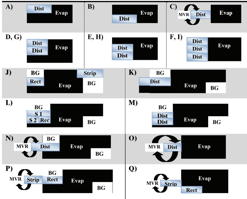
Figure 7.2. The different alternatives included in this work. BG stands for background process. Alternatives D-I are distillation columns (D-F) or stripper(s)/rectifier (G-I).
