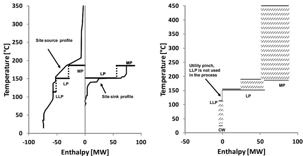
Figure 5.4. Composite curves depicting the site sink and source profiles (left) and the resulting site utility system (right).
