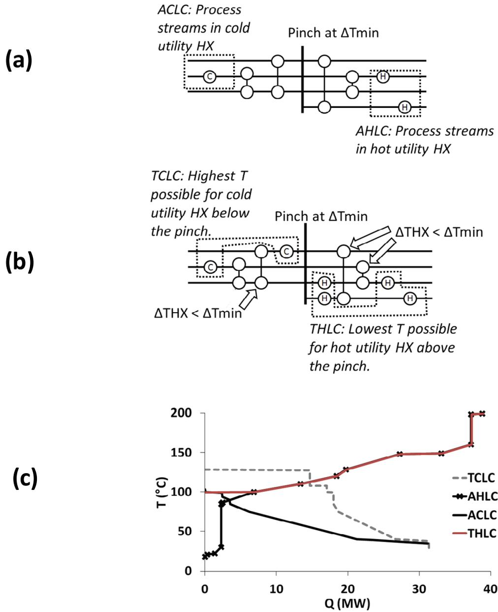
Figure 5.2. Actual heating and cooling loads (a), Theoretical heating and cooling loads (b), and advanced composite curves depicting these loads for the ethanol plant in Papers II and III (c).
