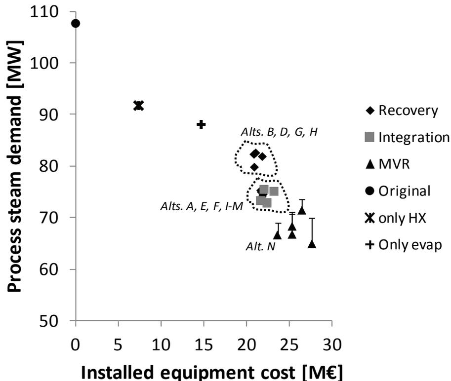
Figure 7.11. Installed equipment cost (distillation, evaporation and background process) vs. process steam demand for the studied alternatives in the repurposed pulp mill ethanol plant.
