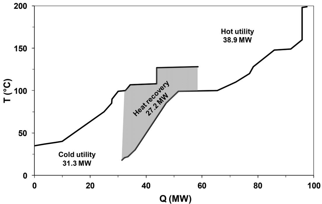
Figure 7.1. Composite Curves of the background process in the base case. The utility demand corresponds to a global  $\Delta T_{min}$  of 28.5 K.
