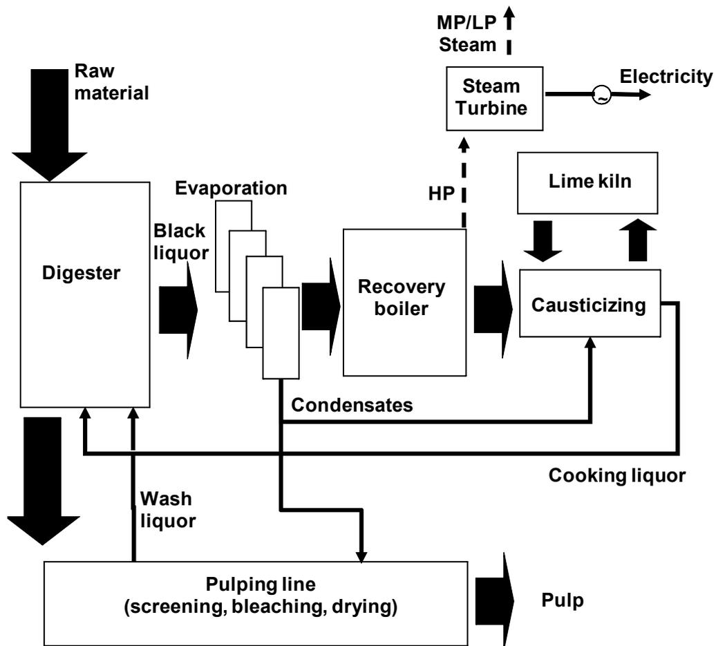
Figure 2.1. Block flow diagram of the Kraft pulp mill process.
