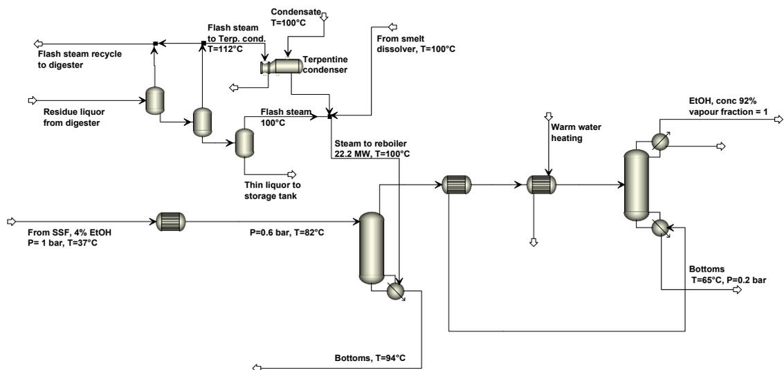
Figure 7.9. Process integration between excess heat from the pulp mill secondary heating system and the first column in the distillation sequence.
