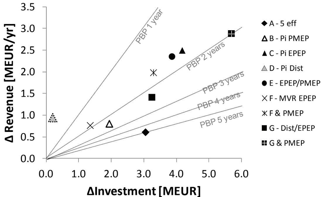
Figure 7.19. Results from the economic analysis at an annuity factor of 0.1 and an electricity price of 60 €/MWh. Pi = integration with pulp mill hw/ww system, EPEPE = Ethanol Process Evaporation Plant, PMEPE=Pulp Mill Evaporation Plant.
