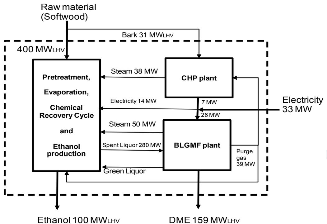
Figure 7.5. Energy flows in the ethanol + DME biorefinery.
