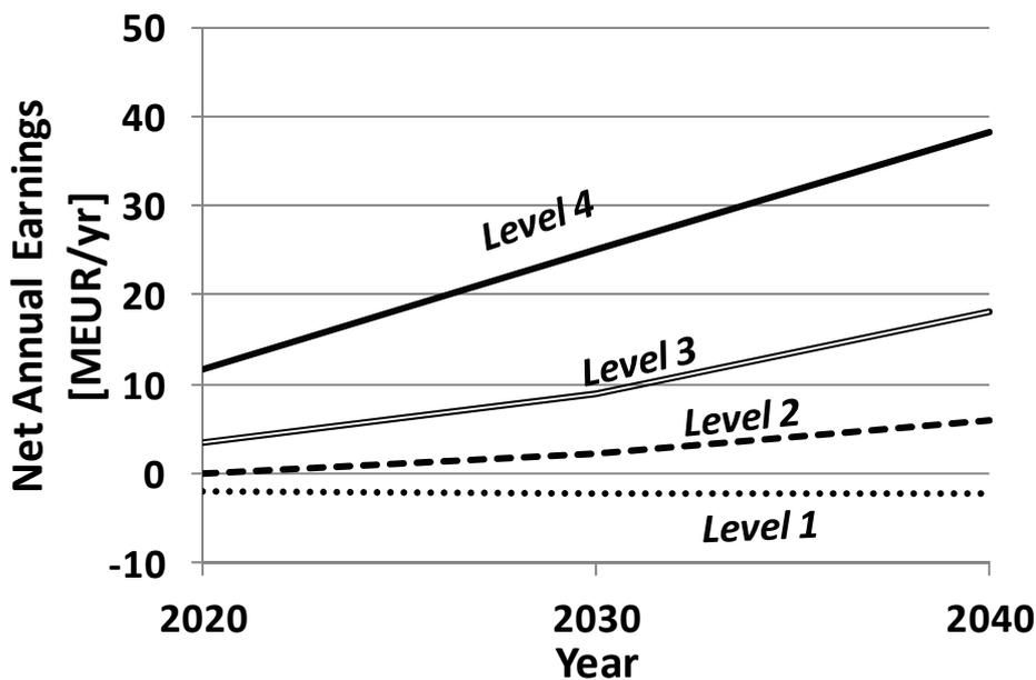
Figure 7.18. Net annual earnings when investing in a CCS plant for four different CO<sub>2</sub> charge levels.
