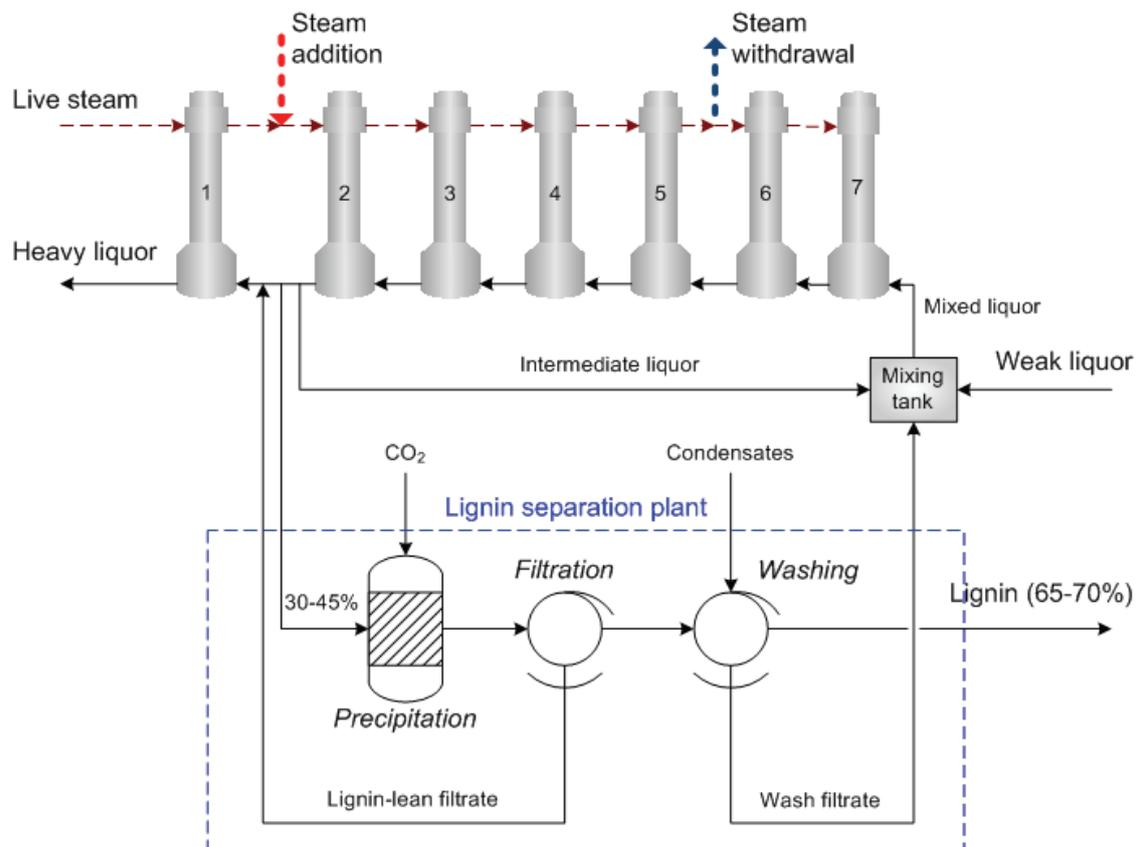
Figure 5.5. Evaporation plant with heat integration and lignin separation (which can be simulated in OptiVap).
