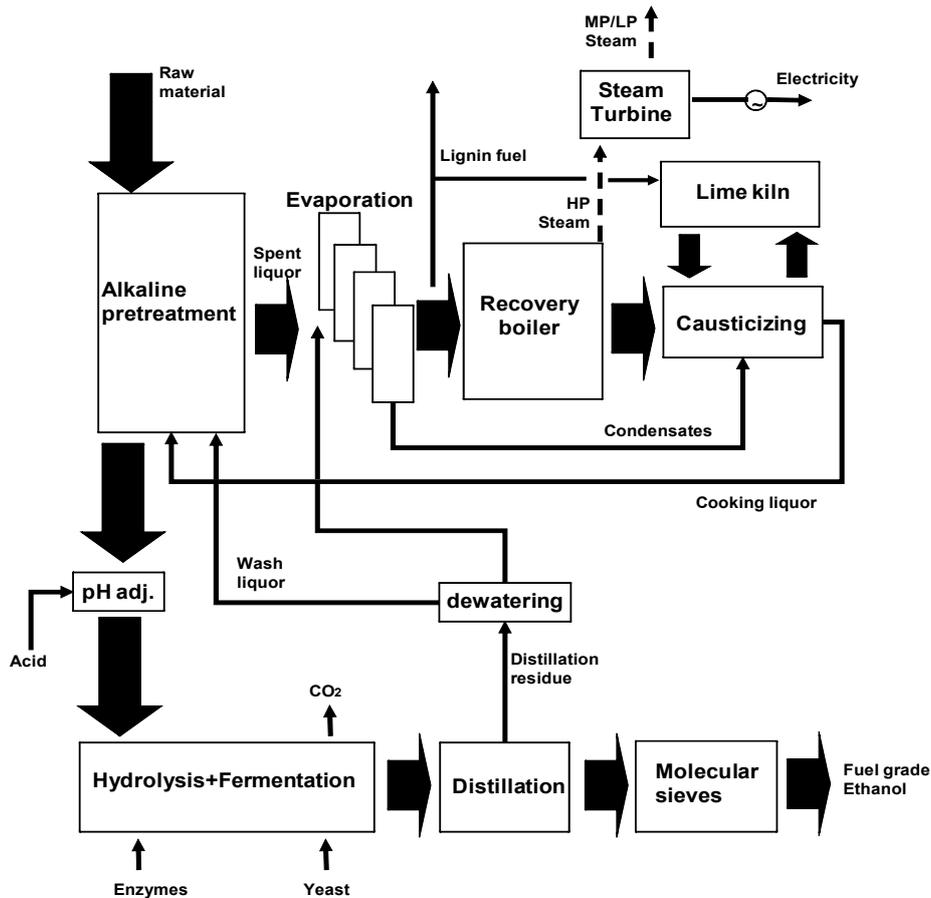
Figure 6.1. Block diagram of the conceptual ethanol production process.
