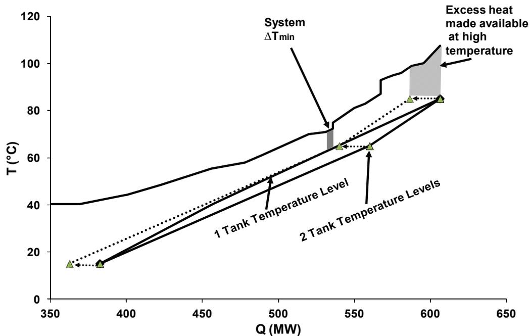
Figure 5.3. Tank curves with one and two tank temperature levels, indicating the excess heat made available for integration when increasing the number of tank temperature levels.
