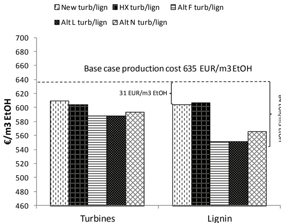
Figure 7.13. The ethanol production cost (Minimum selling price) for the evaluated design alternatives.
