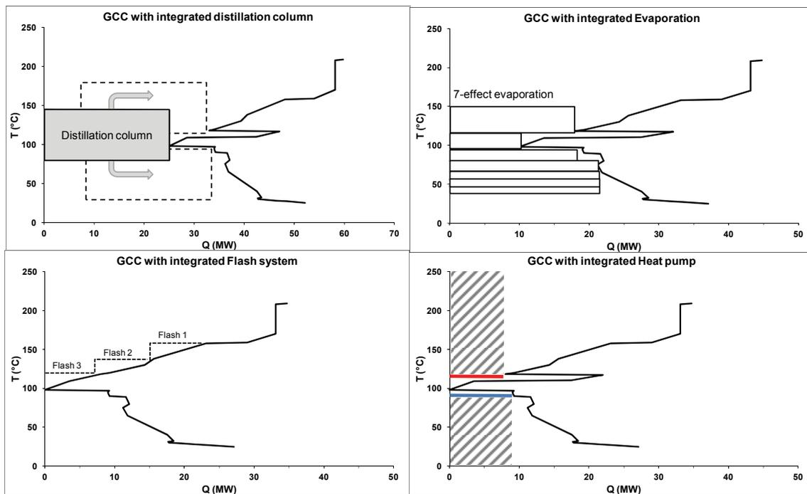
Figure 5.1. Examples of potential for integration by using split GCCs. Distillation column (upper left), evaporation plant (upper right), Flash system (lower left), and a heat pump (lower right).
