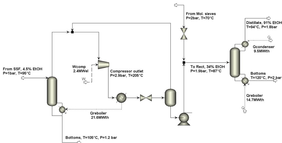
Figure 5.7. MVR-integrated distillation columns (from Paper III).
