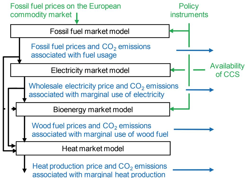
Figure 5.8. Overview of the calculation flow in the scenario model used in this project (courtesy of Axelsson and Harvey [96]). Green arrows represent required inputs, boxes represent calculation units, black arrows represent information flow within the model, and blue arrows indicate outputs from the tool.
