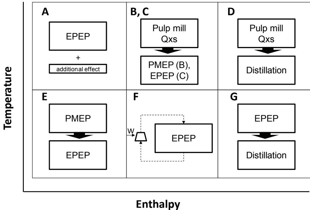
Figure 7.6. The different heat integration alternatives in the co-located ethanol plant and Kraft pulp mill. EPEP = Ethanol Process Evaporation Plant, PMEPE = Pulp Mill Evaporation Plant.
