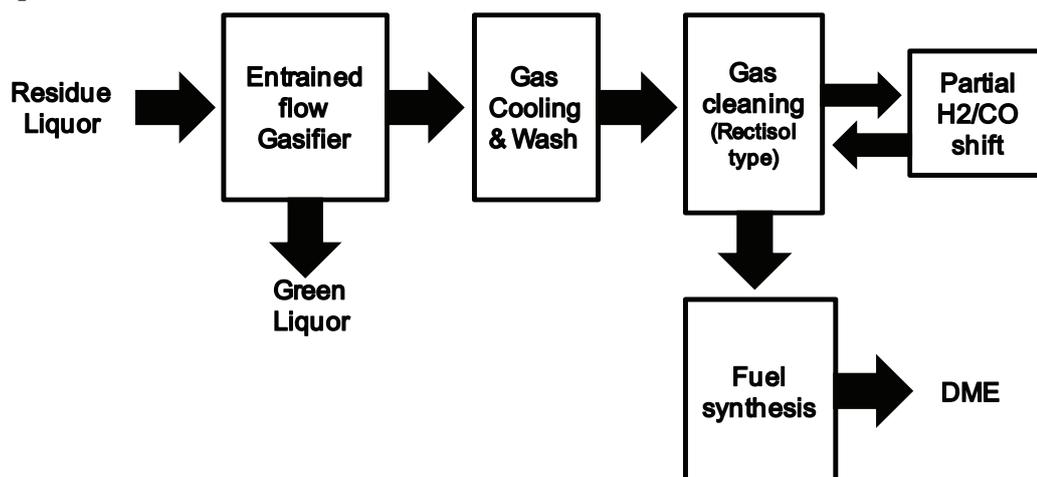
Figure 6.2. Block flow diagram of the black liquor gasification process for production of DME.
