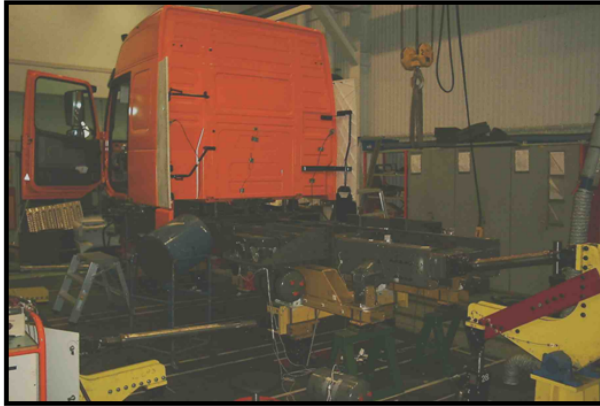
Figure 3.1: Example of TWR application in industry. Durability testing of truck cab at Volvo Group Trucks Technology testing facilities.
