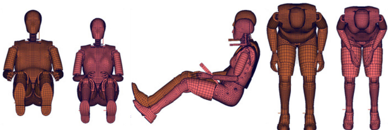
Figure 36. Comparison of the EvaRID V1.0 and the BioRID II models.
