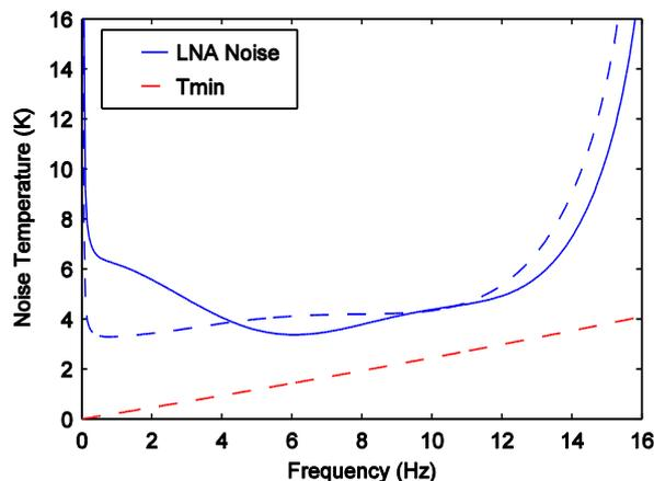
Fig. 4.1: Extracted  $T_{\min}$  of a  $2 \times 100 \mu\text{m}$  InP HEMT at 15 K (red dashed) compared with the simulated noise temperature of the amplifier connected to a  $50 \Omega$  source impedance (blue solid) and  $100 \Omega$  source impedance (blue dashed). The InP HEMT was biased at  $V_{\text{ds}} = 0.6 \text{ V}$ .
