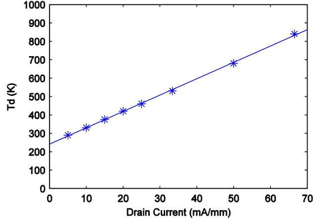
Fig. 3.12: Drain resistor temperature  $T_d$  extracted at different drain current densities from Fig. 3.11.  $V_d$  was 0.6 V for all extraction points and  $I_d$  was swept between 1 mA and 13.3 mA (5 mA/mm and 66.5 mA/mm) for each  $2 \times 100 \mu\text{m}$  InP HEMT.
