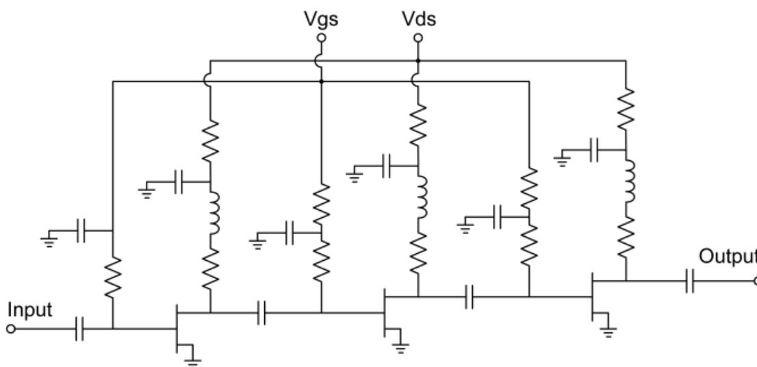
Fig. 4.2: Schematic of the 3-stage 0.5-13 GHz MMIC LNA.
