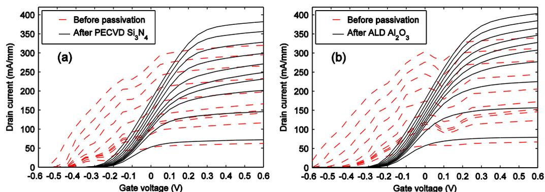
Fig. 2.4: Extrinsic transfer characteristics of  $2 \times 50 \mu\text{m}$  InP HEMTs before and after passivation with (a) PECVD  $\text{Si}_3\text{N}_4$  and (b) ALD  $\text{Al}_2\text{O}_3$ . Drain voltage was swept in steps of 0.1 V from 0.1 V (lower curve) to 1 V (upper curve).
