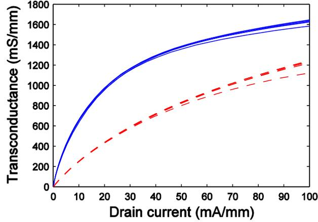
Fig. 3.7: Intrinsic  $g_m$  of a  $2 \times 100 \mu\text{m}$  gate width and 130-nm gate length InP HEMT at 300 K (red dashed) and 4 K (blue solid) ambient temperature.  $V_{ds}$  measured from 0.2 V (lower curve) to 1 V (upper curve) in steps of 0.2 V.
