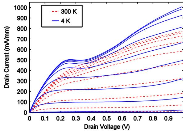
Fig. 3.2: Drain current of a  $2 \times 10 \mu\text{m}$  gate width and 130-nm gate length InP HEMT at 300 K (red dashed) and 4 K (blue solid) ambient temperature.  $V_{\text{gs}}$  measured from  $-0.3 \text{ V}$  to  $0.6 \text{ V}$  in steps of  $0.1 \text{ V}$ .
