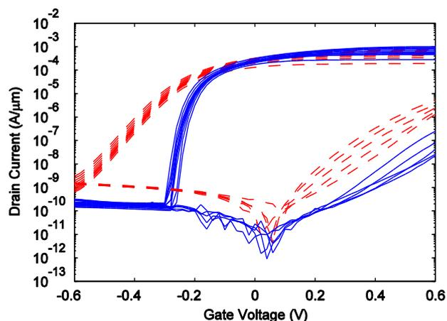
Fig. 3.6: Subthreshold and  $I_g$  characteristics of InP HEMT at 300 K (red dashed) and 4 K (blue solid) ambient temperature.  $V_{ds}$  measured from 0.1 V to 0.5 V in steps of 0.1 V
