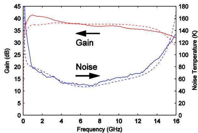
Fig. 4.6: Measured (solid) and simulated (dashed) gain and noise temperature of 0.5-13 GHz LNA module at 300 K.
