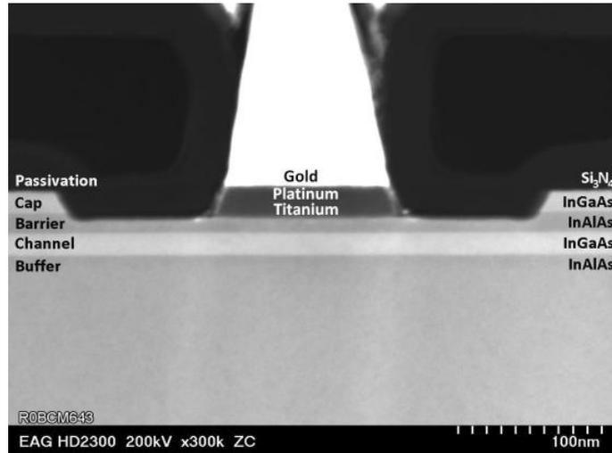
Fig. 2.1: Cross sectional STEM image of gate region in a 130 nm InP HEMT.
