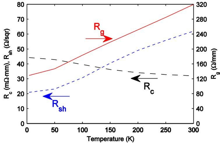
Fig. 2.6: Temperature dependence of  $R_g$ ,  $R_{sh}$  and  $R_c$ .
