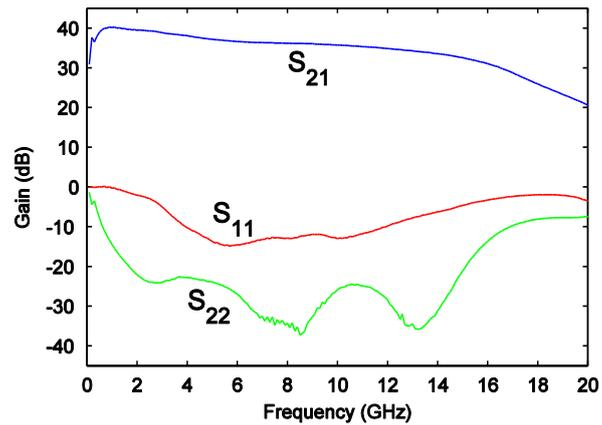
Fig. 4.5: Measured S-parameters of a 0.5-13 GHz LNA module at 300 K
