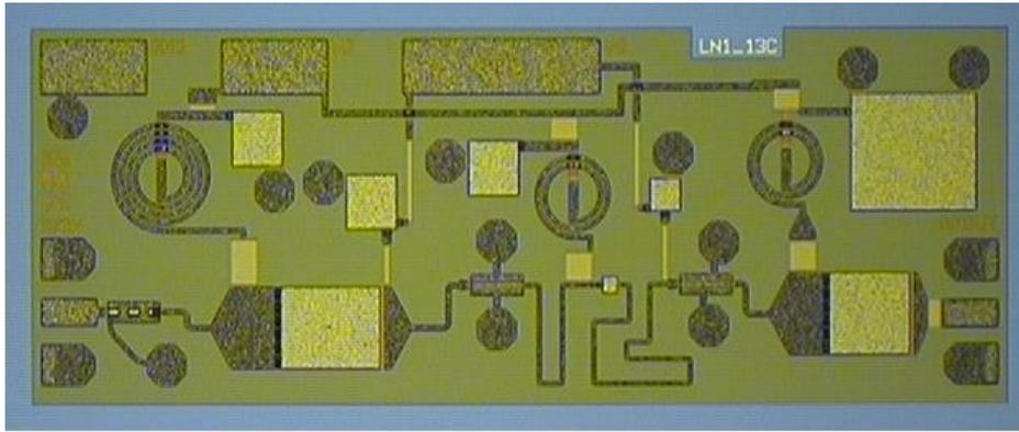
Fig. 4.3: Photograph of fabricated 3-stage 0.5-13 GHz MMIC LNA.
