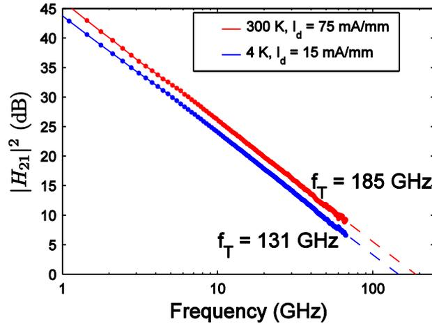
Fig. 3.14: Intrinsic current gain  $|H_{21}|^2$  at optimum low noise bias of  $V_d = 0.6$  V and  $I_d = 15$  mA/mm at 4 K and 75 mA/mm at 300 K
