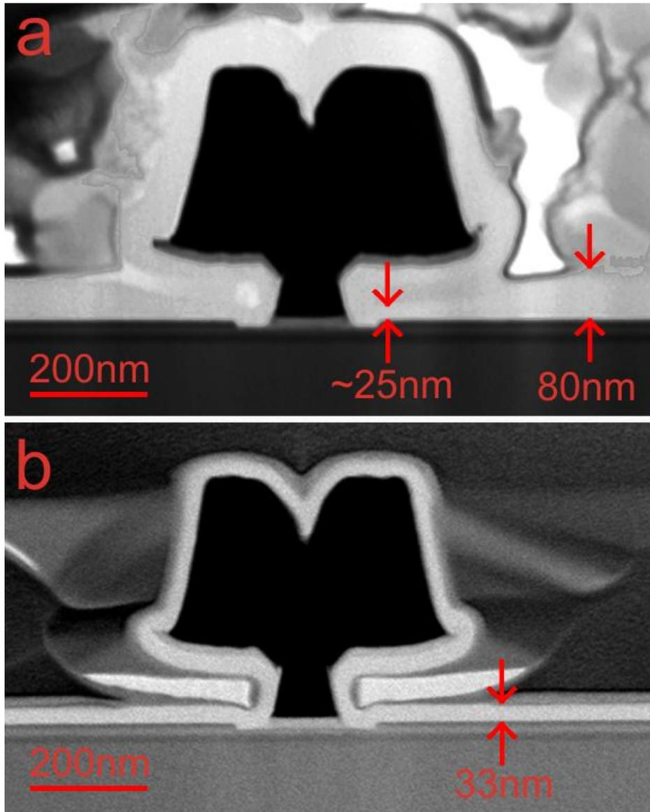
Fig. 2.2: TEM image of the gate region of a) Si<sub>3</sub>N<sub>4</sub> PECVD and b) Al<sub>2</sub>O<sub>3</sub> ALD passivated InP HEMT. The thickness of the passivation is marked in the figures.
