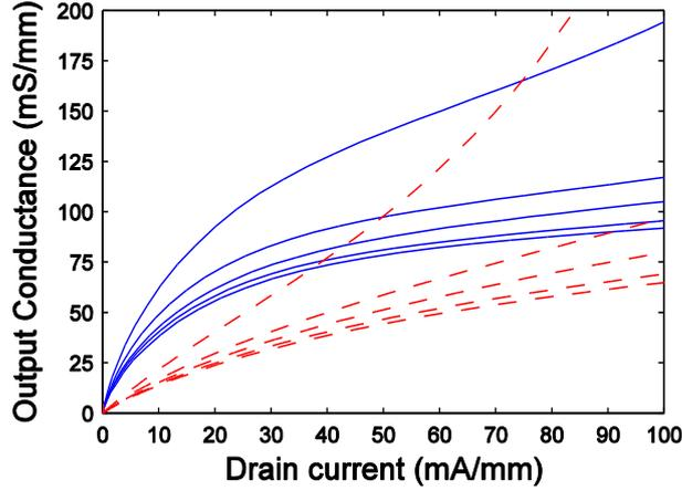
Fig. 3.9: Intrinsic  $G_{ds}$  of a  $2 \times 100 \mu\text{m}$  gate width and 130-nm gate length InP HEMT at 300 K (red dashed) and 4 K (blue solid) ambient temperature.  $V_{ds}$  measured from 0.2 V (upper curve) to 1 V (lower curve) in steps of 0.2 V.
