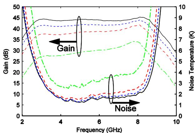
Fig. 3.15: Noise temperature and gain at 10 K of a 3-stage hybrid 4–8 GHz LNA. The 3-stage amplifier was biased at  $V_{DD} = 0.1$  V,  $I_{DD} = 3.3$  mA (green dash-dot);  $V_{DD} = 0.2$  V,  $I_{DD} = 6$  mA (red long dash);  $V_{DD} = 0.3$  V,  $I_{DD} = 8$  mA (blue short dash) and optimum bias  $V_{DD} = 0.45$  V,  $I_{DD} = 9.3$  mA (black solid).
