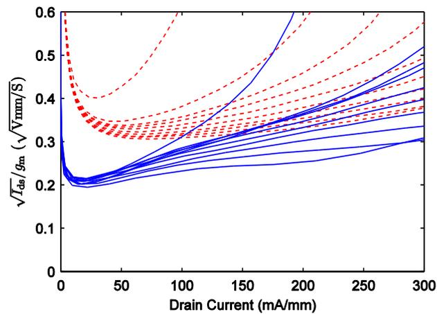
Fig. 3.4:  $\sqrt{I_{\text{ds}}}/g_m$  versus  $I_d$  of a  $2 \times 10 \mu\text{m}$  gate width and 130-nm gate length InP HEMT at 300 K (red dashed) and 4 K (blue solid) ambient temperature.  $V_{\text{ds}}$  measured from  $0.1 \text{ V}$  (upper curve) to  $1 \text{ V}$  (lower curve) in steps of  $0.1 \text{ V}$ .
