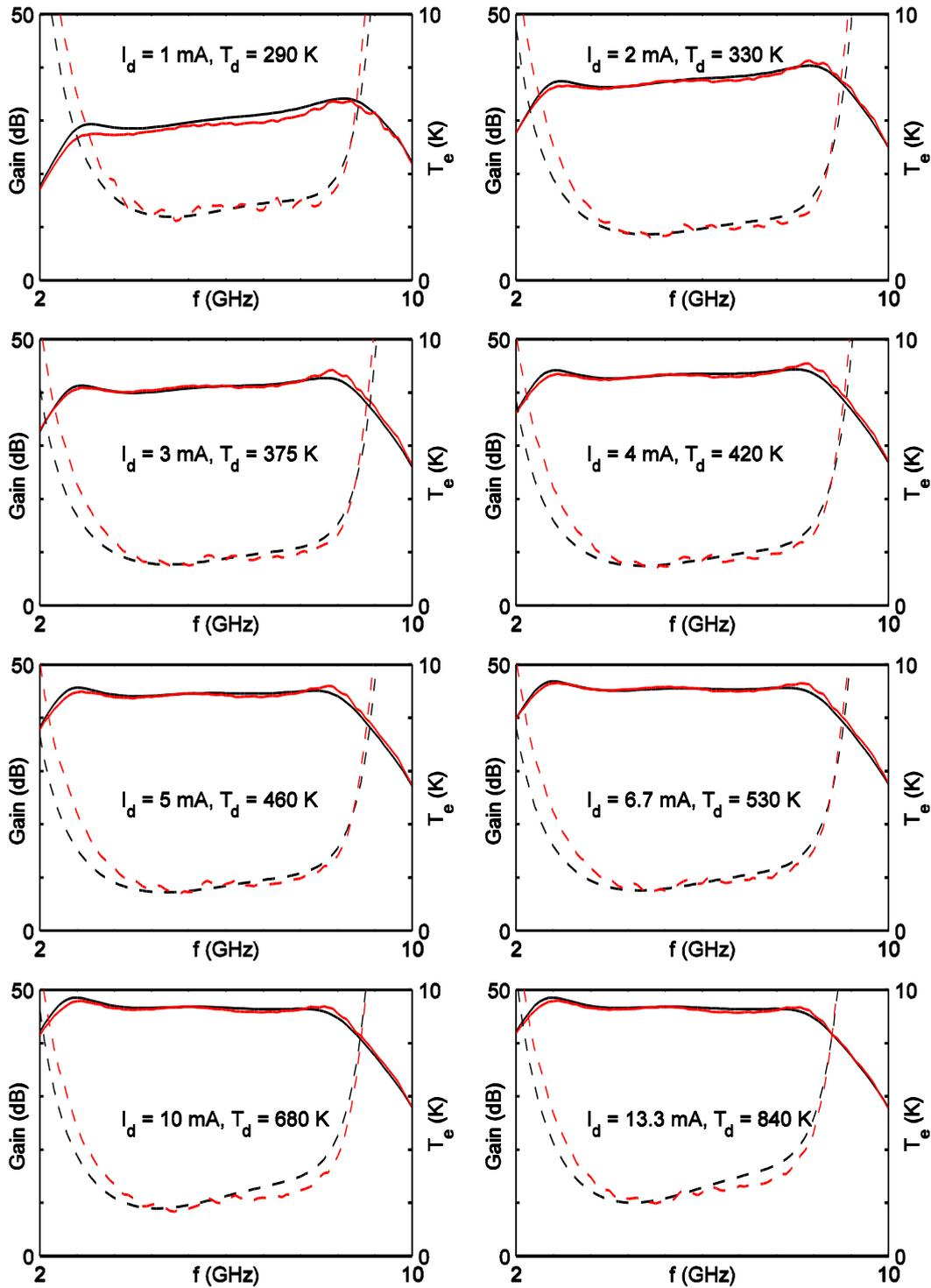
Fig. 3.11: Measured (red) and simulated (black) noise temperature (dashed) and gain (solid) at 10 K of a 3-stage hybrid 4–8 GHz LNA with  $2 \times 100 \mu\text{m}$  InP HEMTs. The 3-stage amplifier was biased so that  $V_{ds}$  over the InP HEMTs was 0.6 V in all graphs.  $I_d$ , denoting the drain current of one InP HEMT, was stepped between 1 mA (top left) and 13.3 mA (bottom right).
