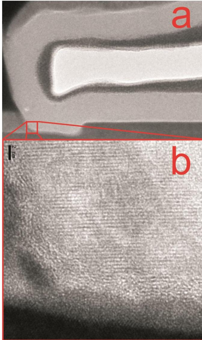
Fig. 2.5: a) TEM image of ALD passivated gate region. b) High resolution TEM image showing atomic layered structure along the film growth direction. The black bar is 2 nm long.
