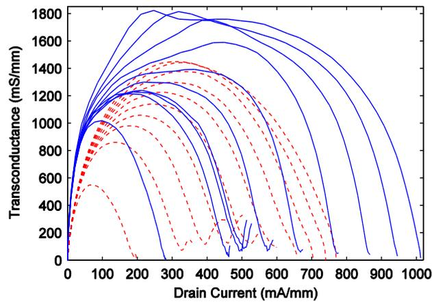
Fig. 3.3: Extrinsic  $g_m$  versus  $I_d$  of a  $2 \times 10 \mu\text{m}$  gate width and 130-nm gate length InP HEMT at 300 K (red dashed) and 4 K (blue solid) ambient temperature.  $V_{\text{ds}}$  measured from  $0.1 \text{ V}$  to  $1 \text{ V}$  in steps of  $0.1 \text{ V}$ .
