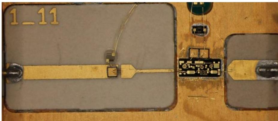
Fig. 4.4: Photograph of 3-stage MMIC mounted in housing together with the input matching network.
