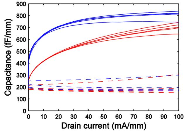
Fig. 3.8:  $C_{gs}$  (solid) and  $C_{gd}$  (dashed) of a  $2 \times 100 \mu\text{m}$  gate width and 130-nm gate length InP HEMT at 300 K (red) and 4 K (blue) ambient temperature.  $V_{ds}$  measured from 0.2 V (upper curve) to 1 V (lower curve) in steps of 0.2 V.
