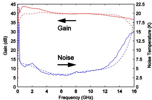
Fig. 4.7: Measured (solid) and simulated (dashed) gain and noise temperature of 0.5-13 GHz LNA module at 15 K.
