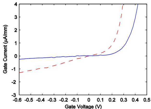
Fig. 3.5: Gate current of a  $2 \times 10 \mu\text{m}$  gate width and 130-nm gate length InP HEMT at 300 K (red dashed) and 4 K (blue solid) ambient temperature.  $V_{ds} = 0 \text{ V}$ .
