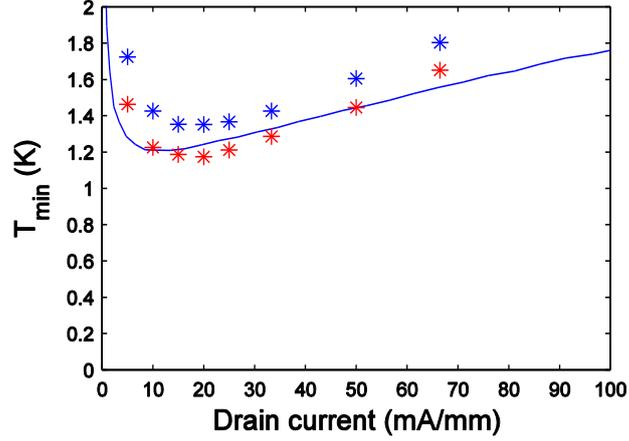
Fig. 3.13: Extracted  $T_{\min}$  with (blue dots) and without (red dots) consideration of the gate current. The noise model suggested in [20] and based on extracted  $f_T$ ,  $R_t$ ,  $G_{ds}$  and  $T_d$  is shown by the blue curve.
