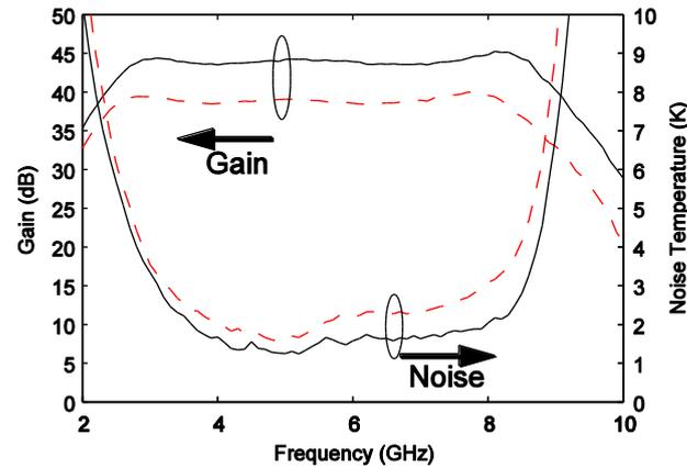
Fig. 3.17: Comparison of gain and noise temperature between 4x50  $\mu\text{m}$  InP HEMTs in this study (black curves) and previous state-of-the-art CRYO3 InP HEMTs [2] (red curves) measured at ambient temperature of 10 K in the same LNA in the same measurement system. The amplifier was in both cases biased at optimum low noise bias. Bias with Chalmers InP HEMTs was  $V_d=0.45\text{V}$  and  $I_d=9.3\text{mA}$ . Bias with CRYO3 InP HEMTs was  $V_d=0.6\text{V}$  and  $I_d=10\text{mA}$ .
