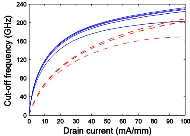
Fig. 3.10: Intrinsic  $f_T$  at 300 K (red dashed) and 4 K (blue solid) at low  $I_d$ .  $V_d$  stepped between 0.2 V (lower curve) and 1 V (upper curve) in steps of 0.2 V.
