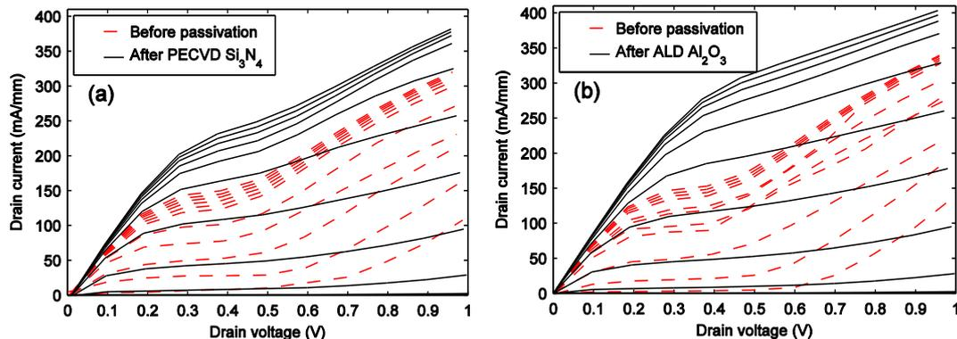
Fig. 2.3: I-V characteristics of  $2 \times 50 \mu\text{m}$  InP HEMTs before and after passivation with (a) PECVD  $\text{Si}_3\text{N}_4$  and (b) ALD  $\text{Al}_2\text{O}_3$ . Gate voltage was swept in steps of 0.1 V from -0.4 V (lower curve) to 0.6 V (upper curve).
