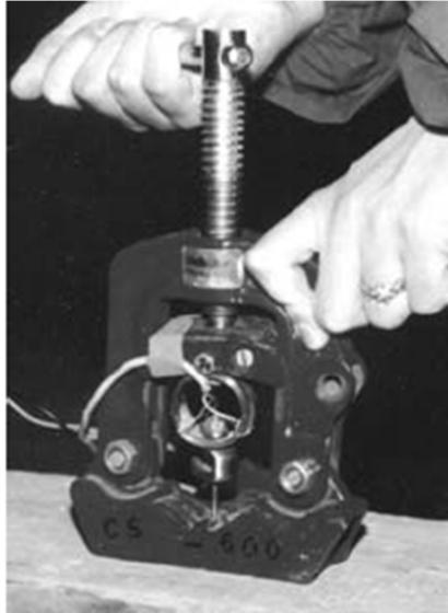
Figure 4.20 Screw withdrawal resistance test (Divós et al., 2001).
