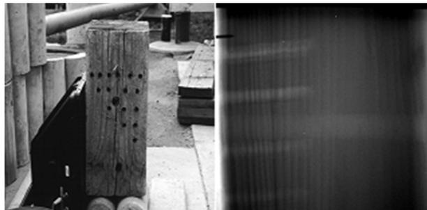
*Figure 4.11 Simulated deterioration that caused loss of cross section results in an deviation of the greyscale on the X-ray image (N.C.P.T.T., 2005).*
