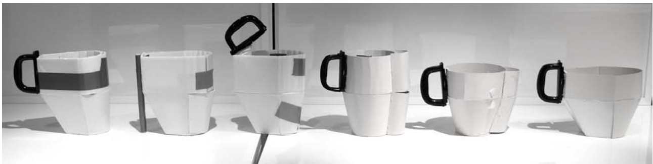
Figure 6.8 Different mock-ups to evaluate the form of the jug
