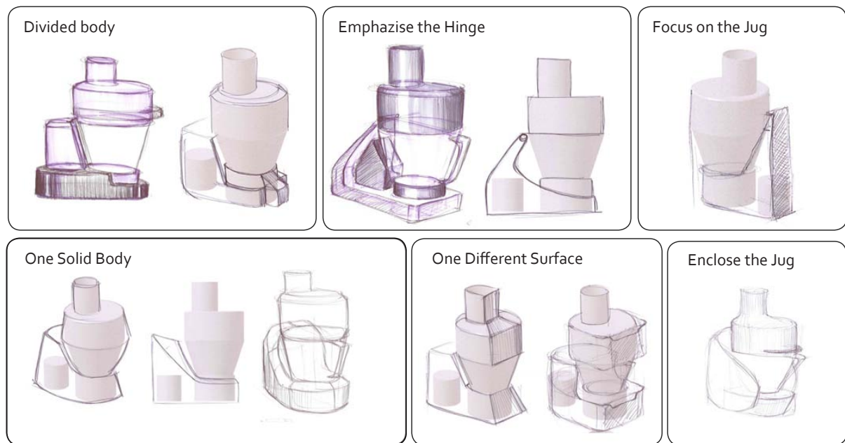
Figure 6.13 Different form tracks worked out for the BlenderJug concept
