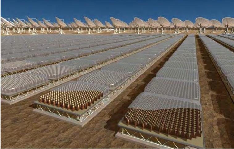
Figure 1.1: An artist's impression (Xilostudios) of the manner in which aperture array tiles in the square kilometer array can be positioned in the field and be protected by radomes [2].
