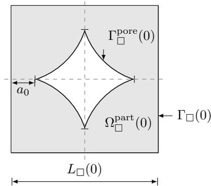
Figure 3.3: *Idealized initial configuration of the RVE in 2D consisting of circular particles in a square lattice.*
