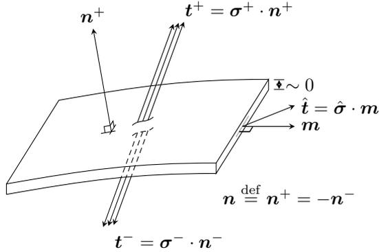
Figure 3.1: *Thin shell representing a surface with in-plane forces due to “surface tension”.*
