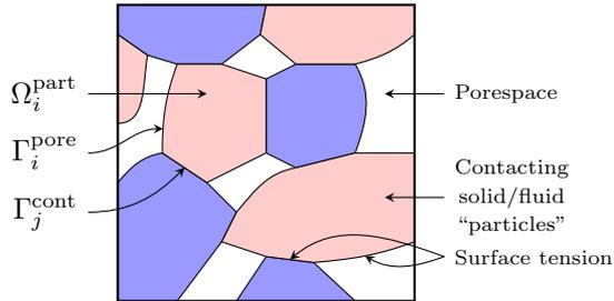
Figure 3.2: *Microstructure of porous particulate material with sintering particles in contact.*
