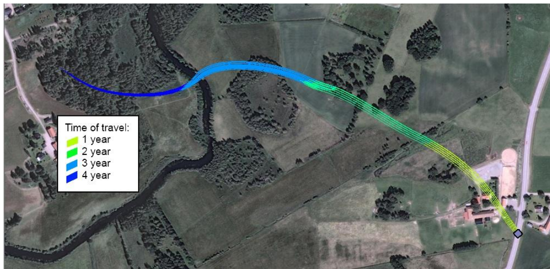
Figure 6.8 Flow path from Road 42 around Bänatorp to the production wells at Storehagen.
