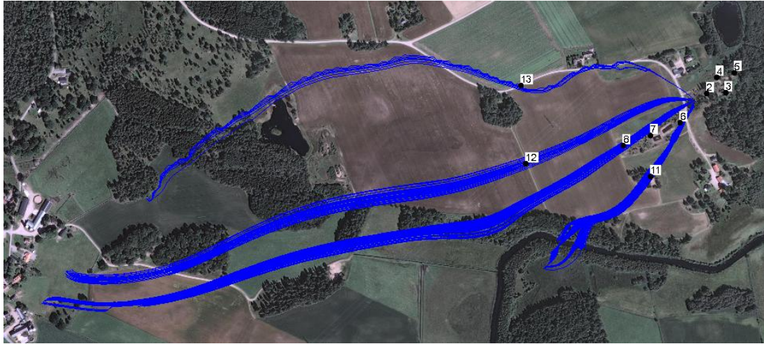
Figure 6.5 Flow patterns to production well via observation wells 13, 12, 8 and 11.
