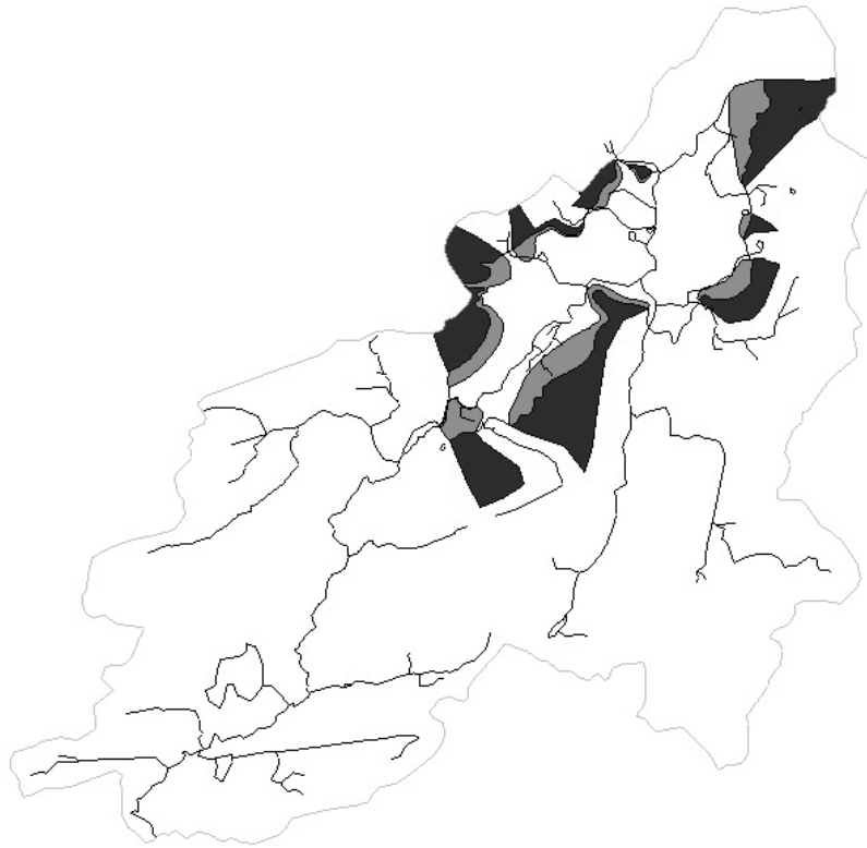
Figure 4.4 Groundwater recharge outside the modelled area. Dark grey areas represent areas that were assumed to contribute to the groundwater recharge in the model. Light grey areas were assigned a higher recharge, which corresponds to the size of the adjoining dark grey area.
