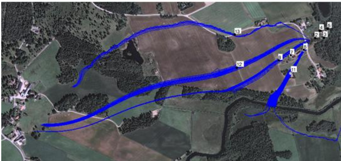
Figure 6.7 Changed flow patterns with a higher recharge rate. Recharge rate was set to the upper confidence limit: 737 mm/year.
