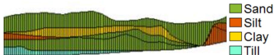
Figure 4.1 Cross section to illustrate the different thicknesses of the horizontal layers.
