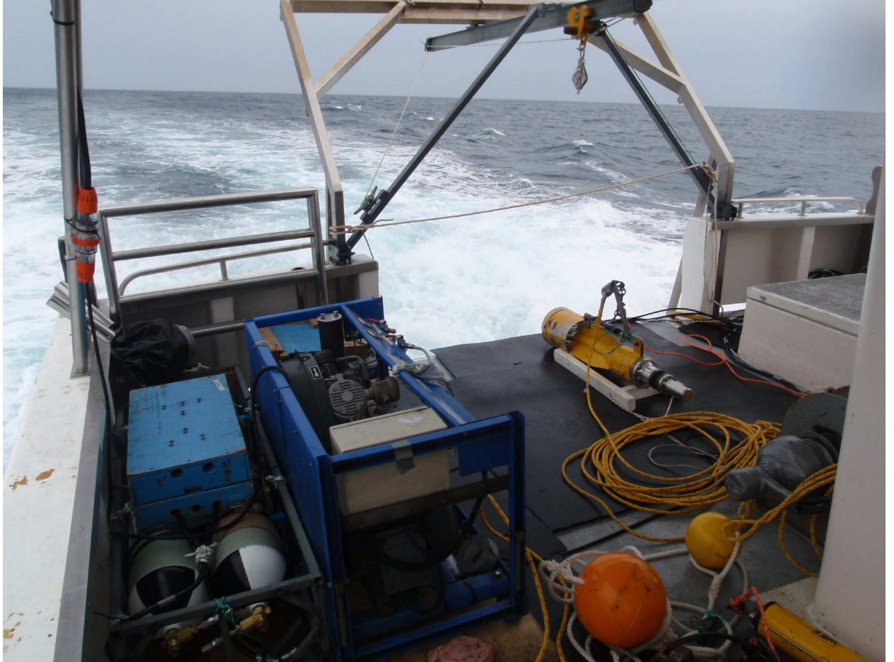
Picture during the JIP 2010 trials, on the seismic vessel. In foreground, the gas bottles and compressor and in the background, the air-gun and deployment gantry.
