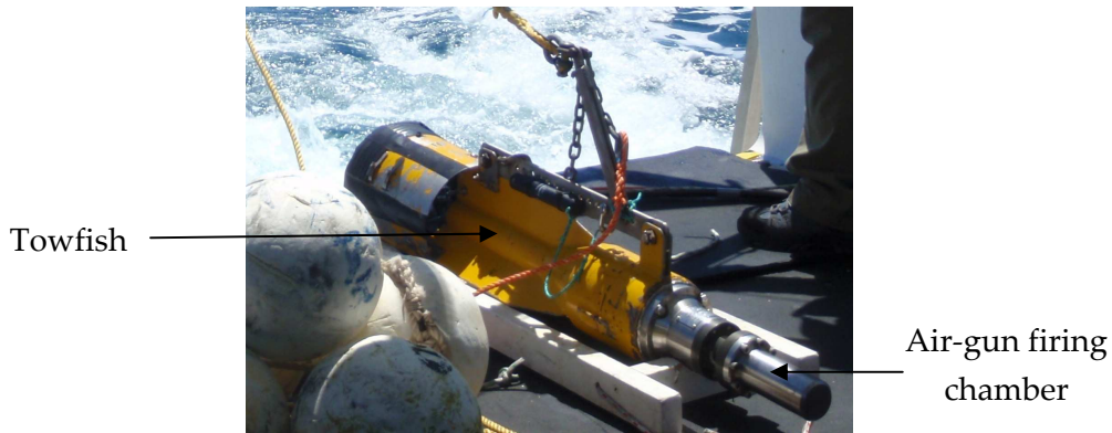
Figure 33: Bolt 600B air-gun bolted into the towfish (yellow body). All the equipment measuring data in the air-gun near-field were bolted into the towfish.
