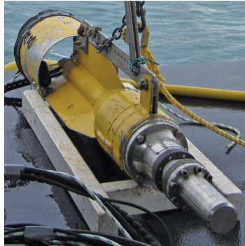
Figure 6: Bolt 600B air-gun with a 20 \text{ in}^3 firing chamber and bolted into a yellow towfish (JIP).
