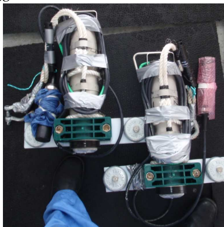
Figure 29: Two noise loggers from the JIP experiments. The body contains mainly a battery pack and electronics. The external wire is connected to the hydrophone.
