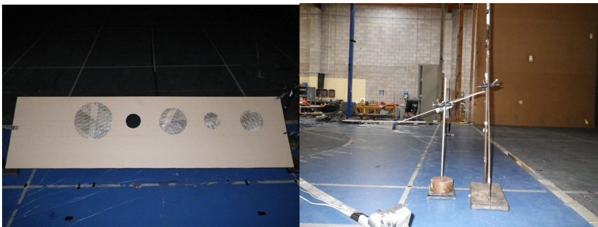
Figure 11-5: Top and side views of the testing of full-scale pressure taps
