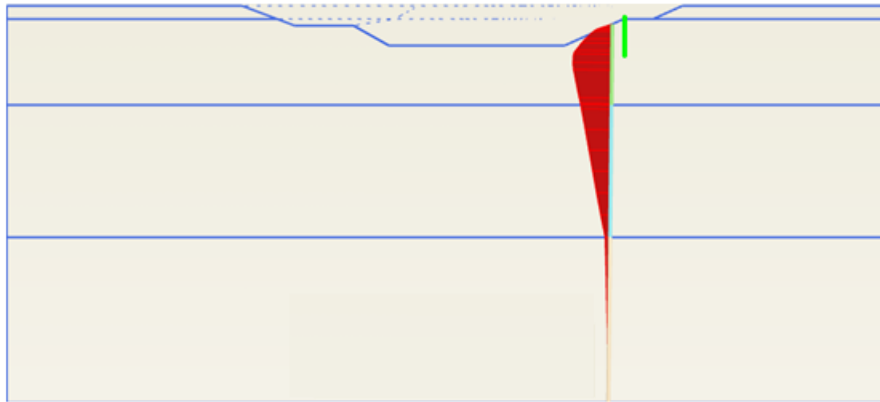
Figure 47: Horizontal displacement reading when the diaphragm wall is installed at the position of the inclinometer and the installed diaphragm wall is shown highlighted in green.
