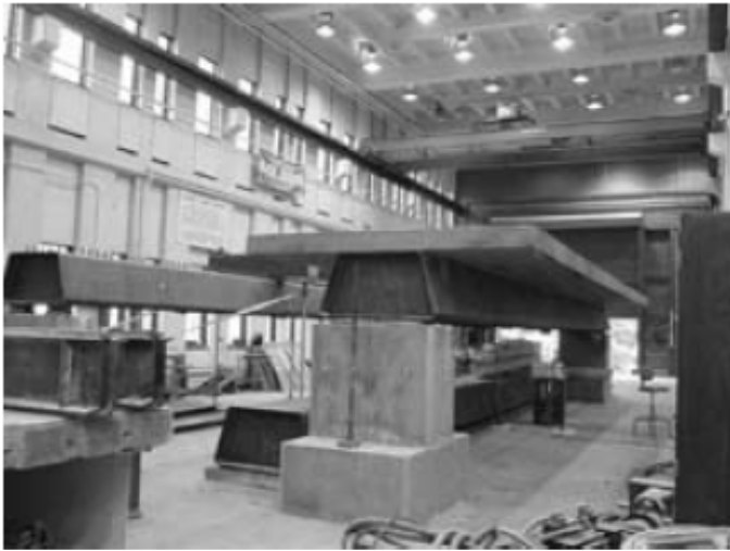
Figure 4.29 Folded plate concept, taken from Highway Bridge Services (2011)
