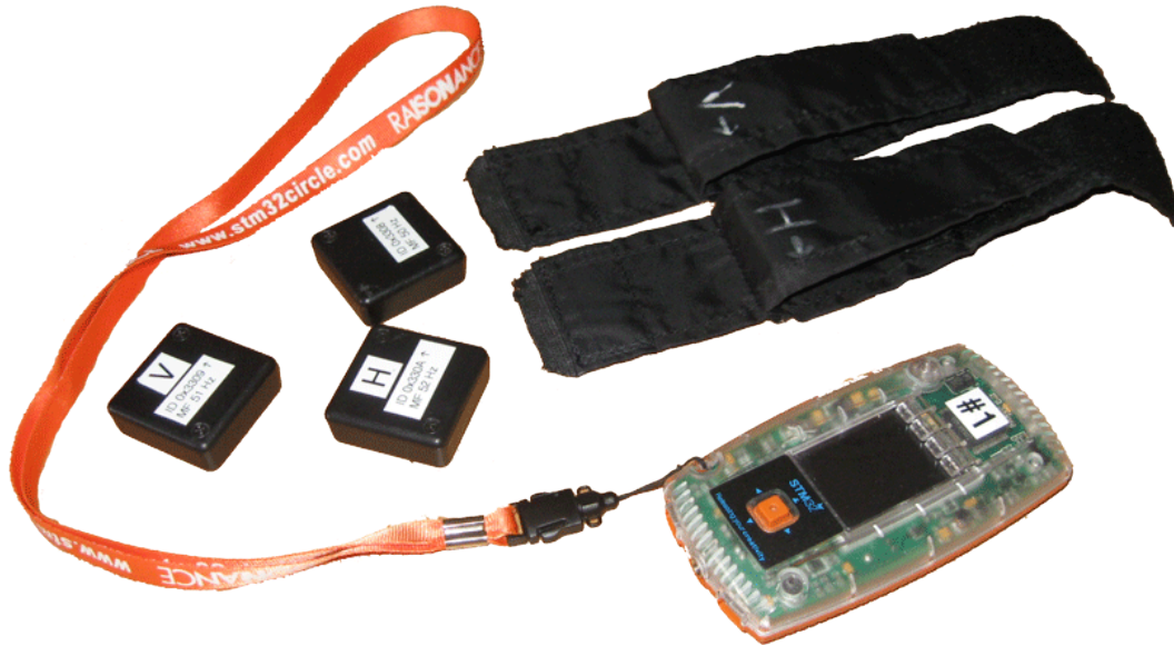
Figure 2.1: Equipment used for measuring accelerometer data of epileptic seizures. Three accelerometer sensors, wrist bands for fixation of sensors to wrists and a portable logger unit for reception and storage of accelerometer data.
